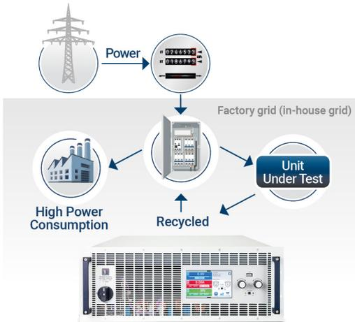
Figure 3. Energy flow with the regenerative power supply.
