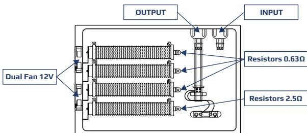
Figure 1. Image of a resistive load bank with DC fans.
