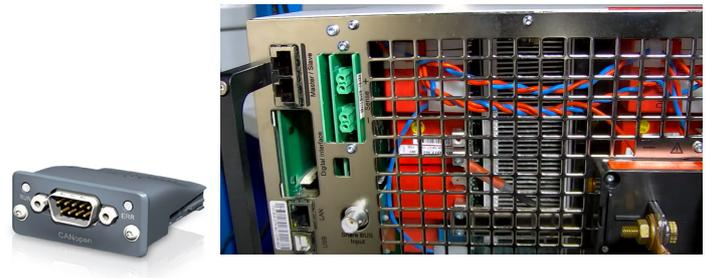
Figure 6. Anybus communication interface modules (on the left) are easily installed into an EA power supply's digital interface slot (on the right) and can be swapped based on changing test needs with a simple screwdriver.
