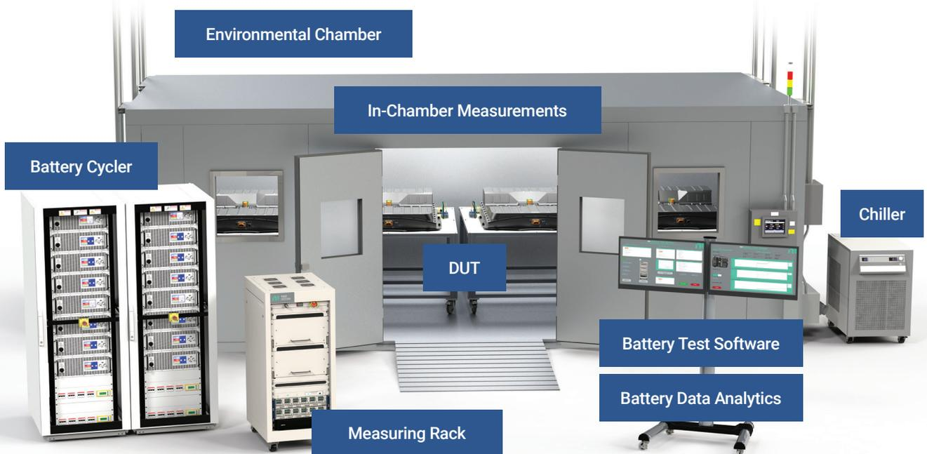
Figure 2. Typical lab setup for battery validation.
