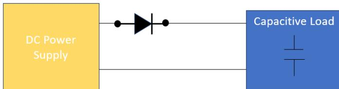
Figure 2. A series diode protects the power supply from capacitive load discharge.
