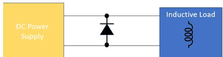
Figure 1. Use of a flyback diode to protect the power supply from back EMF.
