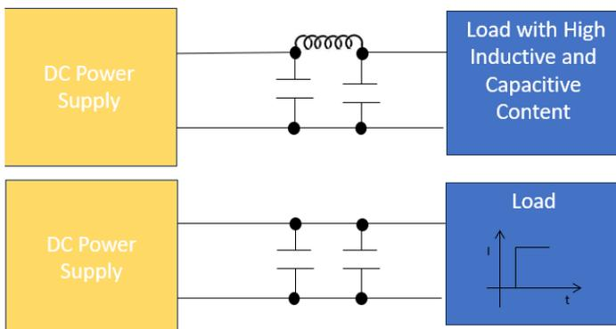
Figure 4. (Top figure) A Pi filter can isolate the power supply from high-frequency effects.
