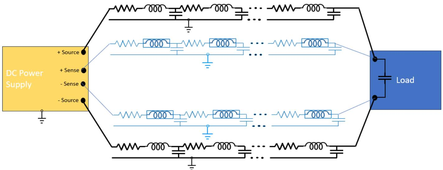
Figure 6. A power supply-load circuit with the source and sense lead wires represented as distributed R-L-C networks. Even though the power supply is delivering DC voltage, the circuit is essentially an AC network.
