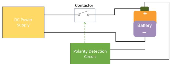
Figure 3. A polarity detection circuit controls a contactor to prevent applying power to a battery if the battery has been incorrectly connected into the circuit.
