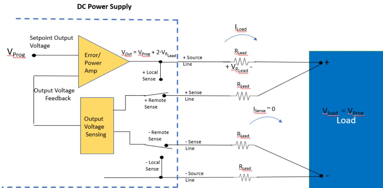
Figure 5. Remote sensing at the load enables the power supply to compensate for the voltage drop in the lead wires and ensure that the programmed voltage is applied to the load.
