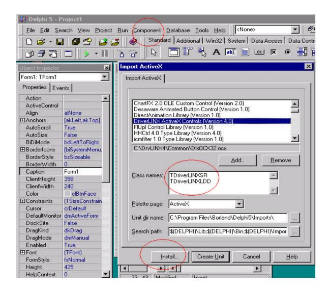
At this point Delphi or Builder will generate a "package" for the DriverLINX ActiveX controls. This unit or package defines classes for the two controls of DriverLINX:
