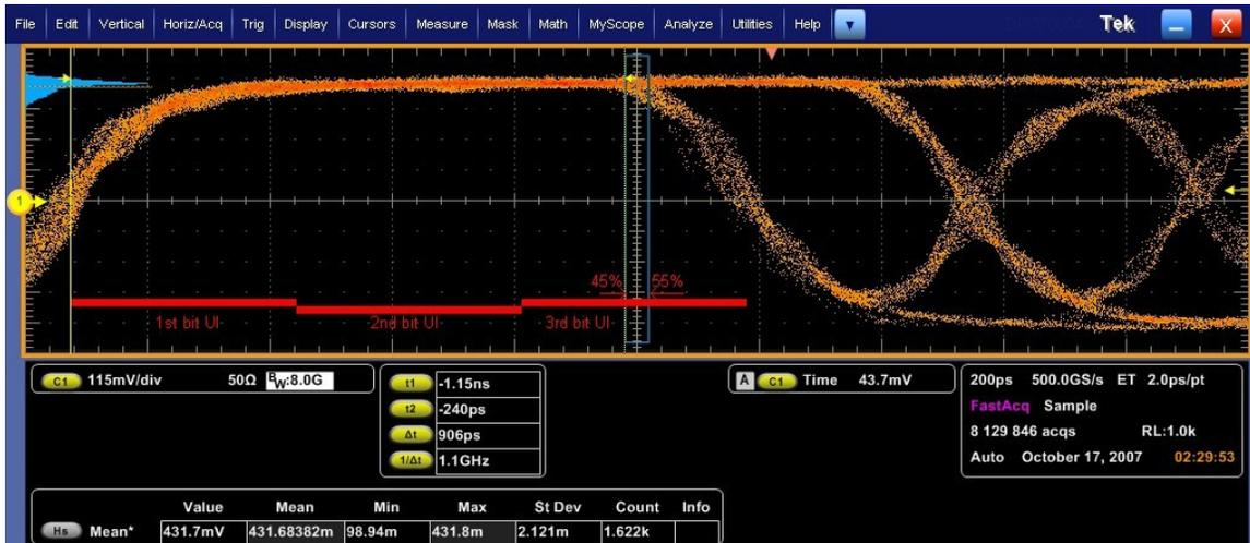
Figure: Measurement of  $V_H$  for Non-Transition bit.
