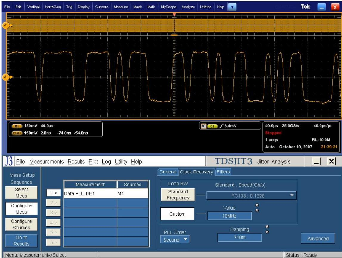
Press Go to Results button and click on “Start” to run the test. When complete, the statistics table will contain the results.
