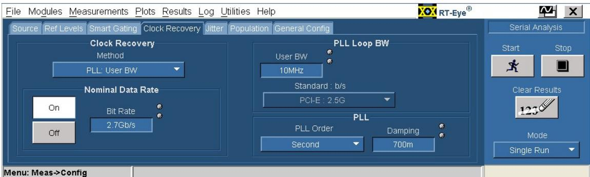
**Figure:** Configuring the clock recovery parameters for Eye Diagram measurement.
