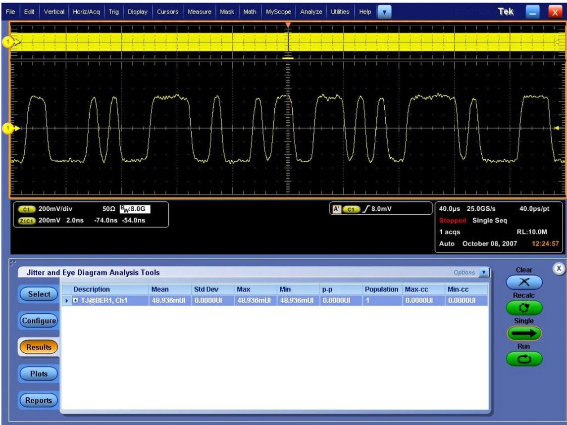
If pre-emphasis is applied the same setup as above can be used to measure Total Jitter.
