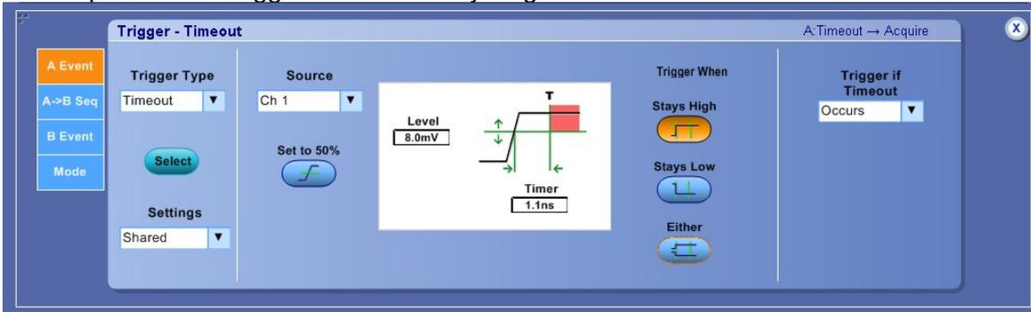
Figure: Screen showing trigger setting for measurement of  $V_H$  for transition and non-transition bit.
