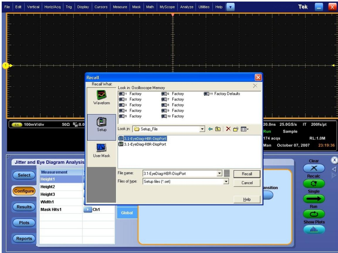
Figure: Recalling setup for Eye Diagram testing.
