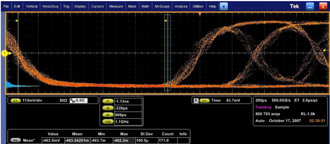
Figure: Measurement of  $V_L$  for Non-Transition bit.
