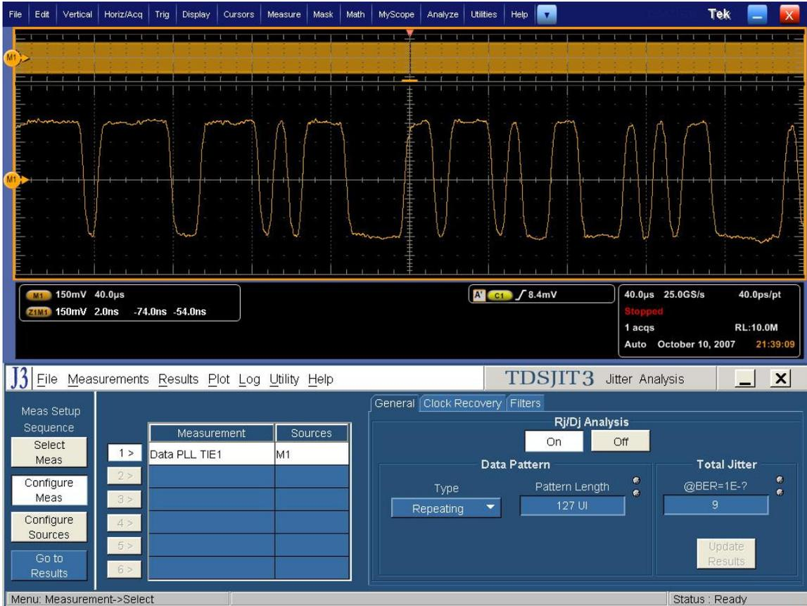
Configure Clock Recovery with 10MHz Loop BW, 2<sup>nd</sup> Order PLL, and a damping factor of 0.707.
