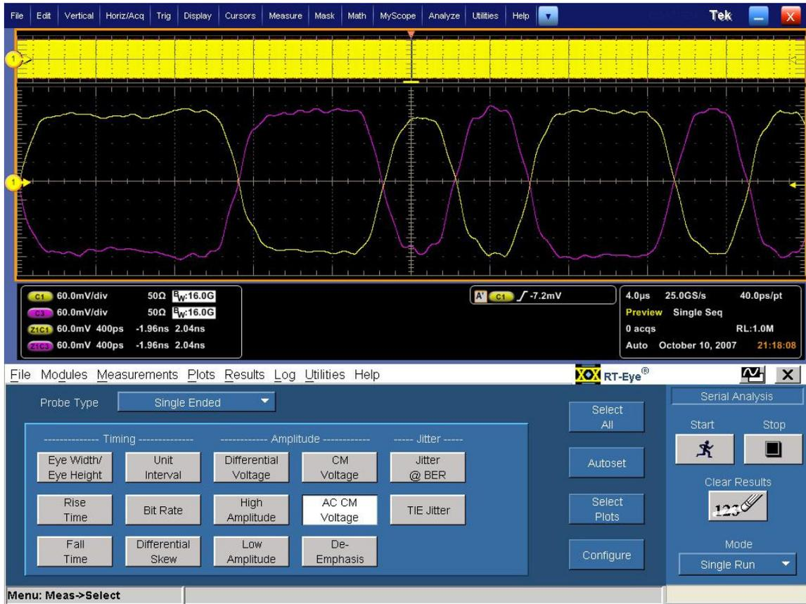
Click on “Start” to run the test. Record the StdDev Common Mode Voltage from the Results → Details section as shown below.
