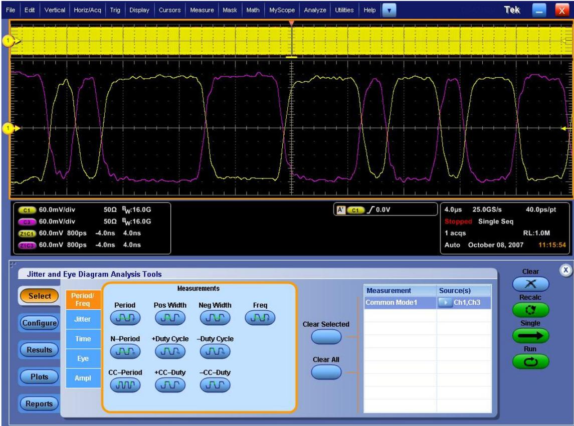
Click on “Start” to run the test. Record the Mean Common Mode voltage as shown below.
