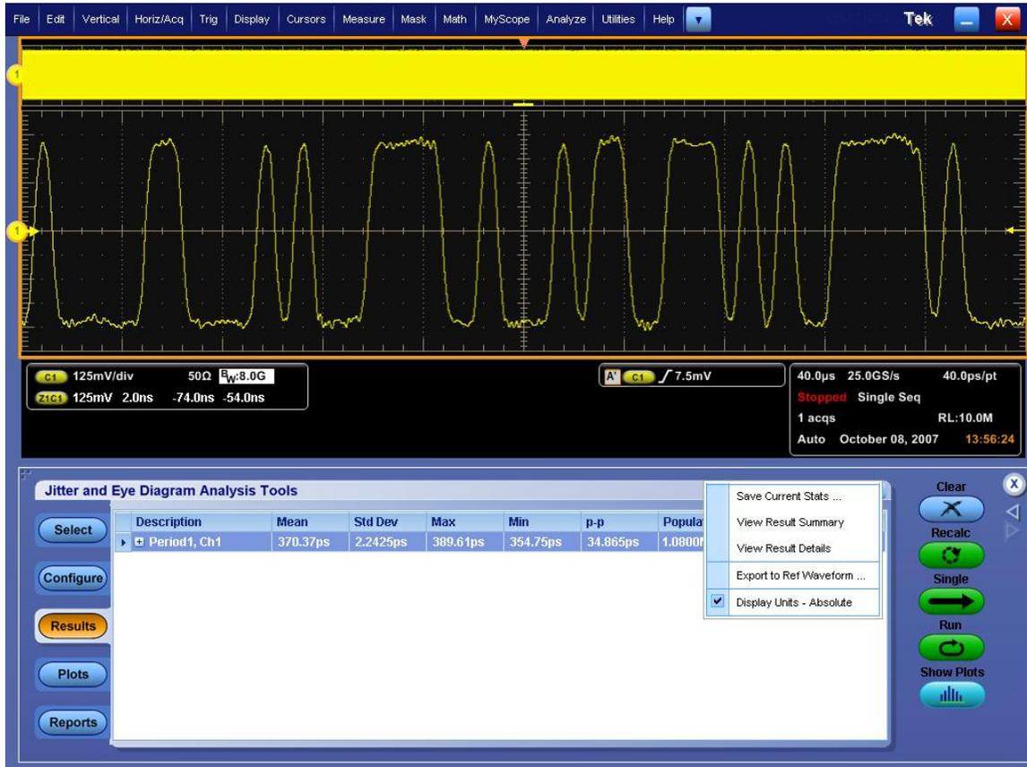
Once the reference waveform is transferred into the scope's storage, minimize the DPOJET screens, so that only the scope UI is displayed. Turn on the scope cursors, and place across 10 cycles of the profile, as shown.
