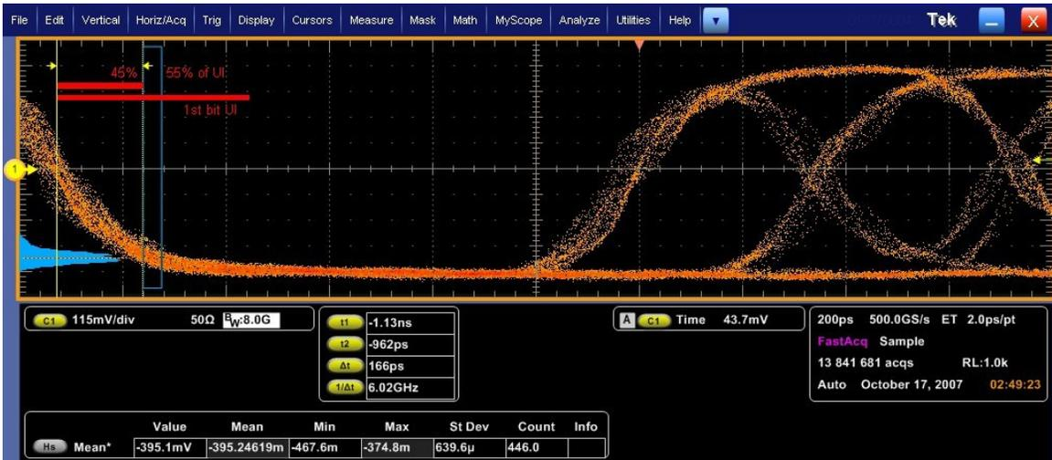
**Figure:** Measurement of  $V_L$  for Transition bit.
