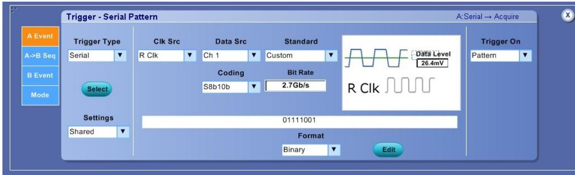
Figure: Scope trigger setting for skew measurement.
