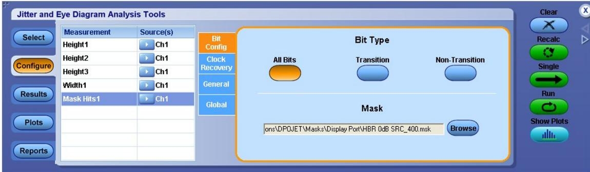
**Figure:** Eye diagram plot configuration – Setting mask file for eye diagram.
