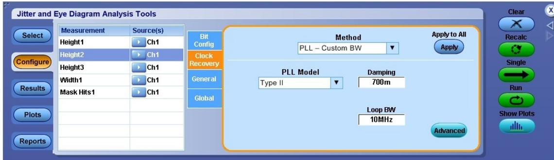
**Figure:** Measurement configuration – Setting clock recovery parameters.
