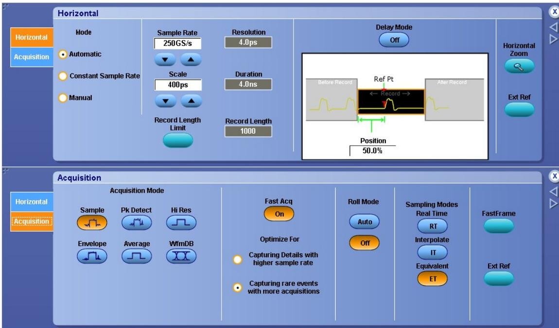
**Figure:** Scope horizontal and acquisition setting for  $V_H$  and  $V_L$  measurements.
