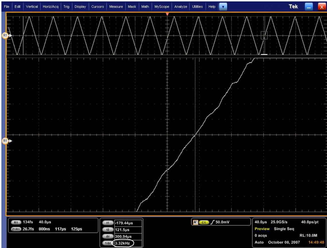
Again, it is necessary to divide the period by 10, then invert to get the modulation frequency, or alternatively multiply the 1/Δt value by 10 to get the modulation frequency.
