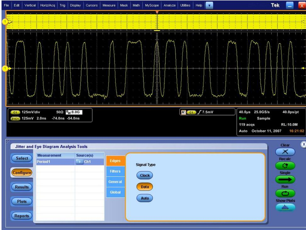
Configure filters: 2<sup>nd</sup> order low pass, 1.98MHz
