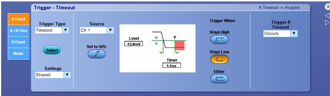
**Figure:** Scope trigger setting for  $V_H$  and  $V_L$  measurements.
