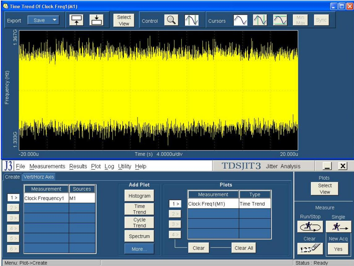
To get more measurement resolution, use the Export: Save function in JIT3's plot screen, and select "Ref" from the pull-down menu. This transfers the Period Profile into the scope's Ref waveform memory.
