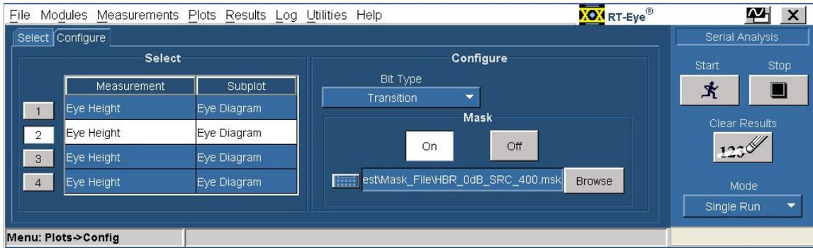
**Figure:** Configuring the plots and Eye diagram mask files for Eye Diagram measurement.
