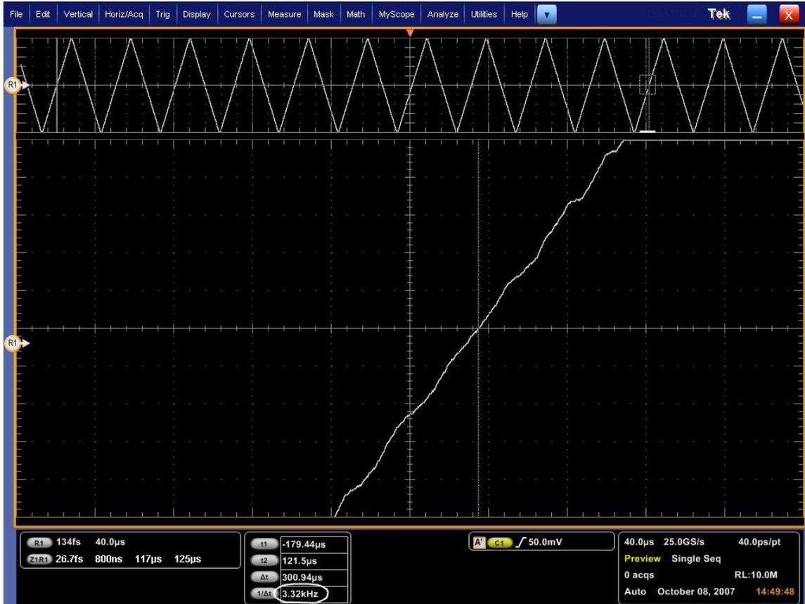
Again, it is necessary to divide the period by 10, and then invert to get the modulation frequency, or alternatively multiply the  $1/\Delta t$  value by 10 to get the modulation frequency.
