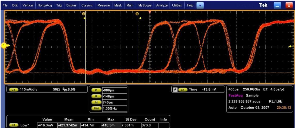
Figure: Screen showing measurement of  $V_L$  with cursor gating enabled
