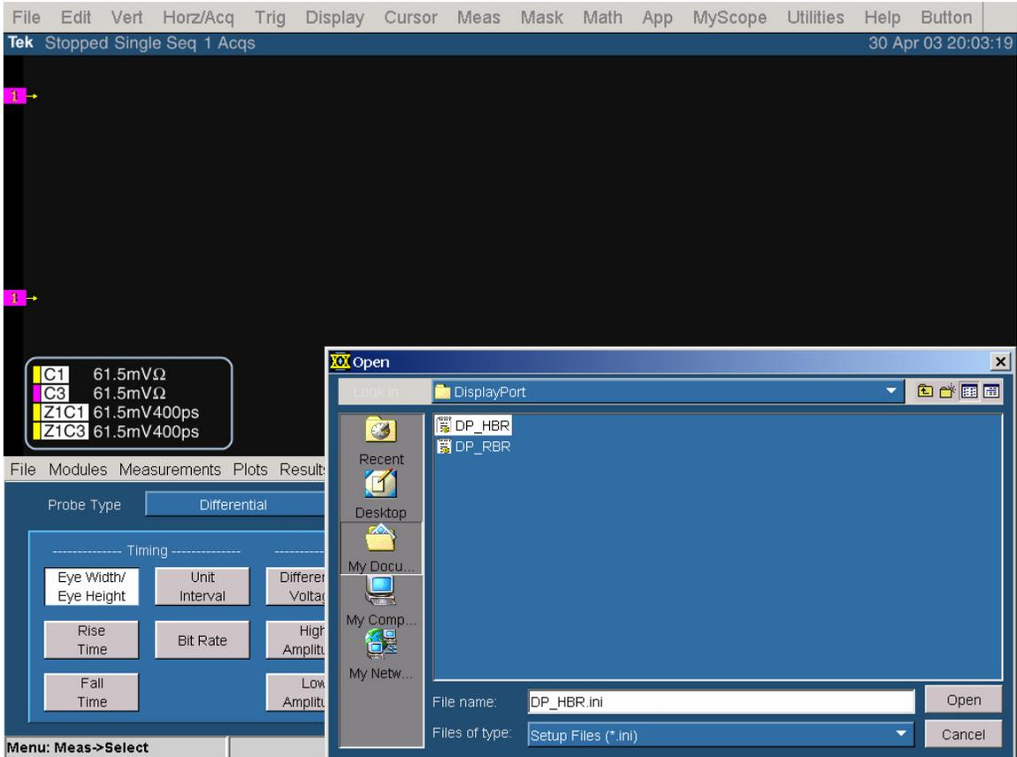
**Figure:** Recalling setup for Eye Diagram measurement on RT-Eye application.
