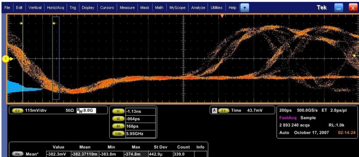
Figure: Measurement of  $V_L$  for Transition bit of signal with pre-emphasis.
