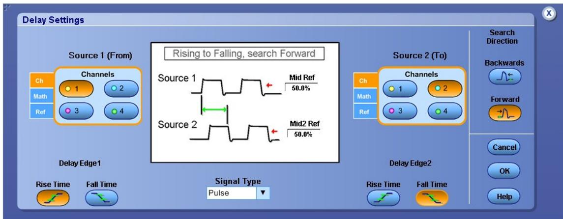
**Figure:** Delay measurement setting for intra-pair skew measurement.
