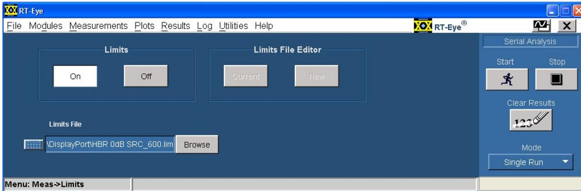
**Figure:** Configuring the limits for Eye Diagram measurement.
