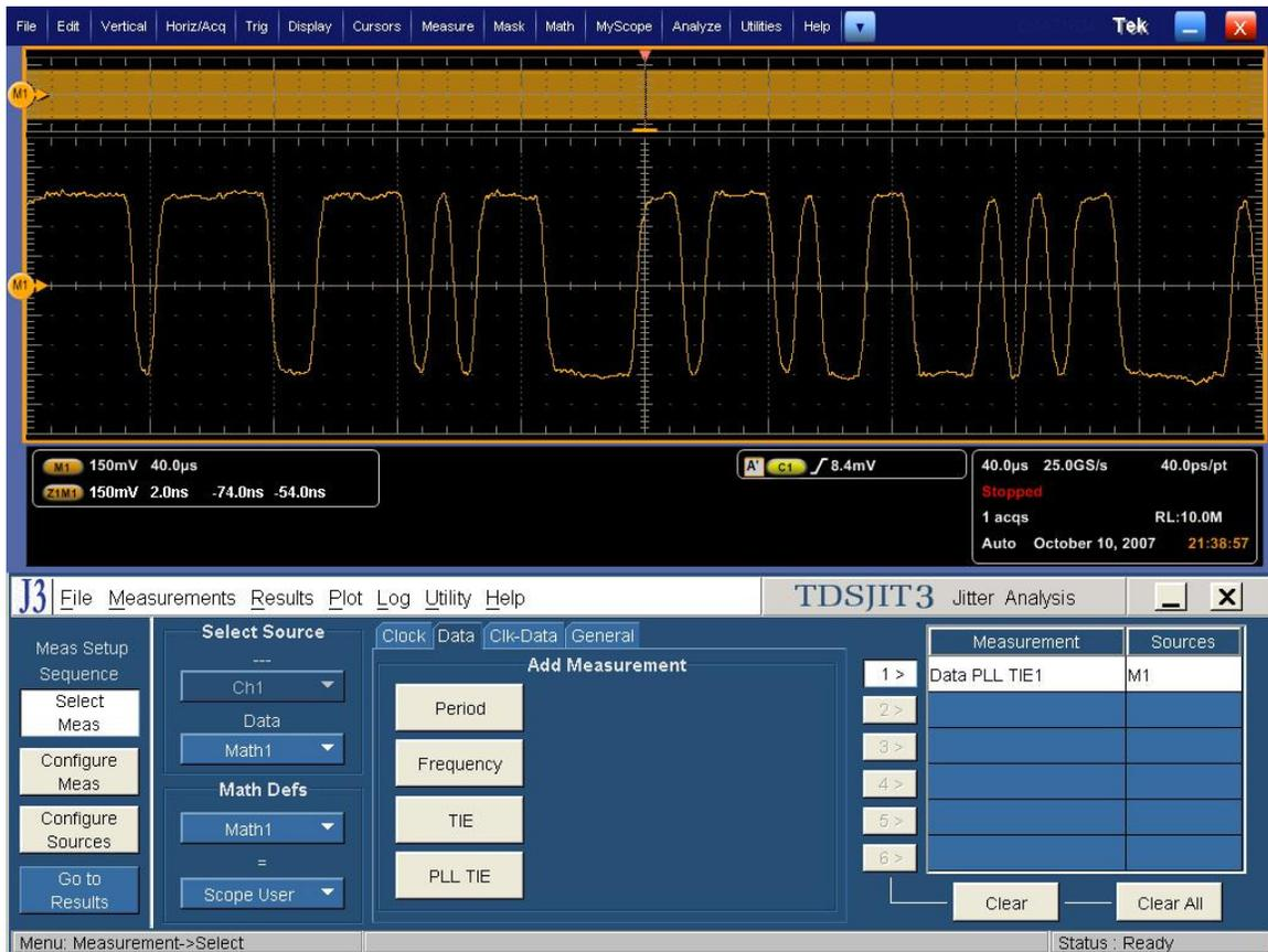
In the Configure enable RjDj analysis with a repeating pattern length of 127 and BER-9.
