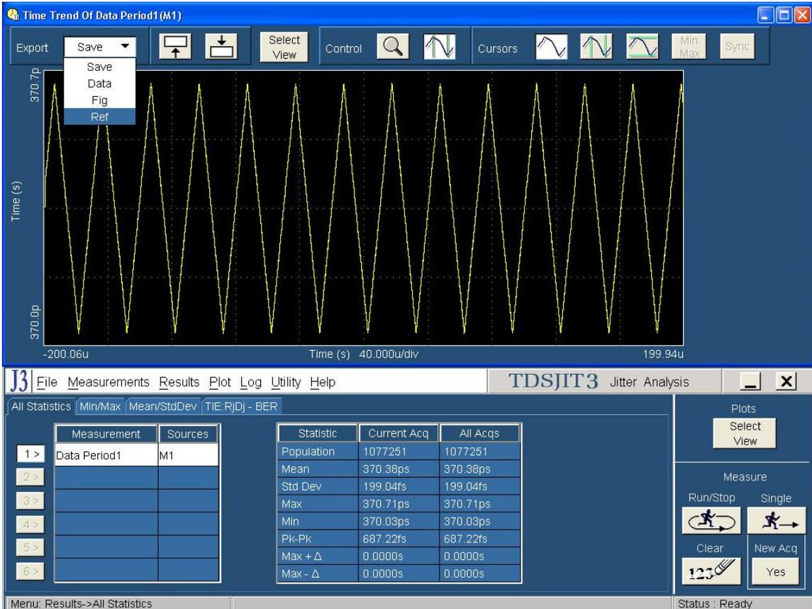
Using the same technique described in 3-14, record each of the 10 max period peak points. Average these values to determine the Measured Mean Max period.
