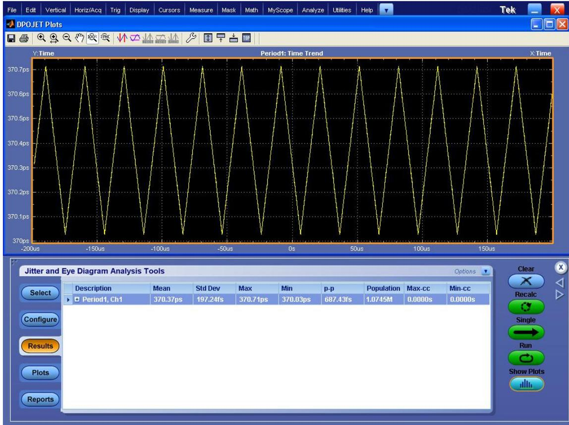
In some cases, it will be adequate to make the measurements using the cursor capability in DPOJET to measure the modulation frequency. Set cursors at the X axis crossing across 10 cycles. To arrive at the modulation frequency, take the delta time value, divide by 10, and invert to get frequency.
