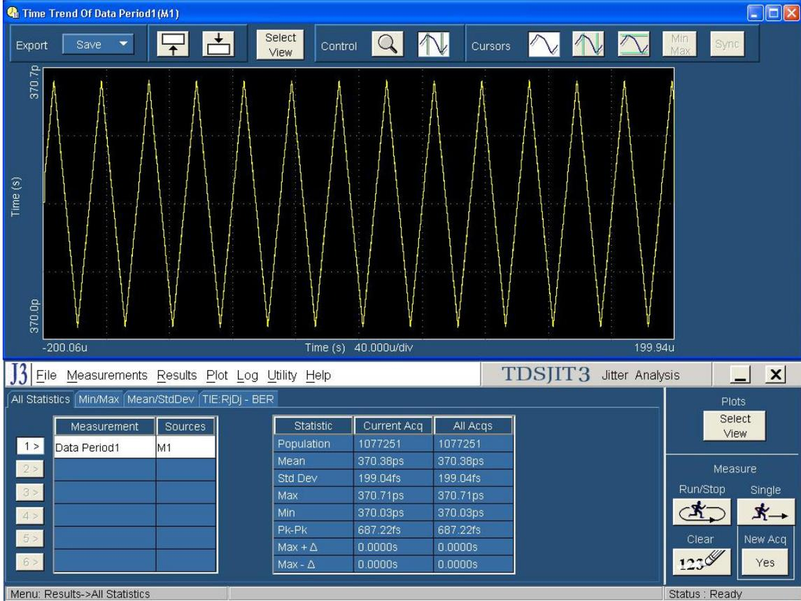
**NOTE: The TDSJIT3 software provides the ability to do cursor measurements directly on the profile plot. However, the 4 digits of resolution obtained when using JIT3 cursor measurements (1000 ppm) is not sufficient for this test.**
