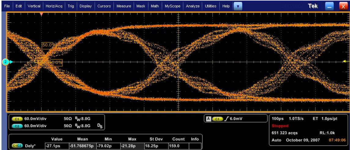
Figure: Skew measurement using scope delay measurement.
