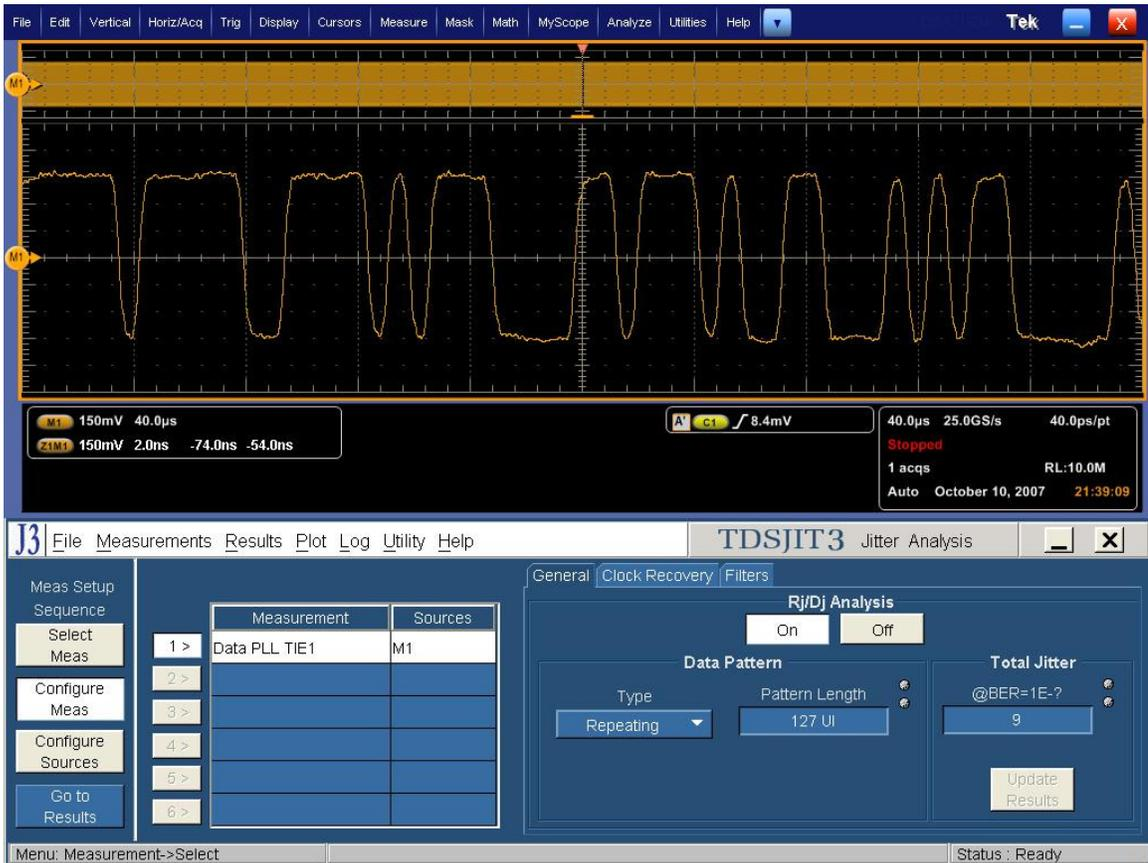
Configure Clock Recovery with 10MHz Loop BW, 2nd Order PLL, and a damping factor of 0.707
