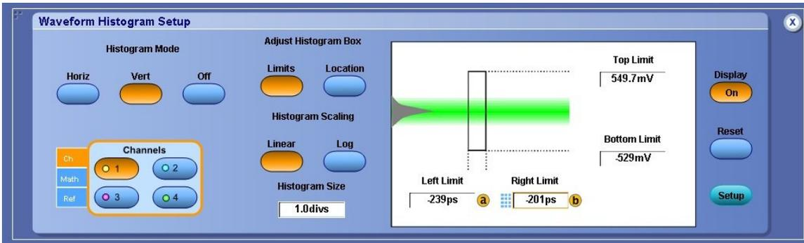
**Figure:** Waveform histogram setting to measure  $V_H$  and  $V_L$  for transition and non-transition bit.
