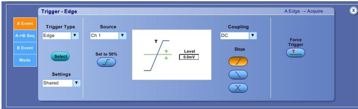
**Figure:** Trigger setting for intra-pair skew measurement.
