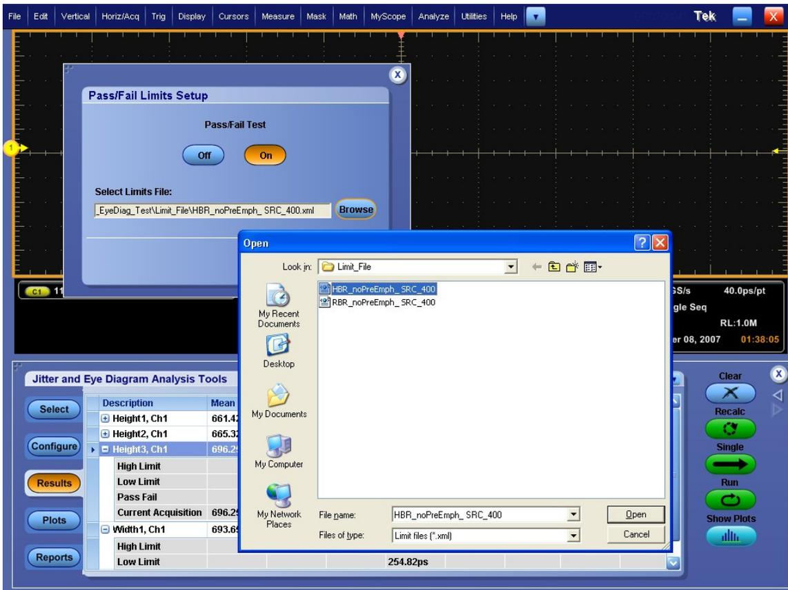
**Figure:** Pass/Fail limit setting – Navigate through Analyze > Jitter and Eye Analysis > Limits.
