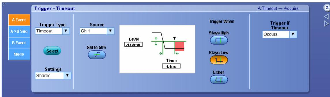
**Figure:** Scope trigger setting to measure  $V_L$  for transition and non-transition bit.
