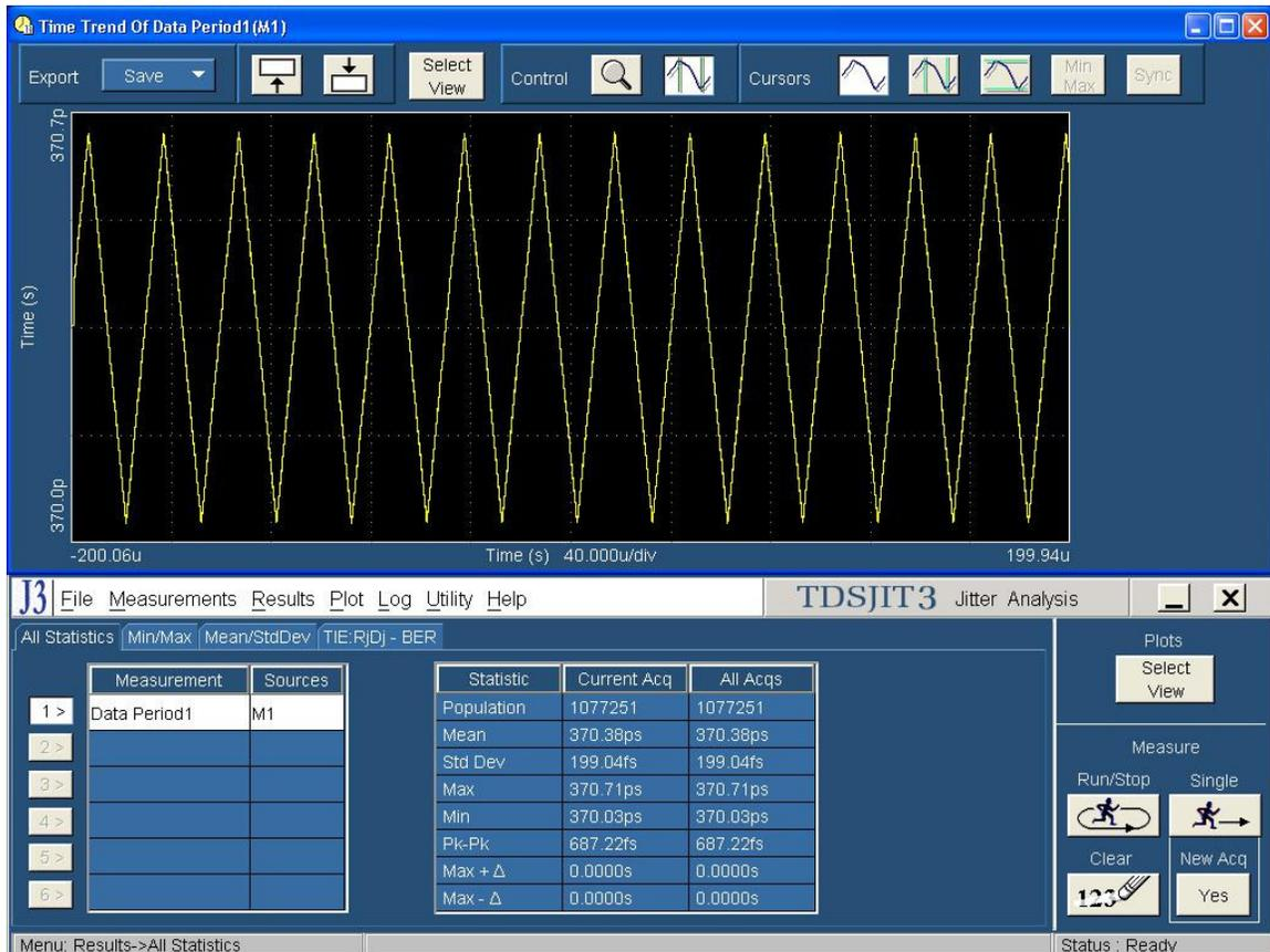
In some cases, it will be adequate to make the measurements using the cursor capability in JIT3 to measure the modulation frequency. Set cursors at the X axis crossing across 10 cycles. To arrive at the modulation frequency, take the delta time value, divide by 10, and invert to get frequency.
