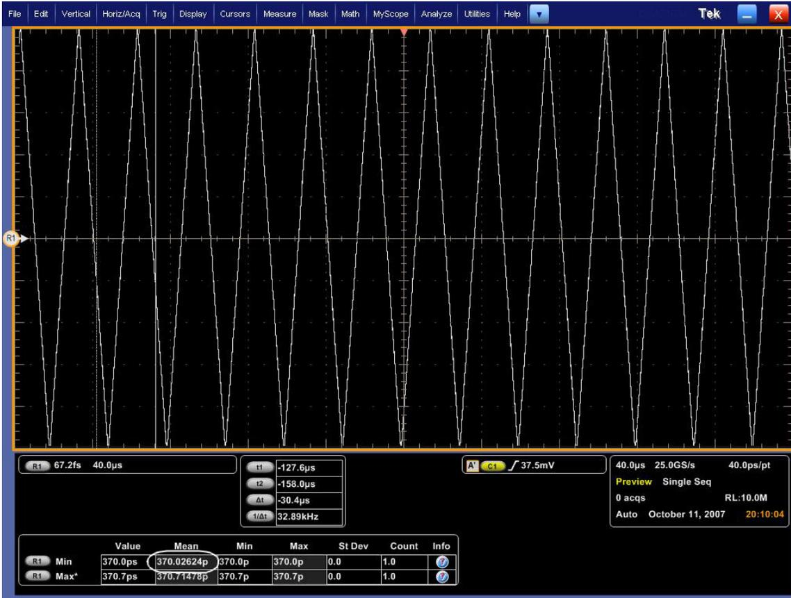
Calculate deviation = (Nominal – Measured Mean Min Period)/Nominal \* 1e6 ppm where Nominal is 370.3704 ps for HBR devices and 617.2840 ps for RBR devices.
