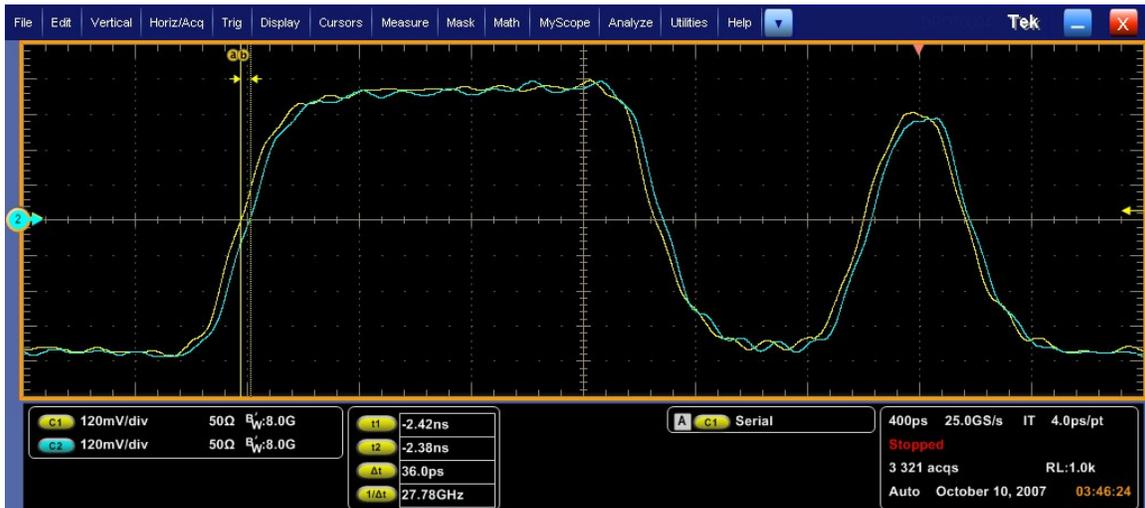
Figure: Skew measurement using cursors by triggering on specific pattern.
