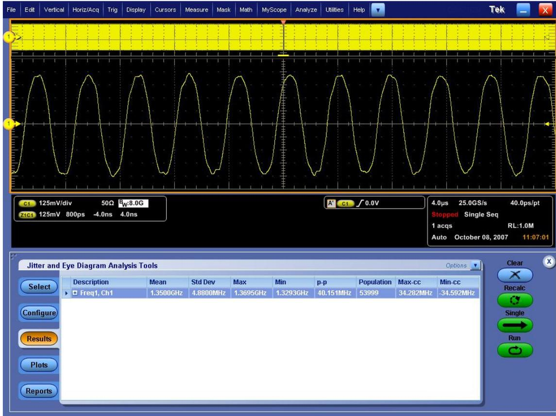
Note that this measurement is rounded up from an internal representation of 9 digits. For measurements that are near the limit, it is possible to use the following procedure to view additional resolution on the measurement.
