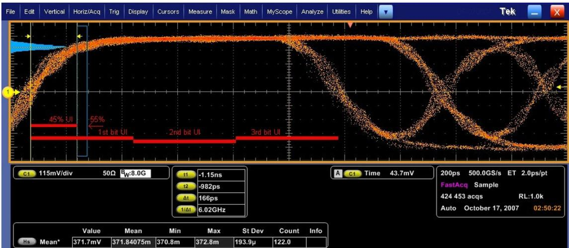
Figure: Measurement of  $V_H$  for Transition bit.
