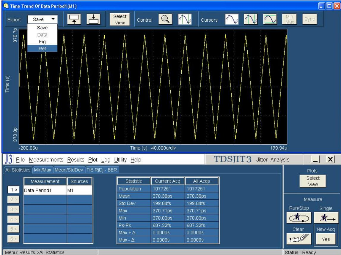
Once the reference waveform is transferred into the scope's storage, minimize the TDSJIT3 screens, so that only the scope UI is displayed.
