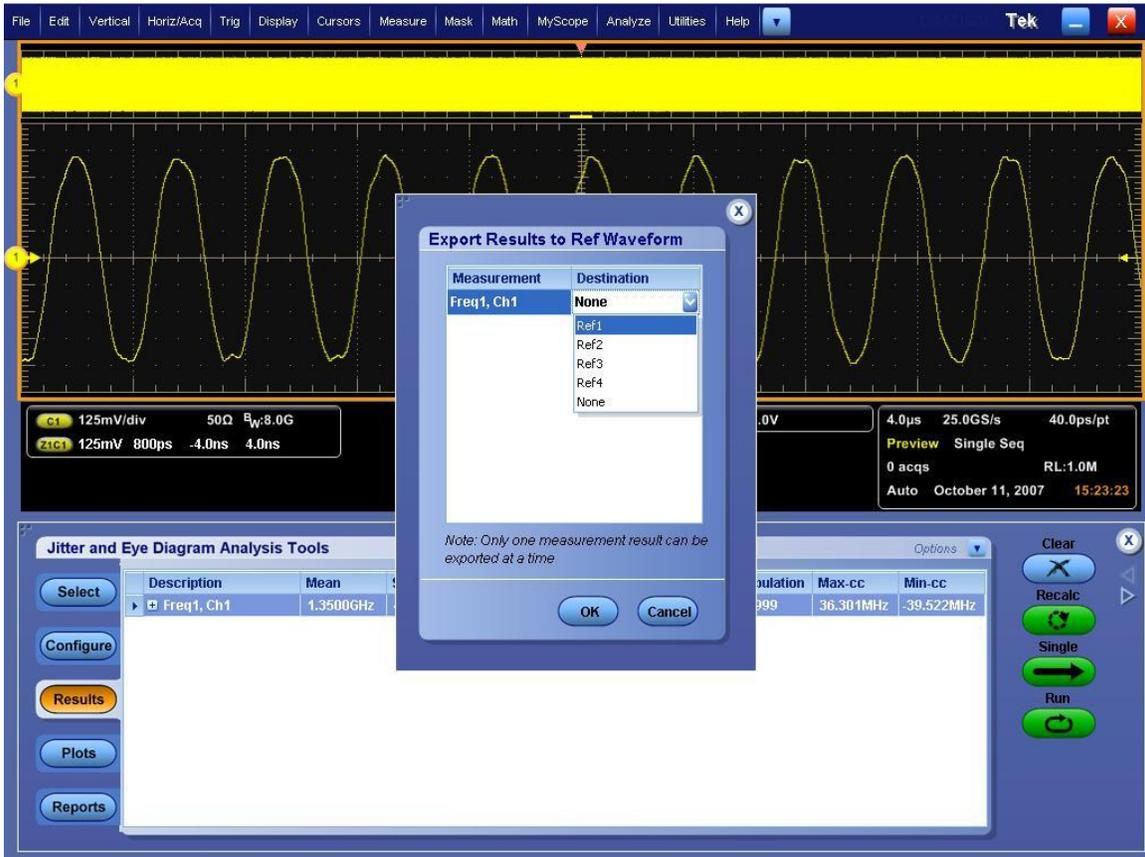
Once the reference waveform is transferred into the scope's storage, minimize the DPOJET screen so that only the scope UI is displayed.
