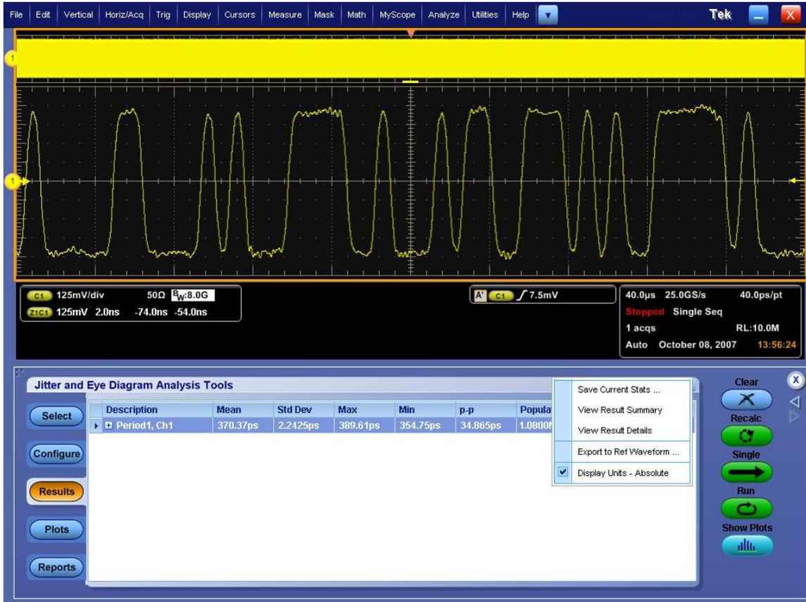
Using the same technique described in test 3-14, record each of the 10 max period peak points. Average these values to determine the Measured mean Max period.
