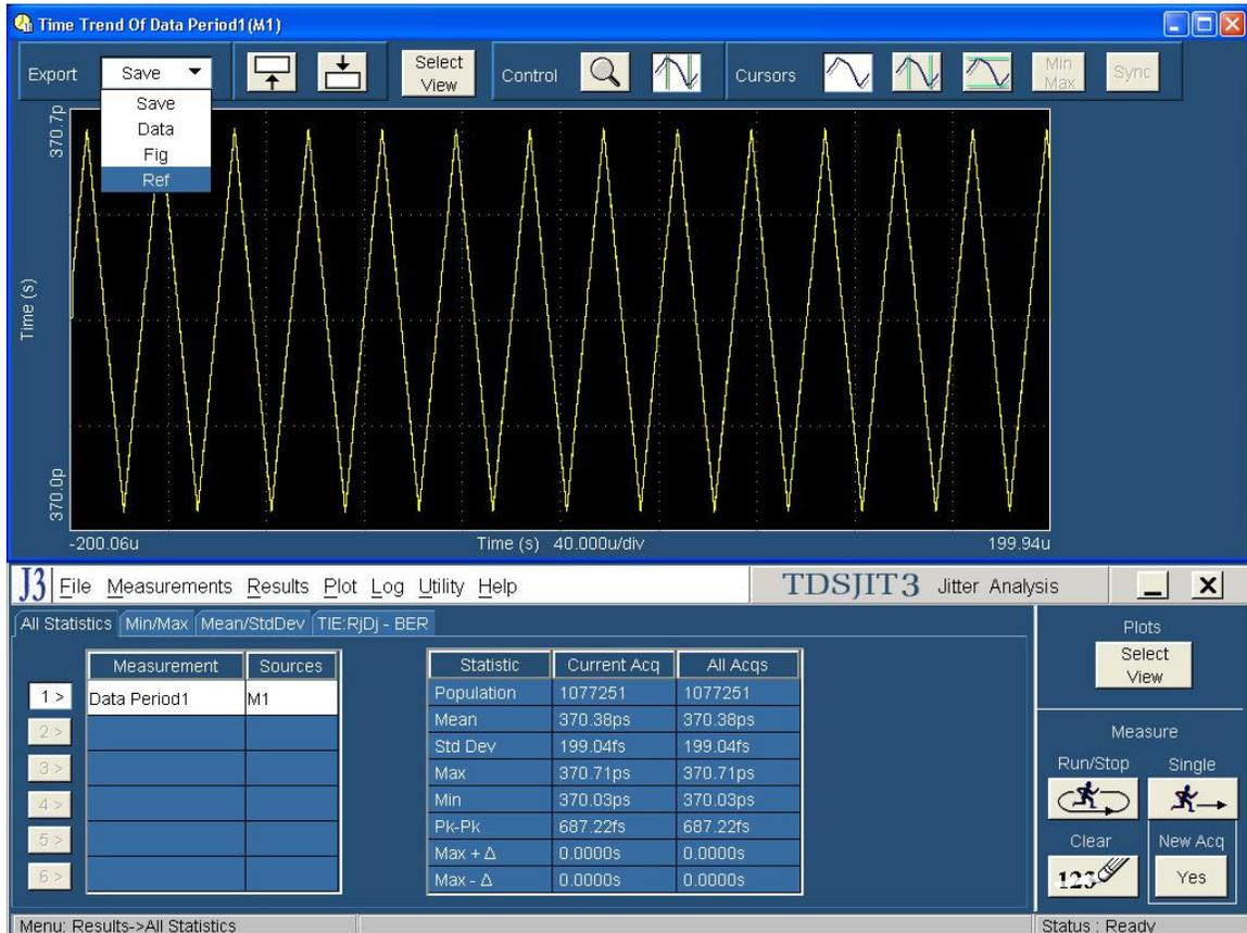
Once the reference waveform is transferred into the scope's storage, minimize the JIT3 screens, so that only the scope UI is displayed.
