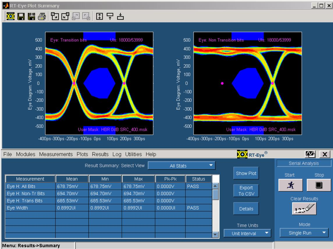
Figure: Eye Diagram measurement result with plots and pass/fail status.
