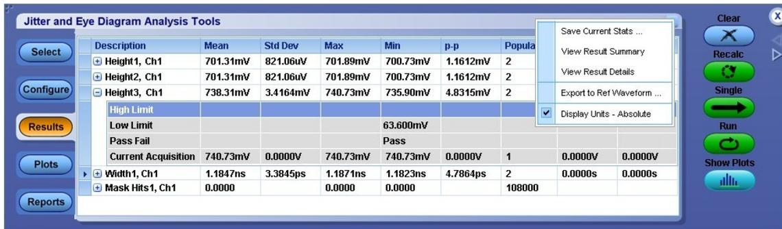
**Figure:** Configuring the results for showing Eye Width in terms of UI (than absolute value in sec.)
