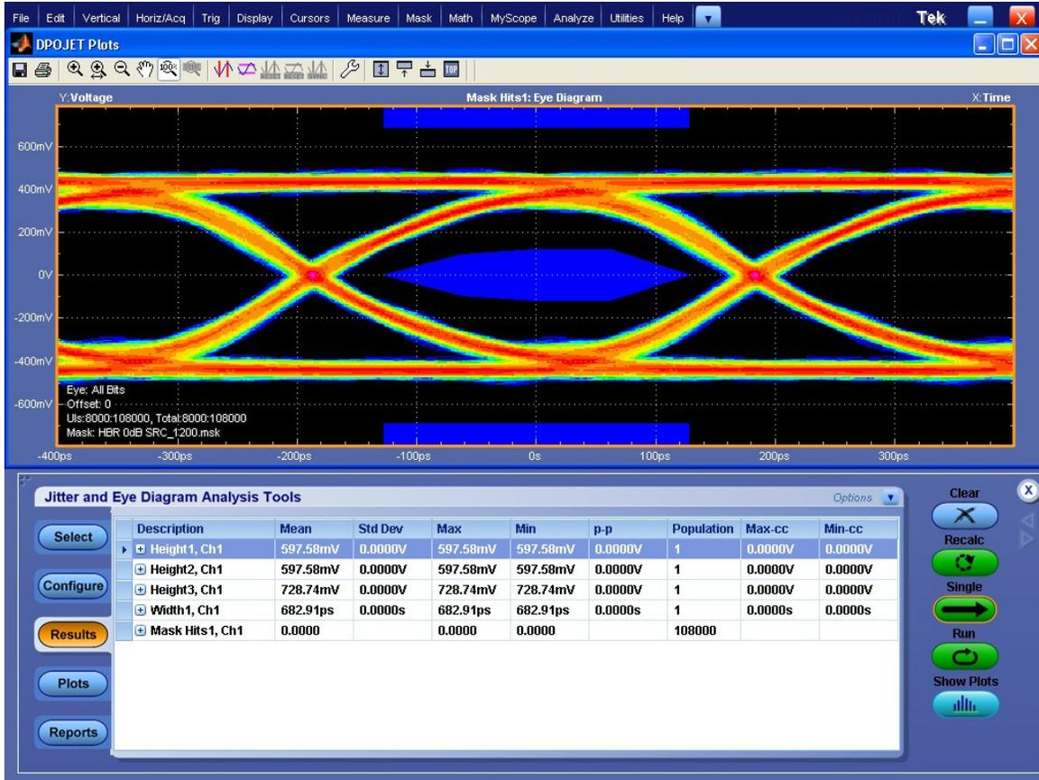
Figure: Eye Diagram test results with Pass/Fails status and eye diagram plots.
