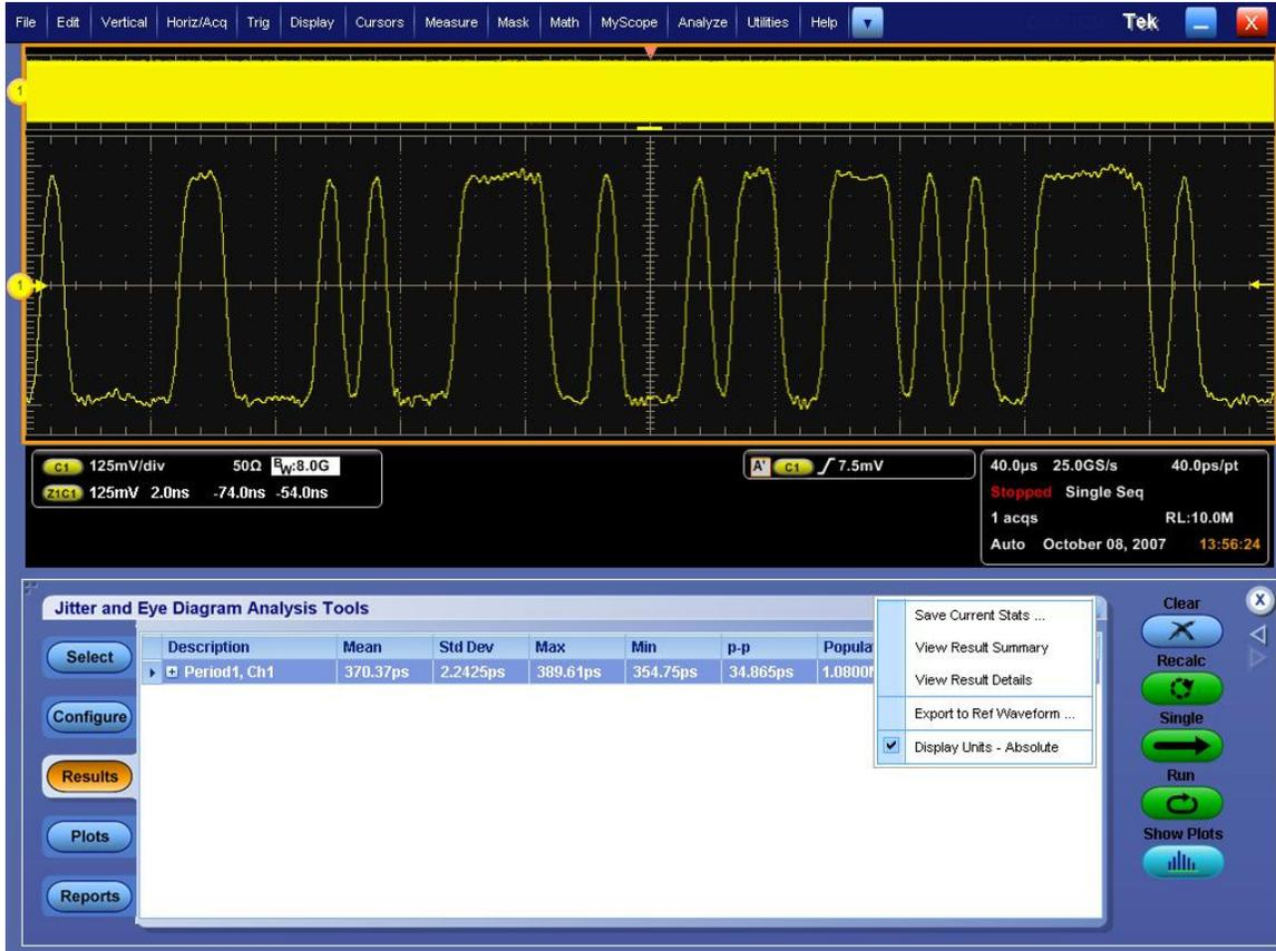
Create a Max and Min measurement (Max will be used for test 3-16). In the Meas menu select Gating using the Cursor method.
