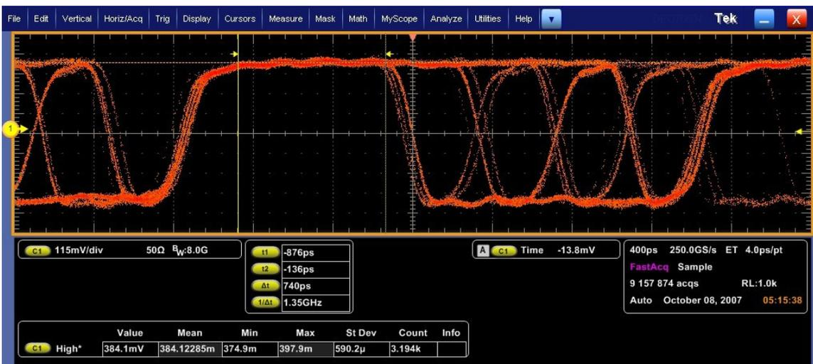
Figure: Screen showing measurement of  $V_H$  with cursor gating enabled
