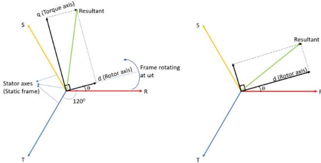
Fig. 2a. Motor with high torque ( $q \gg d$ )
