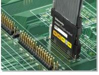
Once we have decided on the test points, we still need to answer the how – that is, which probes that we will use. The cardinal rule is that any probe we use needs to accurately transmit signals from the board to the acquisition system input.
