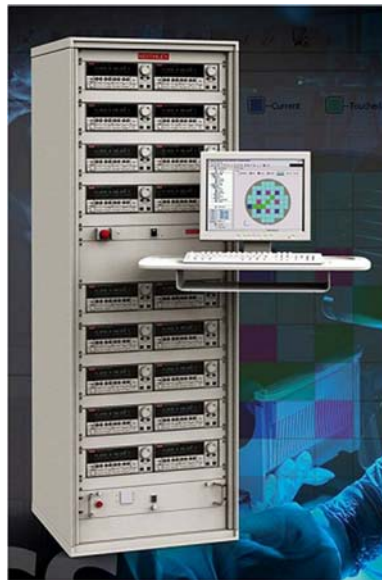
Figure 1. Mainframeless 36-channel semiconductor test system.
