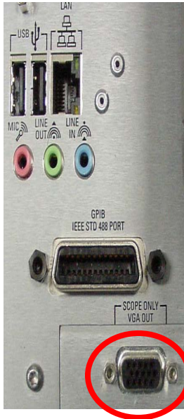
Figure A: TDS5000B VGA OUT port
