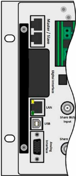
Remove the slot cover. If needed, use a screw driver.
