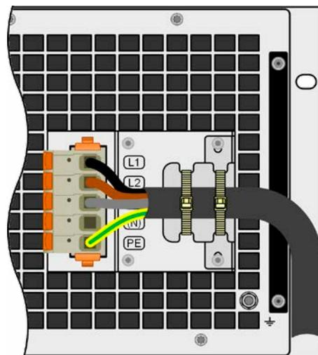
Figure 11 - Fully installed strain relief
