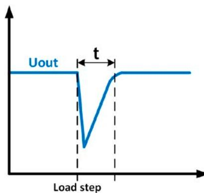
Example for a pos. load step: the DC output will collapse below the adjusted value for a short time.  $t$  = transient time to settle the output voltage.
