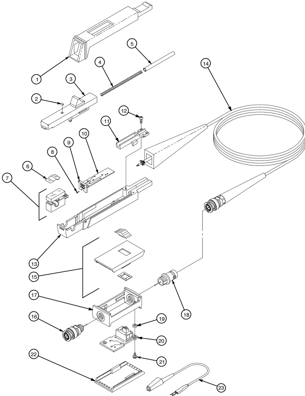
Figure 13: P6021 exploded view
