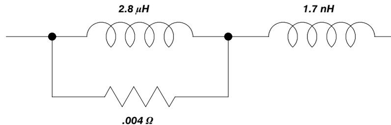
**Figure 2: Insertion Impedance of the P6021**
