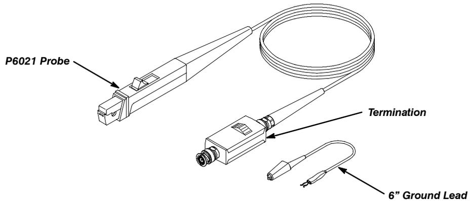
**Figure 1: The P6021 Probe and termination**
