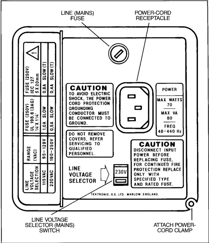
Figure 1-1. Voltage selector switch, fuse, and power-cord receptacle.
