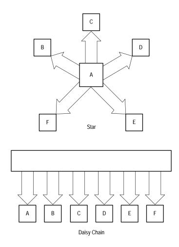
Figure 1-4: Connecting Multiple Instruments on the GPIB
