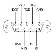
Figure A-2: Rear Panel RS-232 Connector
