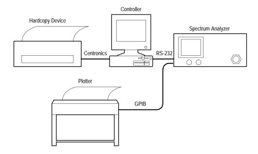
Figure 1–3: Typical Small Instrument System for GPIB
