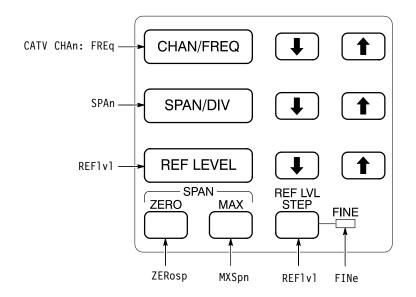
Table 3-4: FREQUENCY, SPAN/DIV and REF LEVEL Front Panel Commands
