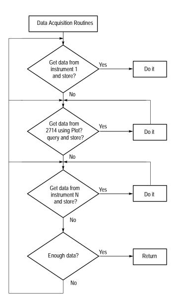
Figure 6–8: Possible Data Acquisition Scheme
