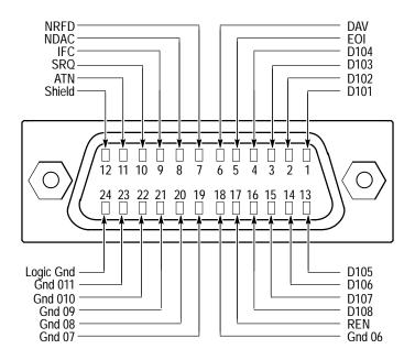
Figure B-1: IEEE Std 488.1 (GPIB) Connector
