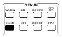
**DEMOD MENU** 0 OFF 1 AM DEMODULATOR **DETector** 2 FM DEMODULATOR 3 BROADCAST (AM) VIDEO VMOnitor 9 VIDEO SETUP MENU **BROADCAST** 0 VIDEO DETECT MODE VDMode **POSITIVE** 1 SYNC POLARITY VSYnc 2 VIDEO POLARITY **NEGATIVE VPOlarity**
