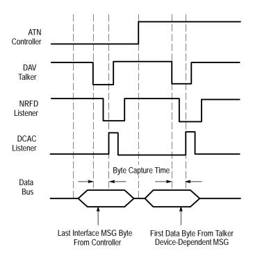
Figure B-4: Handshake Timing Sequence, Idealized
