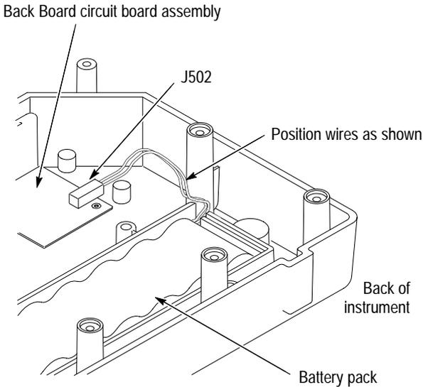
**Figure 6-5: Removing the Back Board circuit board assembly**
