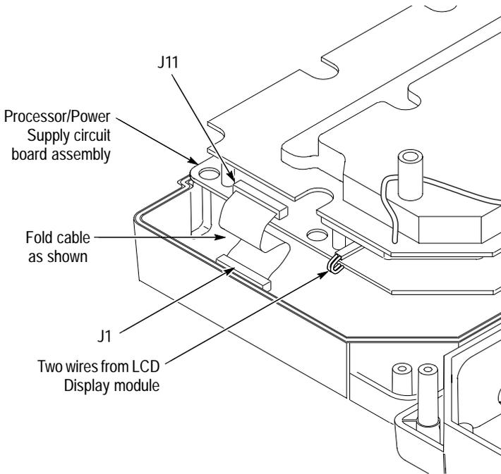
**Figure 6-6: Positioning the ribbon cable**
