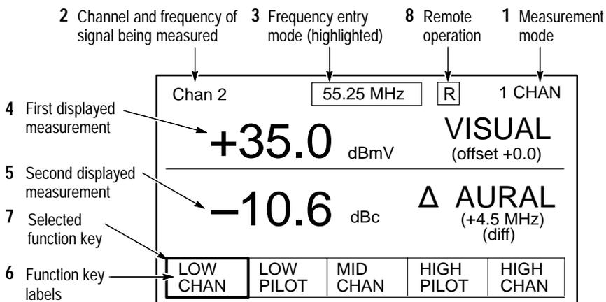
Figure 2-4: Display readouts and labels
