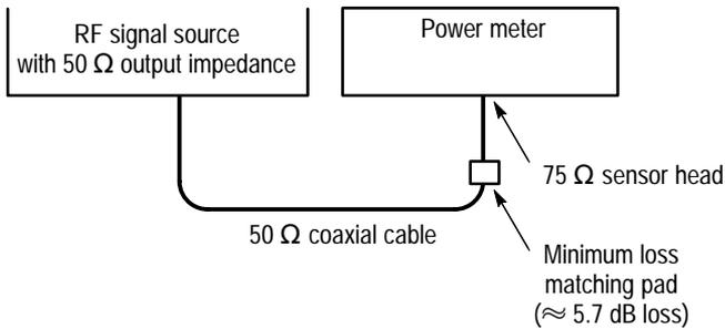
**Figure 5-2: Alternate hookup for 50  $\Omega$  source output**
