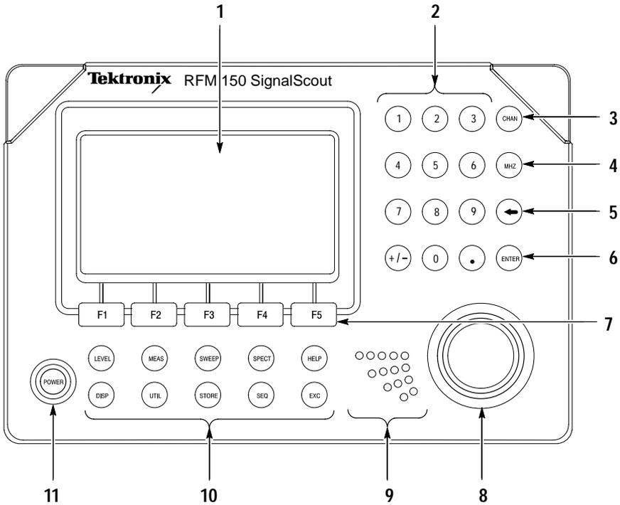
Figure 2-2: The RFM 150 front panel, showing controls
