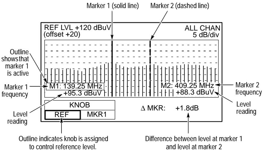
Figure 2–11: The all channel mode display
