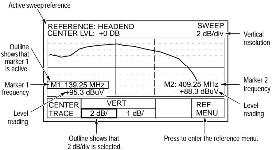
Figure 2–21: The sweep LVL/REF submenu display
