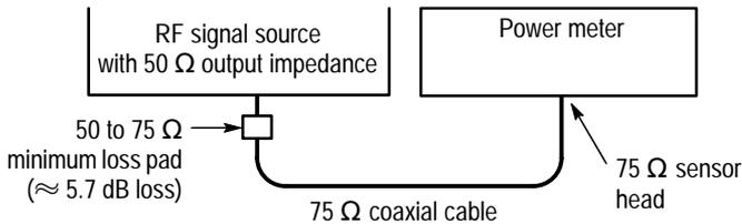
Figure 5–1: Hookup for 50  $\Omega$  source output
