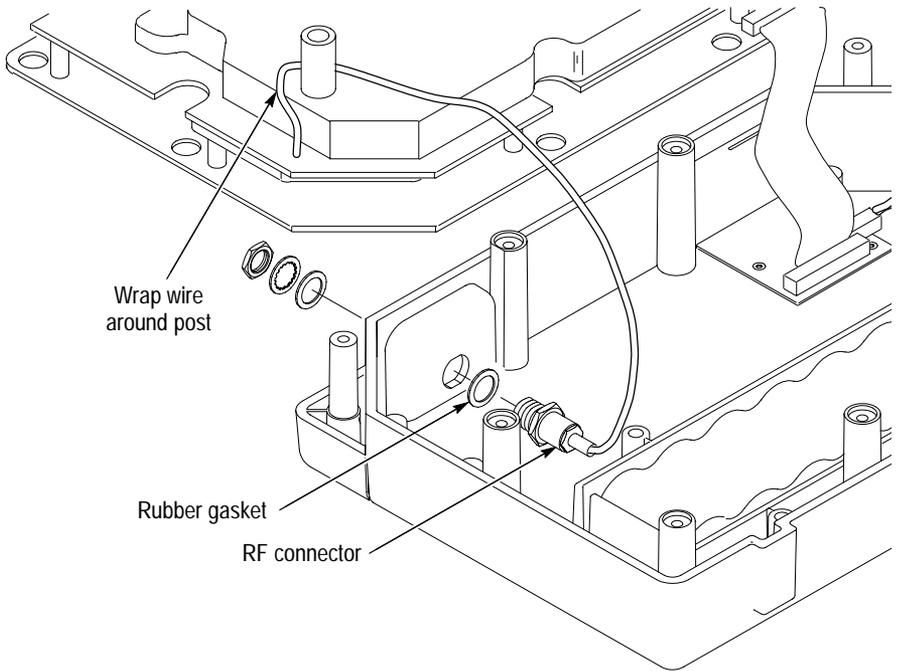
**Figure 6-7: Installing the RF connector**
