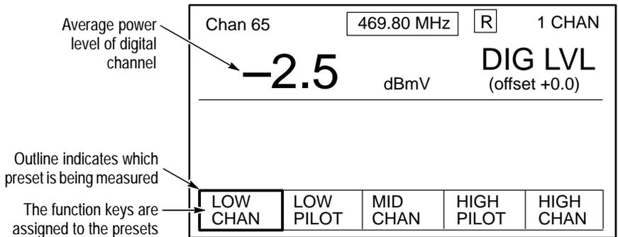
Figure 2–8: The 1 channel mode (digital channel)
