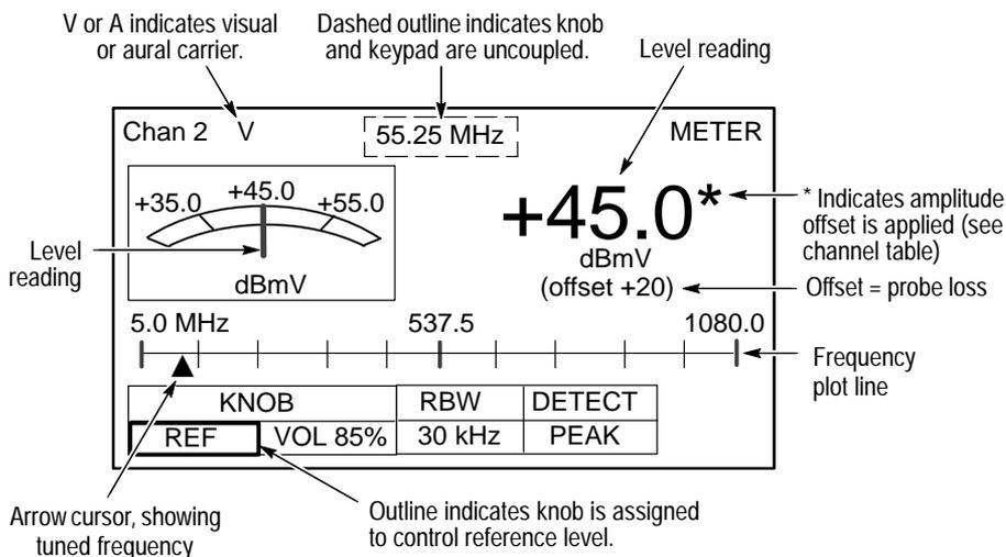
Figure 2–12: The meter mode display
