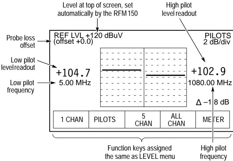
Figure 2–9: The pilots mode display
