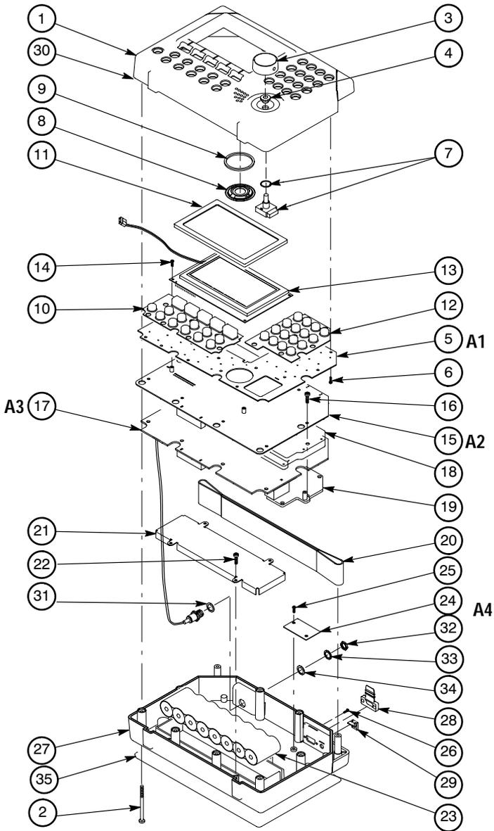
Figure 8-1: Exploded view of the RFM 150
