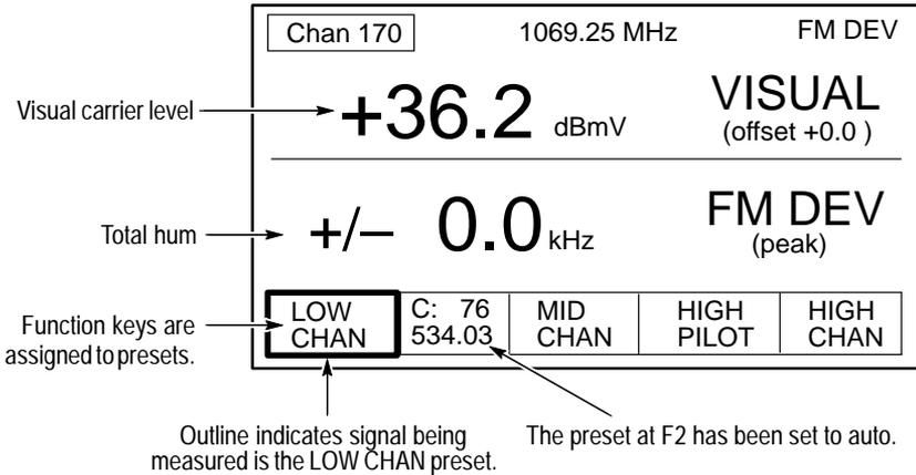
Figure 2-16: The FM deviation measurement mode display
