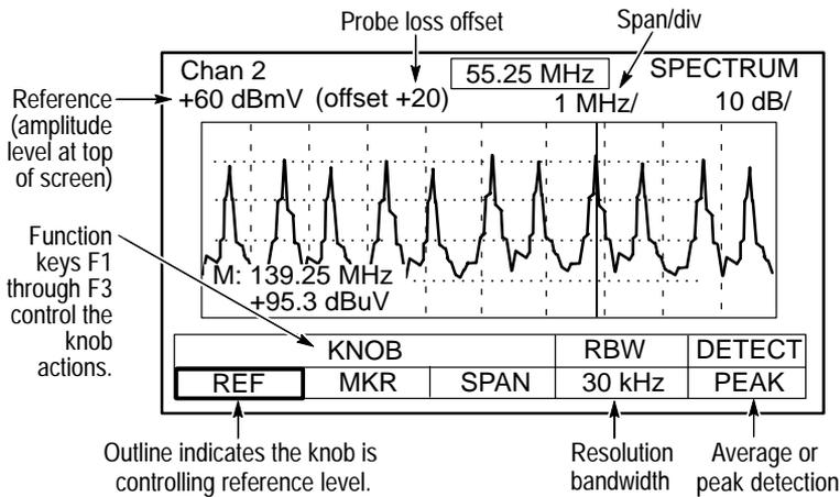
Figure 2–19: The Spectrum mode display (analog channel)
