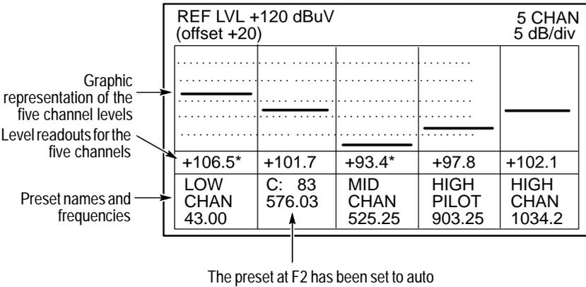
**Figure 2–10: The 5 channel mode display**
