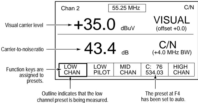
**Figure 2–13: The carrier-to-noise measurement screen (analog channel)**
