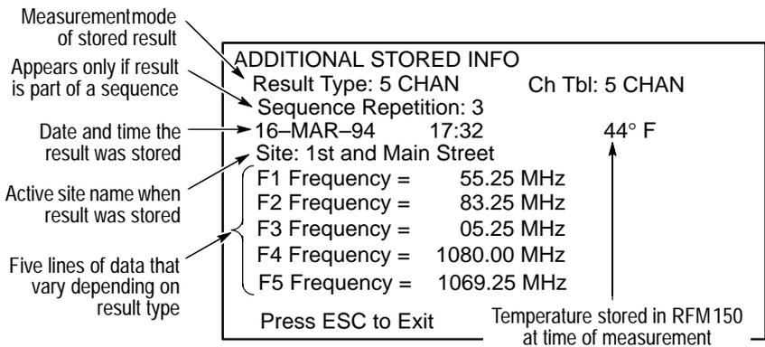
**Figure 3–11: Additional information screen for 5 channel measurement type**
