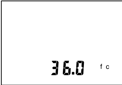
Figure 1–9: Typical Single Channel Display
