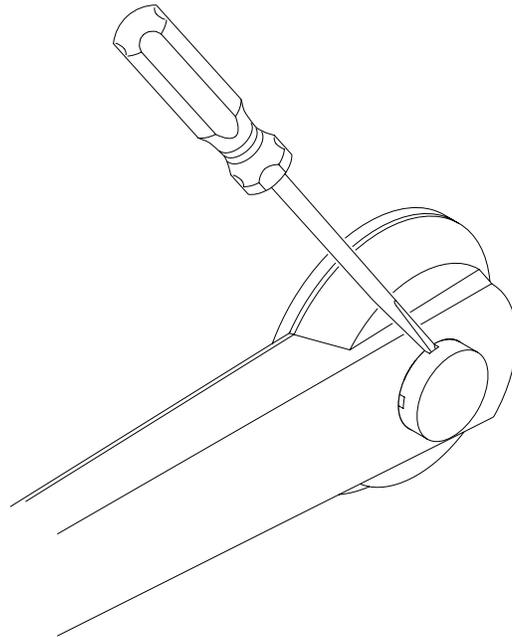
**Figure 6–52: Removing the thumb release button from the swing arm**
