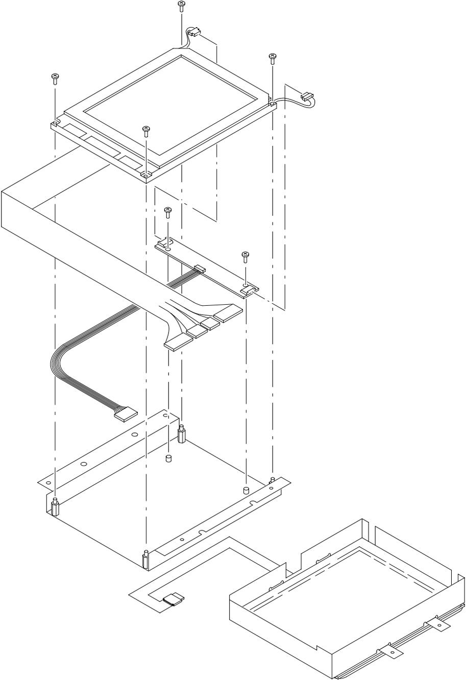
Figure 6-41: LCD assembly exploded view serial number B020100 to B020632
