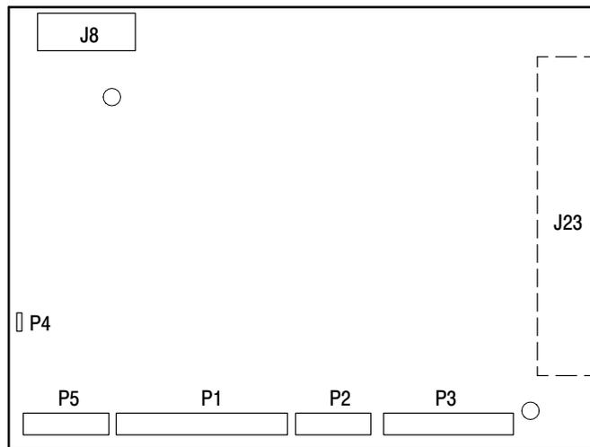
**Figure 6–29: LCD Display Driver board with connector locations**
