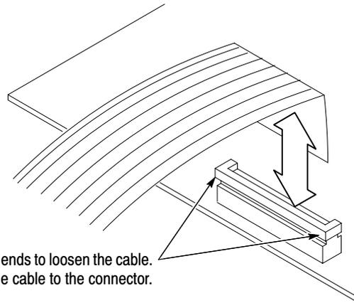
**Figure 5–3: Disk drive flexible circuit board connector operation**
