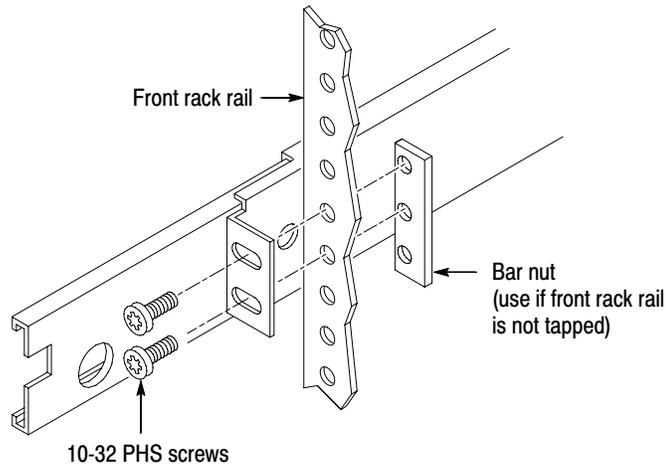
**Figure 6-49: Mounting the slide to the front rail**
