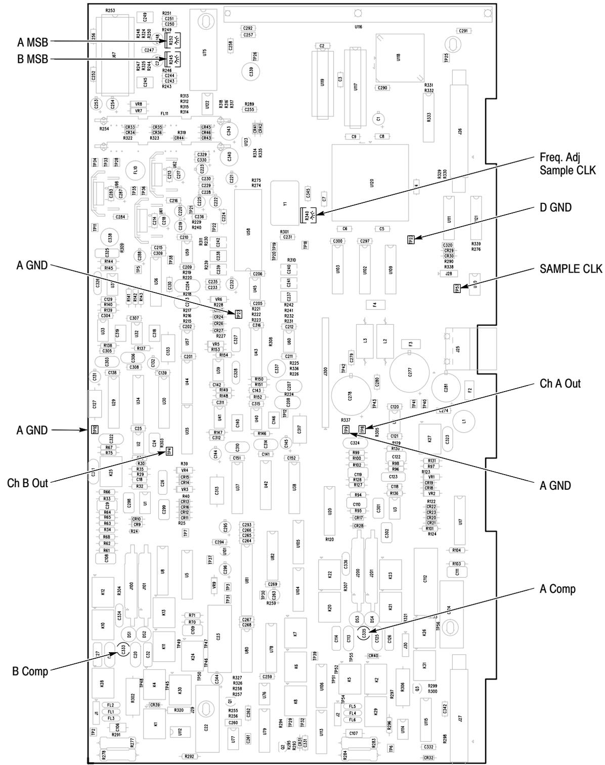
Figure 5-2: Acquisition board test points and adjustment locations
