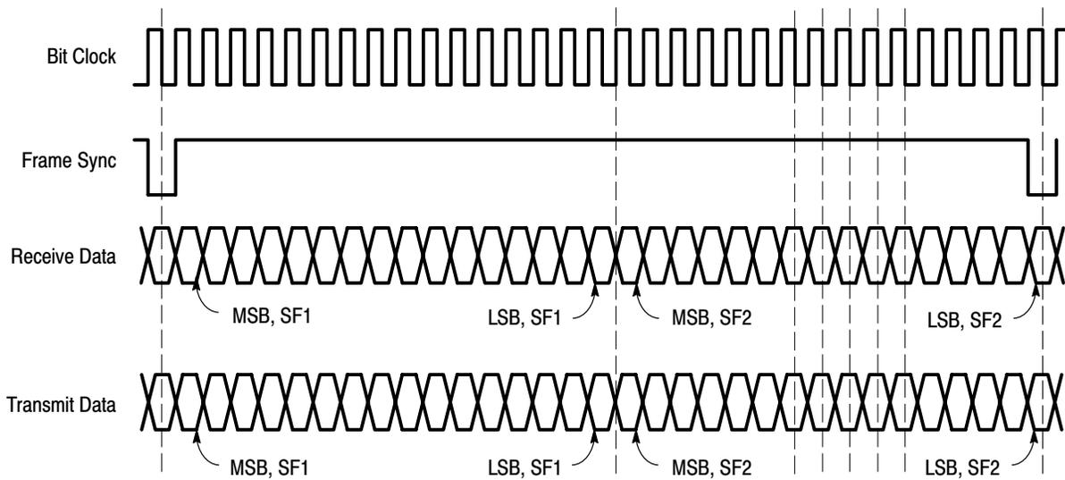
NOTE: All Data is sampled on the FALLING edge of Bit Clock.
