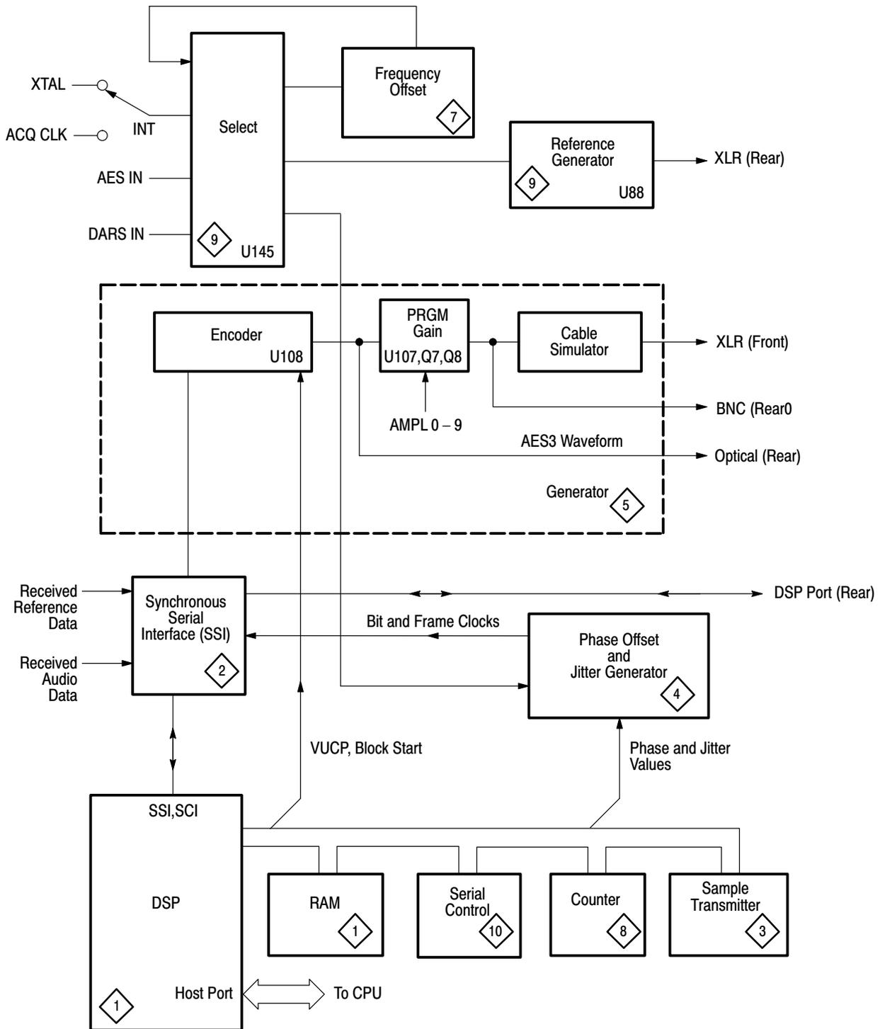
Figure 3-5: Digital audio generator simplified block diagram
