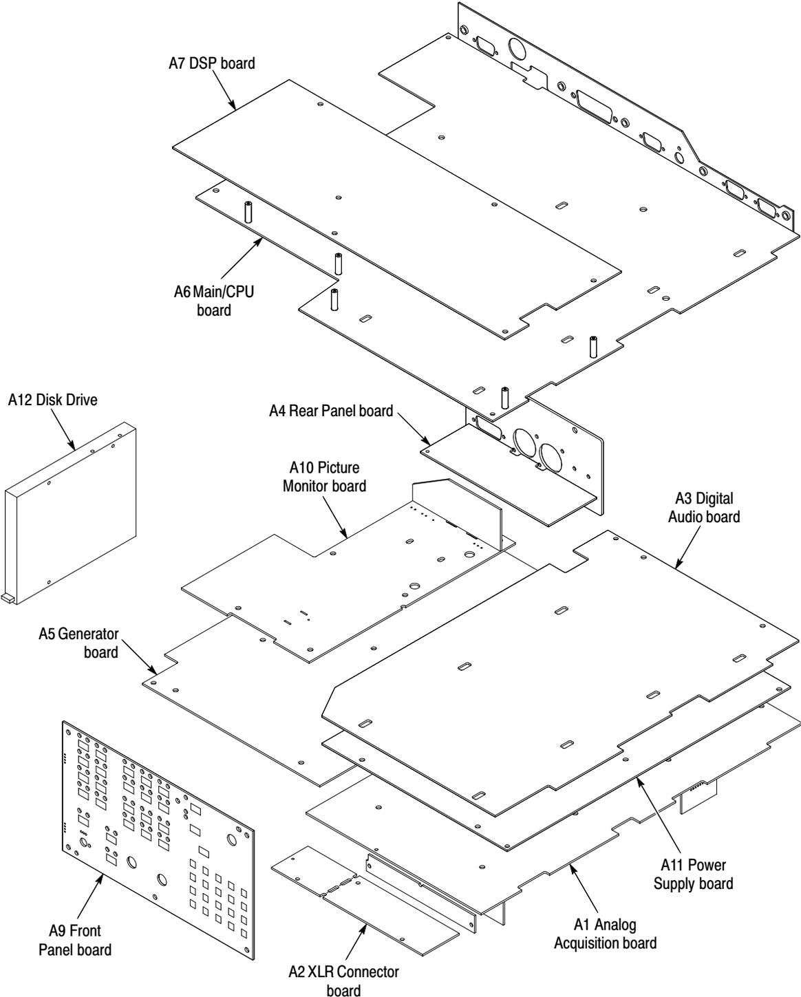
Figure 6-19: Circuit board assemblies for CRT display version
