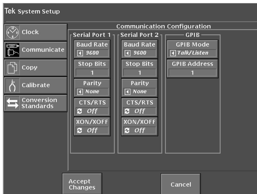
**Figure 4–27: GPIB setup in the communications configuration screen**
