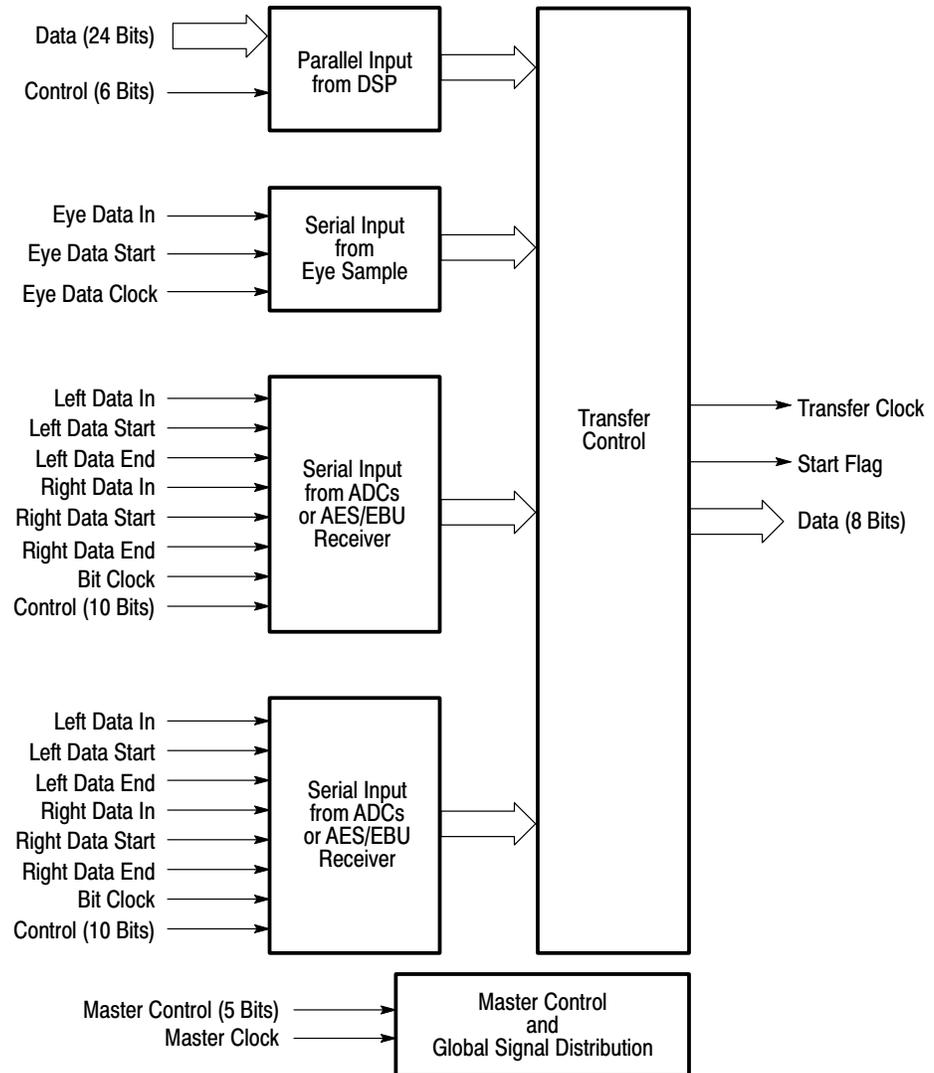
**Figure 3–4: Sample transmitter block diagram**
