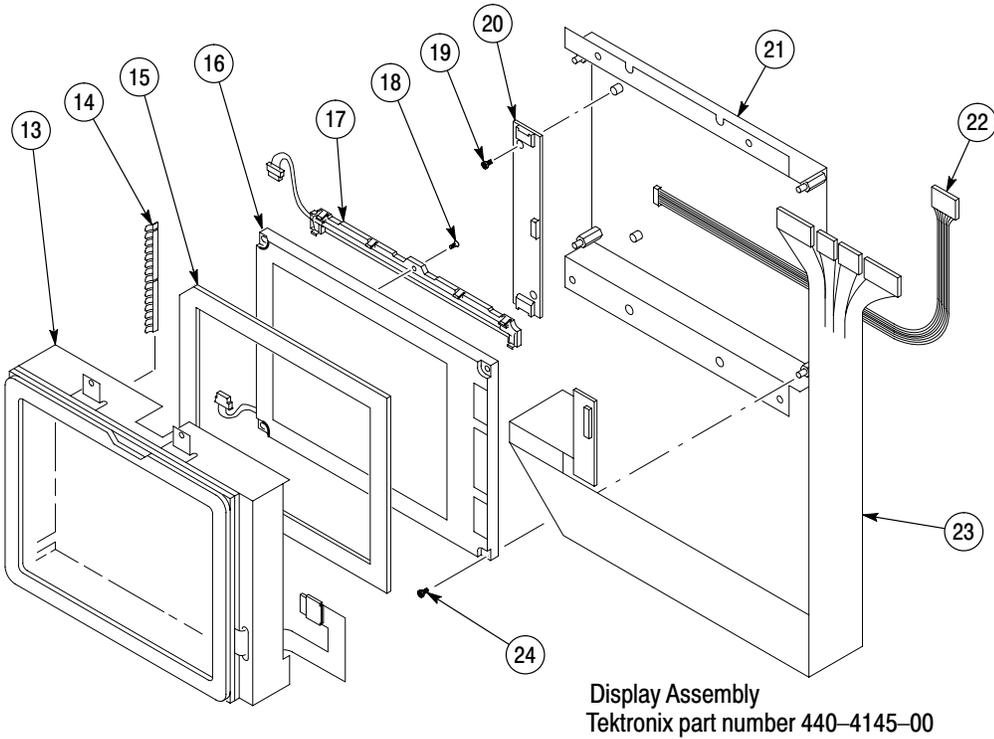
**Figure 10-7: LCD display assembly subparts – SN B020100 and above**
