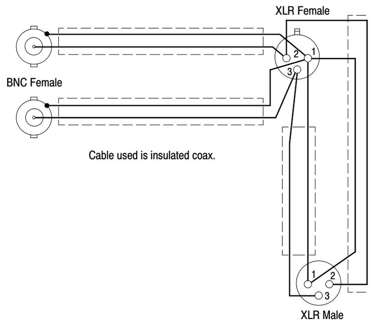
**Figure 4–19: Dual BNC to dual XLR cable adapter**
