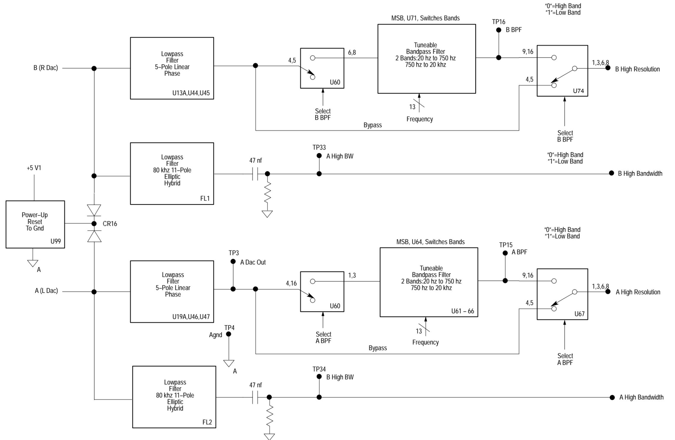
Figure 9-11: Analog Generator, analog filters block diagram
