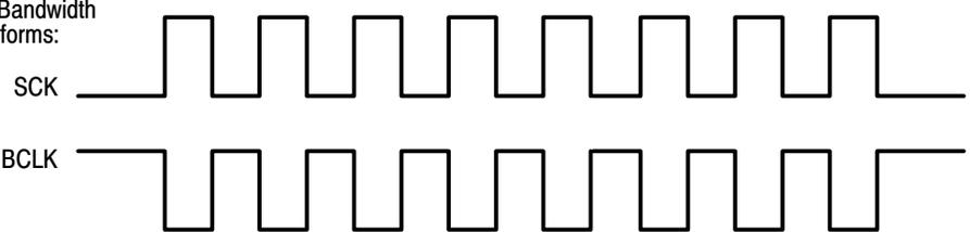
**Figure 3–13: S-Clock disable used for DSP mode control**
