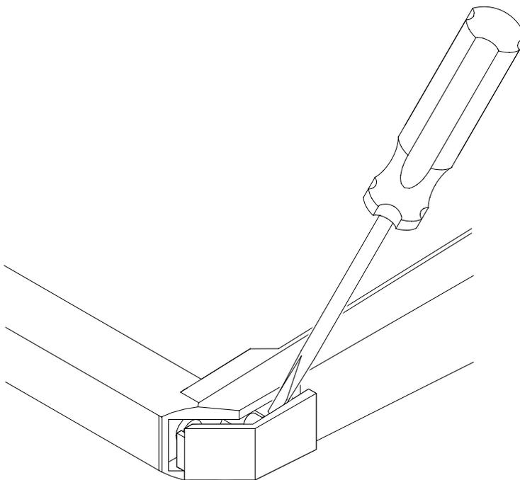
**Figure 6-51: Removing the plastic handle screw cover**
