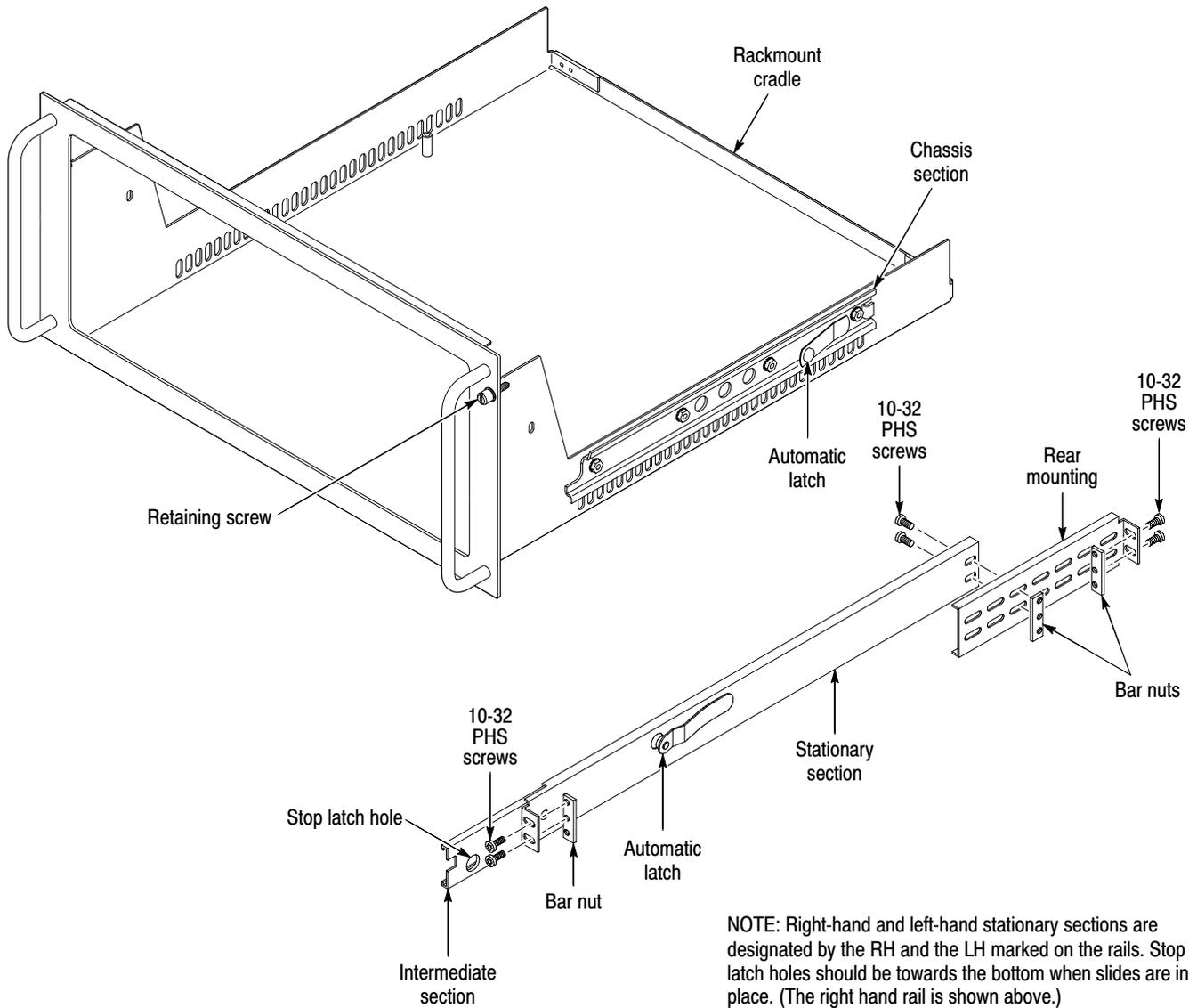
Figure 6-47: Exploded view of the slide-out track assembly
