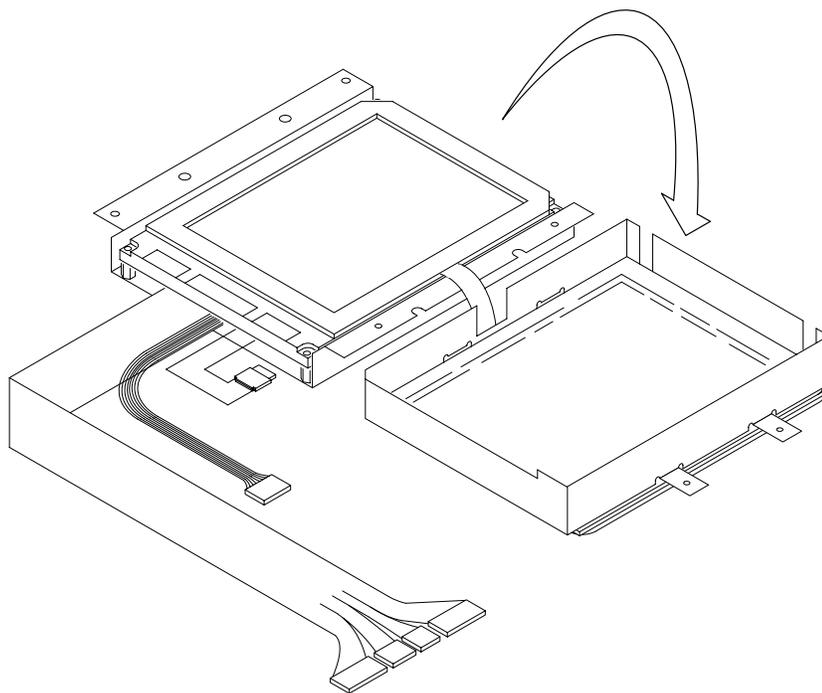
**Figure 6–39: Touch screen assembly removal B020253 to B020692**
