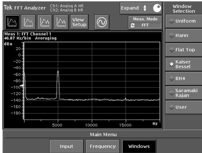
Figure 4–17: FFT Analyzer Window menu display
