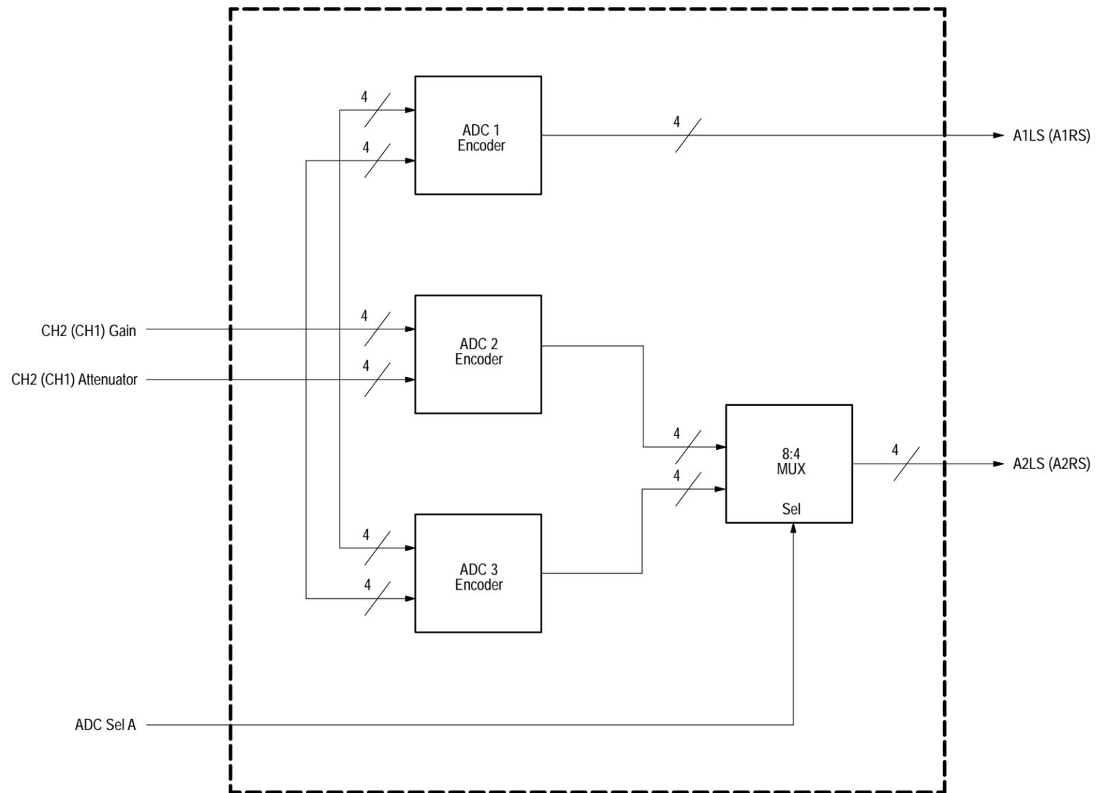
Figure 9-6: Analog acquisition, part 2 of the data formatter PAL
