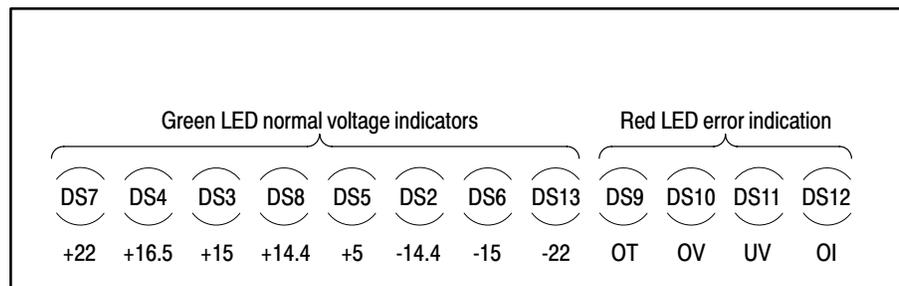
**Figure 6–2: Power supply status indicators for the CRT display power supply**
