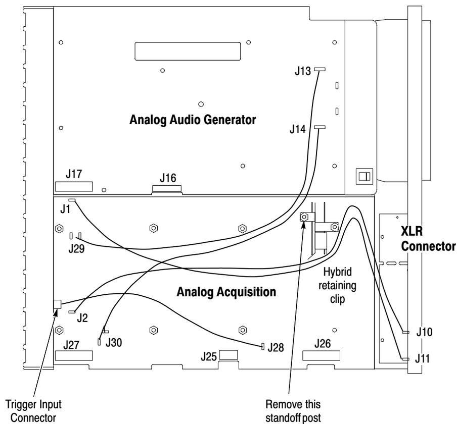
**Figure 6–24: Bottom view showing the connections to the Analog Acquisition board**
