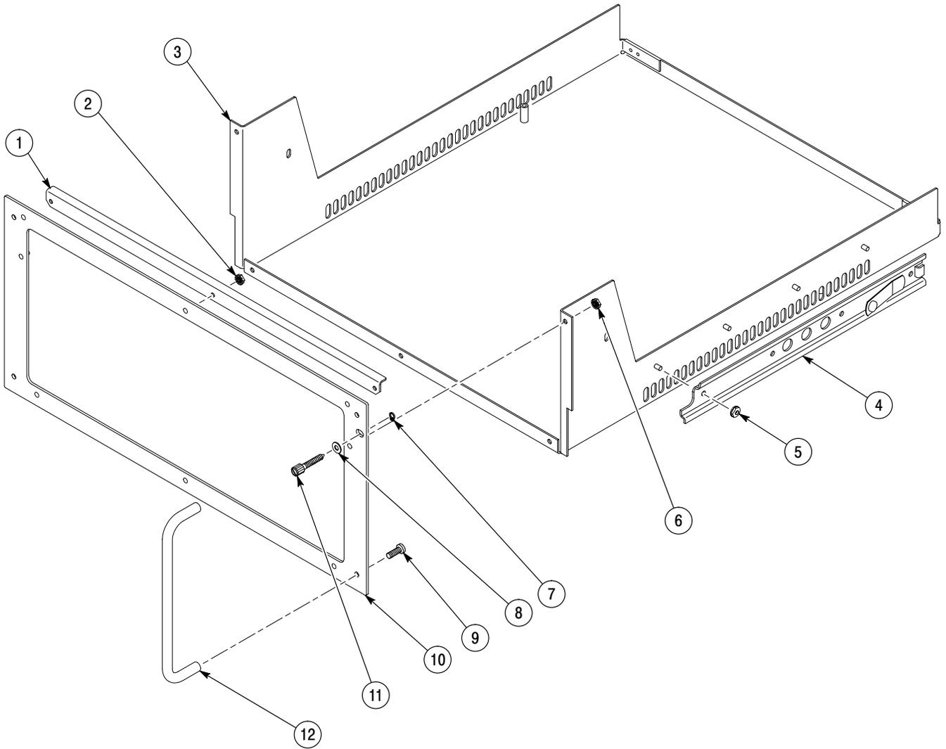
Figure 6-55: Exploded view of the rack adapter assembly
