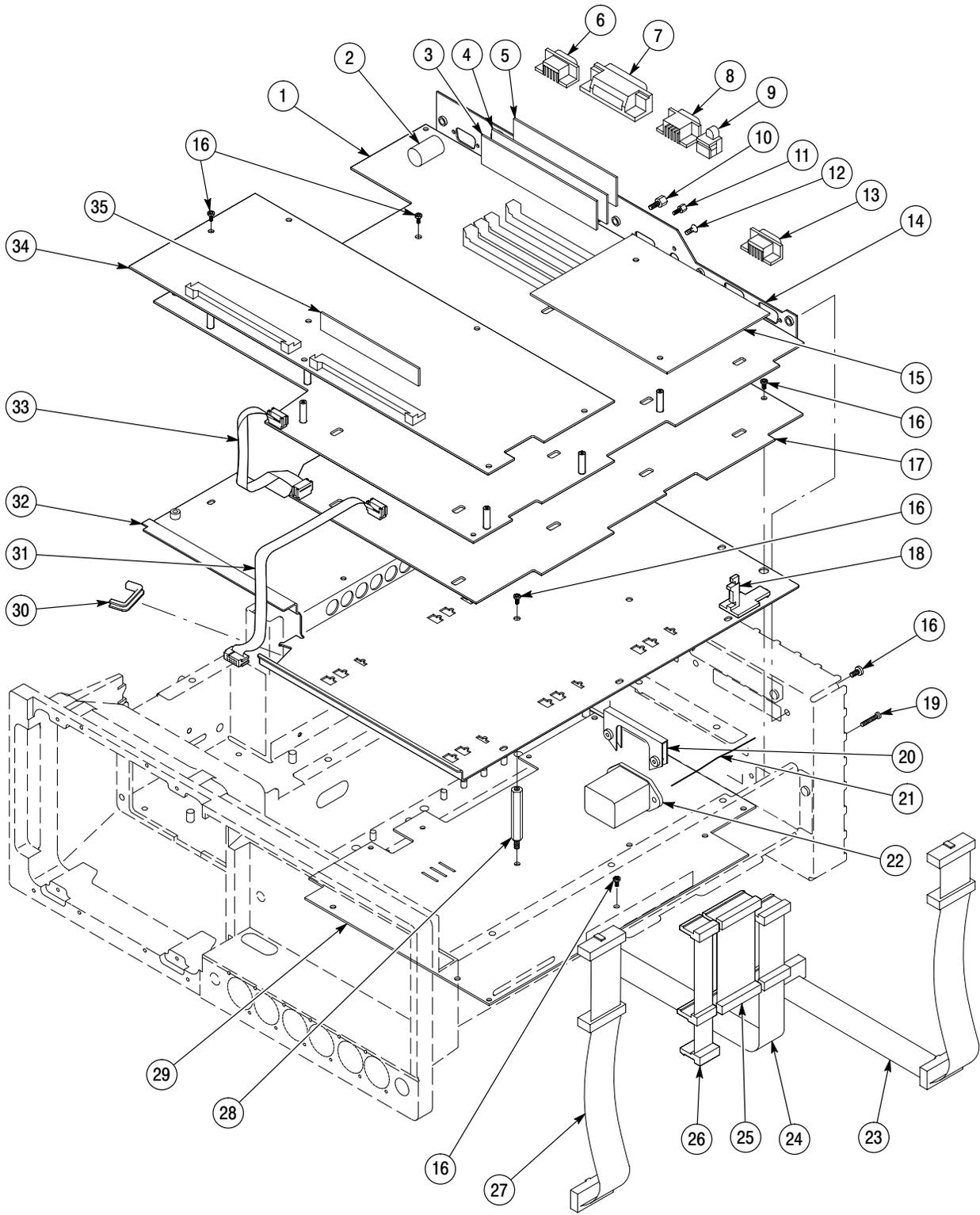
Figure 10-4: Top view – SN B020100 and above only
