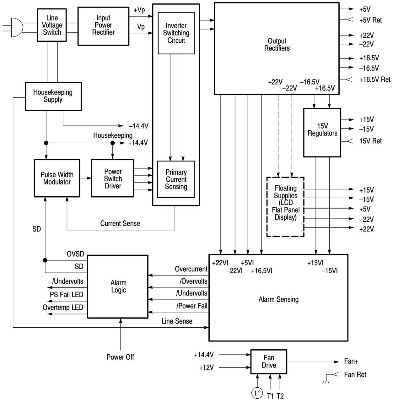
Figure 3–20: Power supply block diagram
