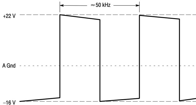
**Figure 3-15: Switching waveform for -15 V floating power supply**
