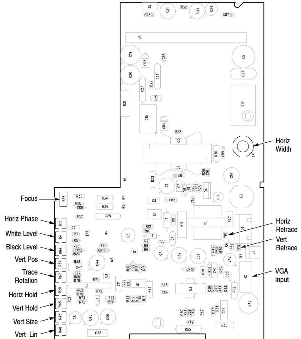
**Figure 5-4: CRT display monitor board adjustment locations**
