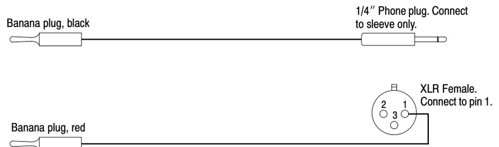
**Figure 4–11: Impedance check adapter cables**
