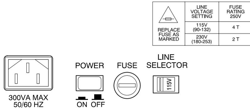
Figure 2-1: Rear panel fuse, power connector, On/Off Switch, and line selector
