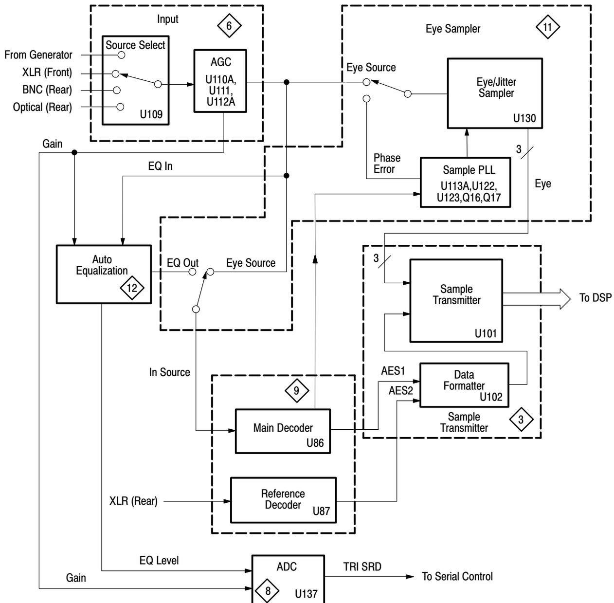
Figure 3-7: Digital audio receiver simplified block diagram
