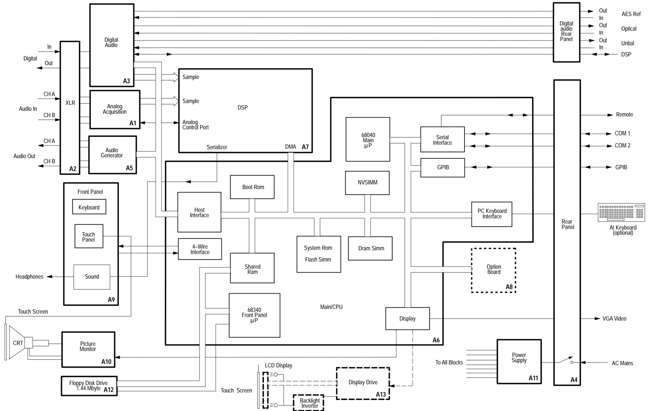
Figure 9-1: AM700 overall block diagram
