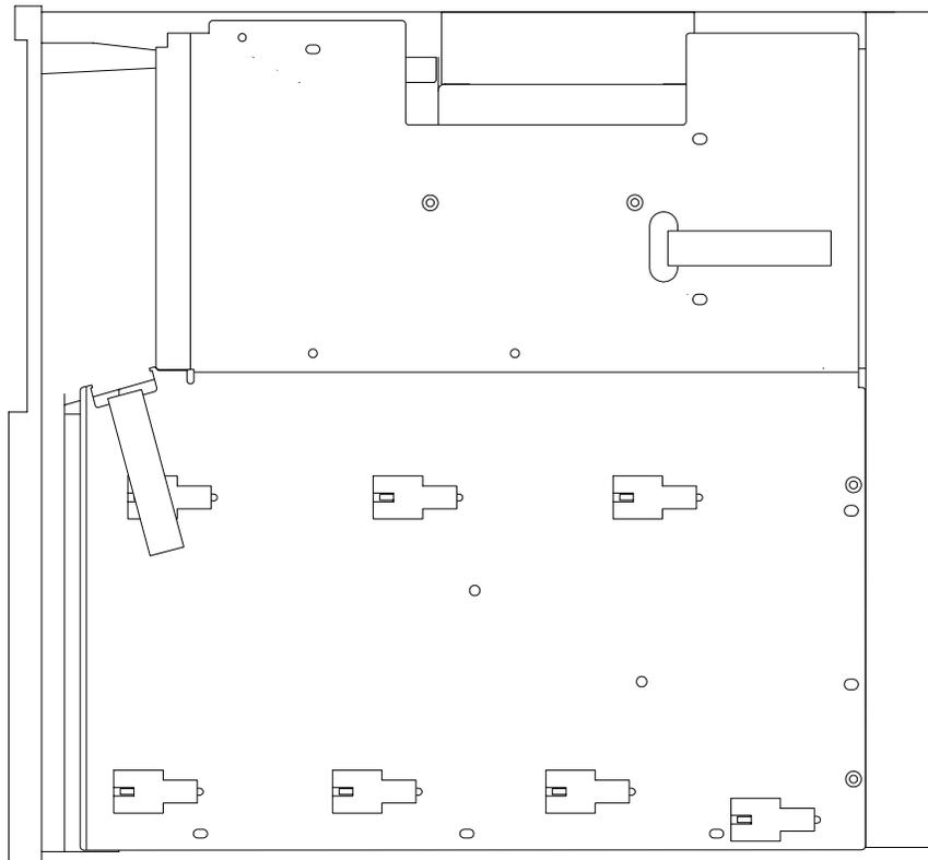
**Figure 6-37: Power supply and monitor board cover plate screws and cables (CRT display version)**
