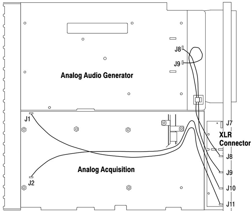
**Figure 6-26: Bottom view showing the XLR connector board cable connections**
