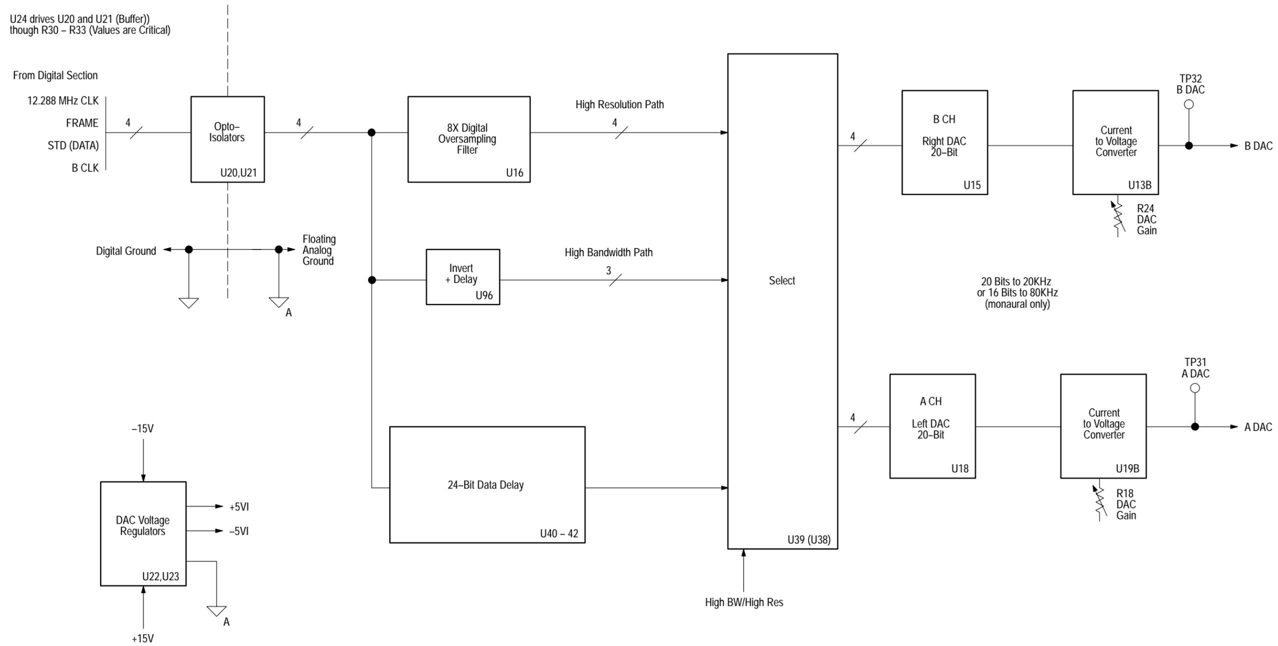
Figure 9-10: Analog generator DAC and current-to-voltage converters
