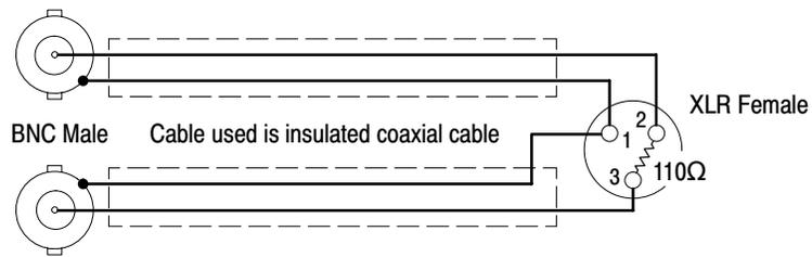
**Figure 4–18: Dual BNC to 110 Ω XLR adapter cable**
