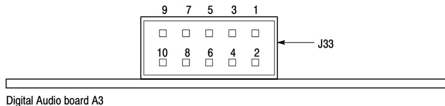
**Figure 5–7: Pin arrangement for J33, the PLL voltage test points**
