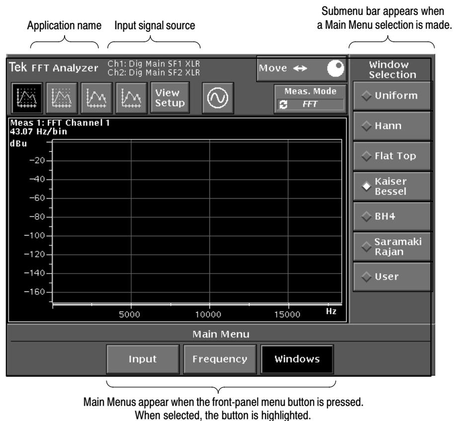
**Figure 2–2: Touch screen interface with main menu and submenu displayed**
