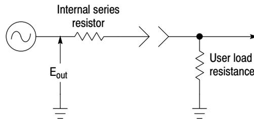
**Figure 2-21: Generator output voltage divider for dBm calculations**
