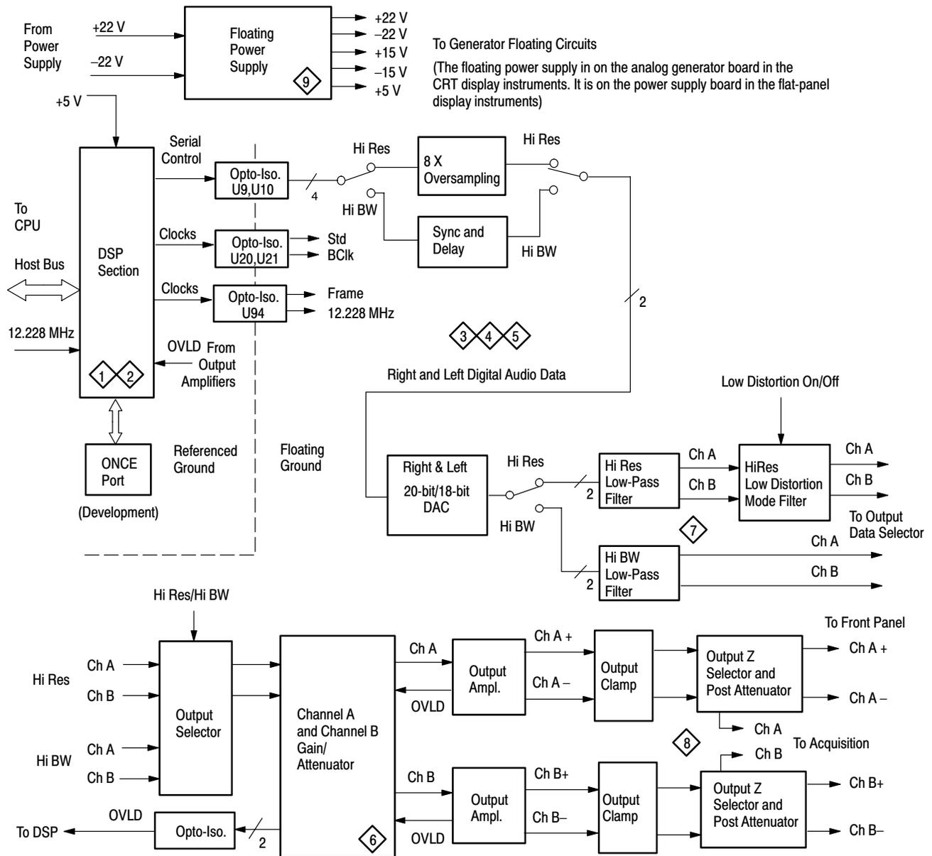
Figure 3–11: Analog generator simplified block diagram
