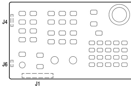
**Figure 6-34: Front panel board connector locations**
