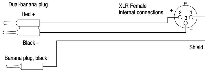
**Figure 4–7: Cable for generator output level check**
