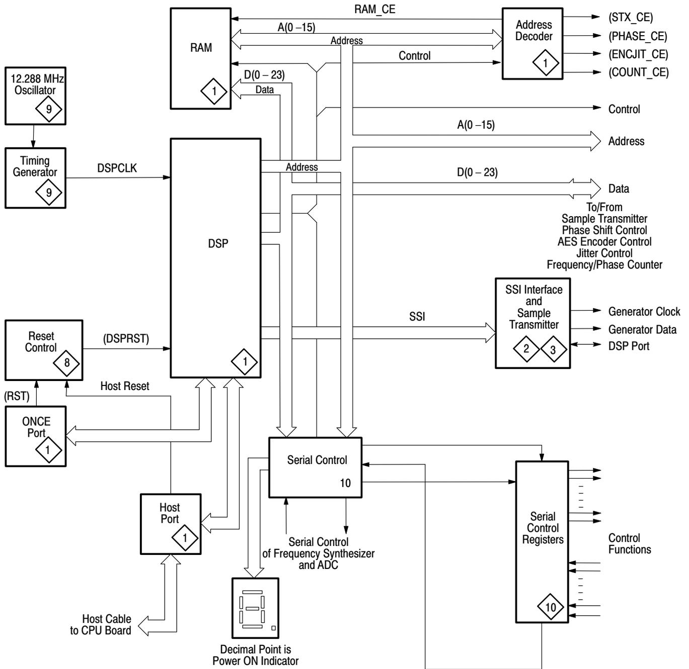
Figure 3-6: Digital audio board DSP section block diagram
