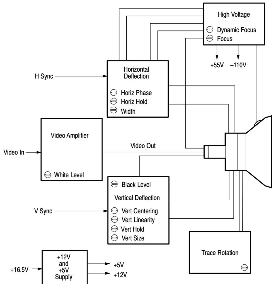
Figure 3–19: Picture monitor simplified block diagram
