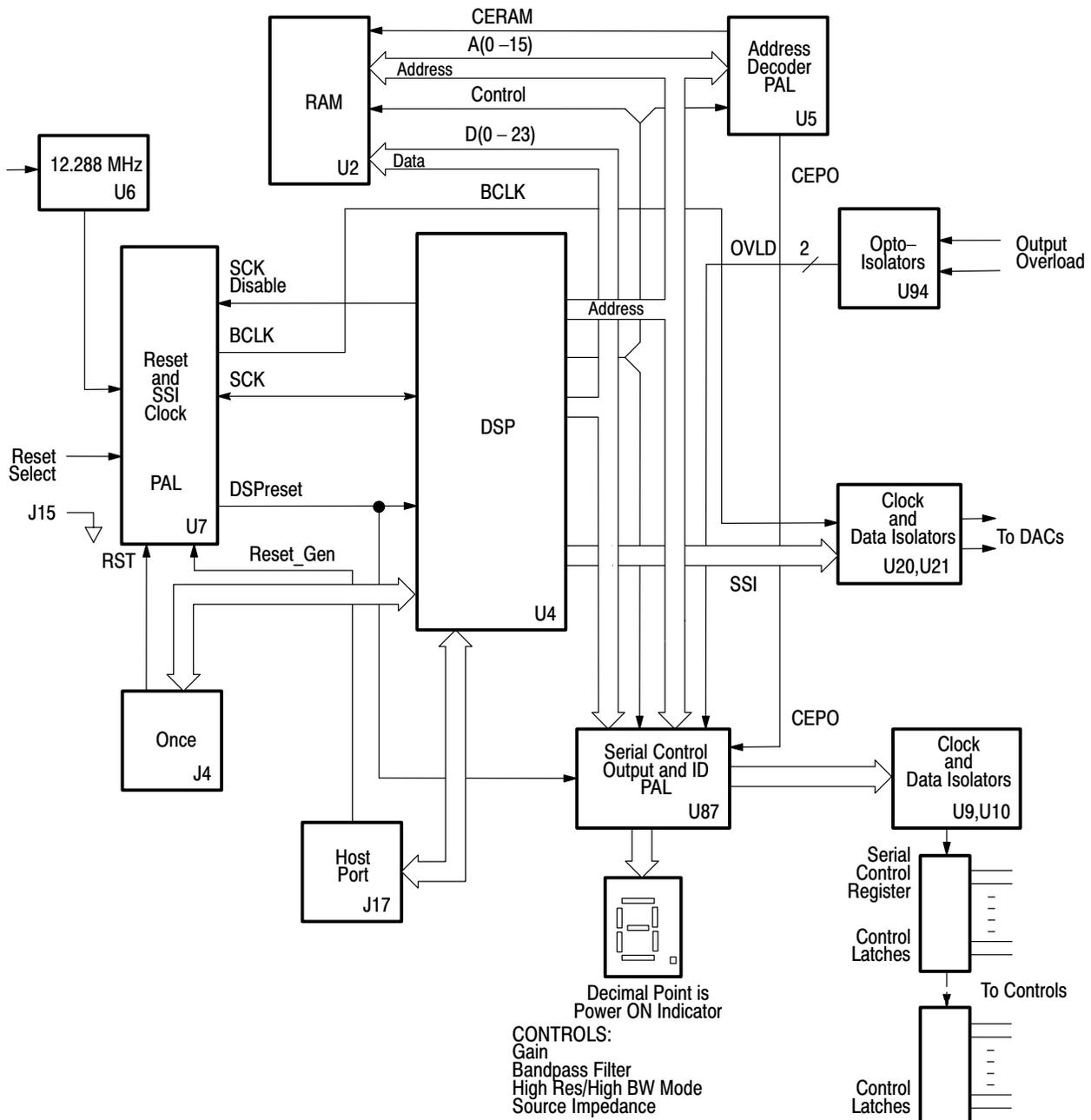
Figure 3-12: Analog generator DSP section block diagram
