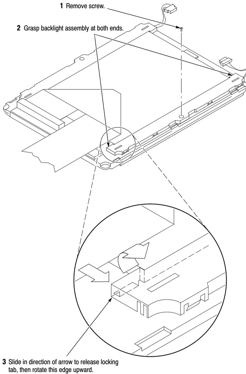
**Figure 6-42: Backlight removal**
