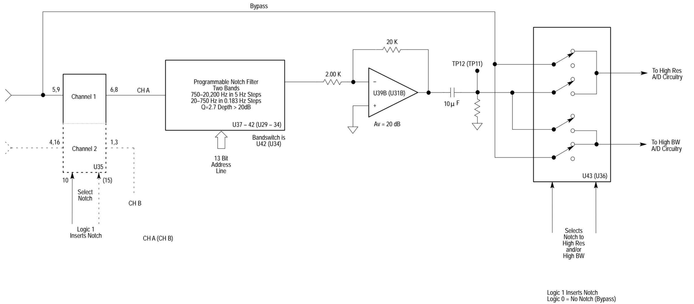
Figure 9-3: Analog Acquisition input section CH A notch filter
