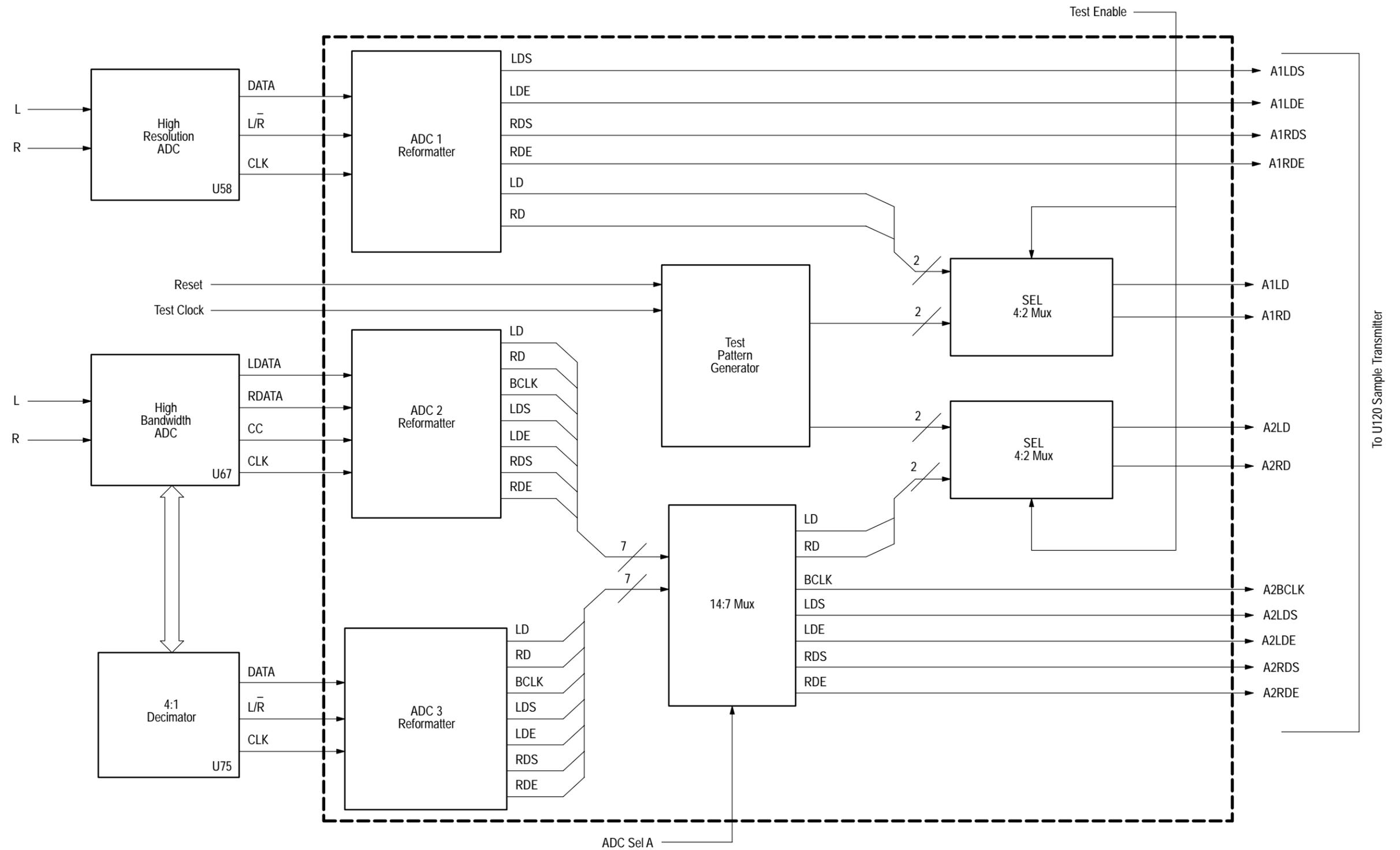
Figure 9-5: Analog acquisition, part 1 of data formatter PAL
