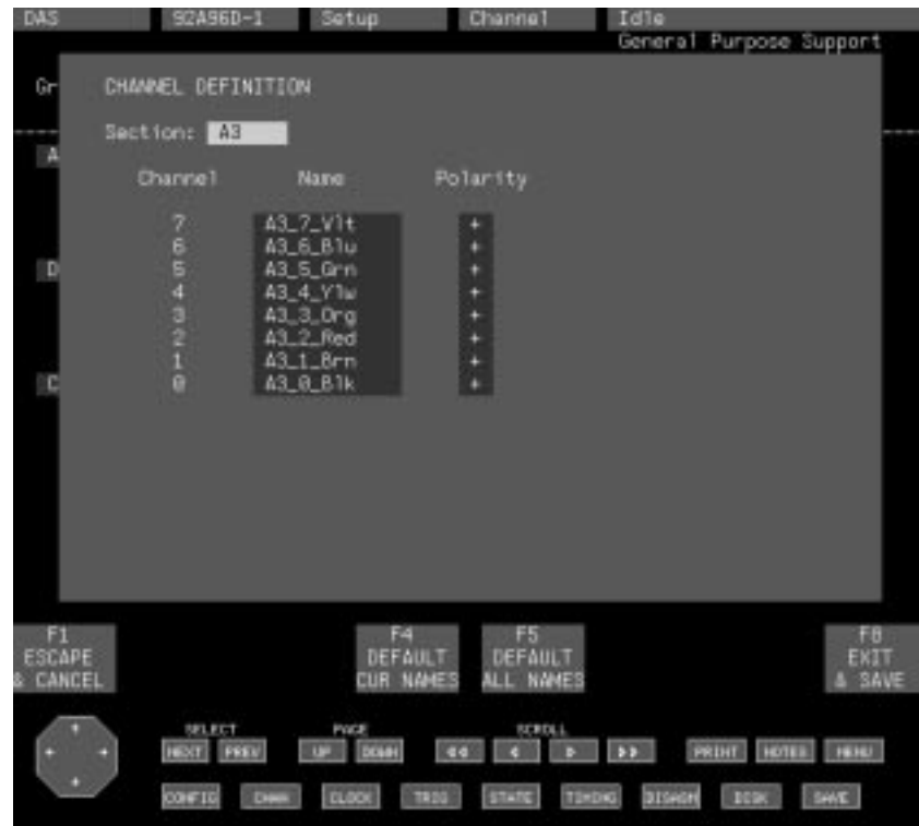
Figure 3–6: Channel Definition Overlay (Section Field Open)
