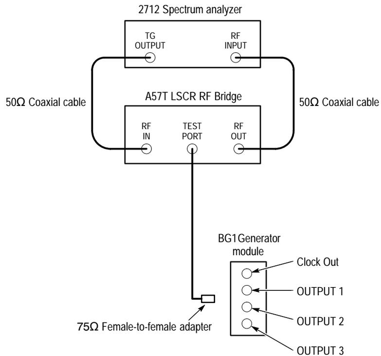
**Figure 4–1: Equipment hookup for checking return loss**
