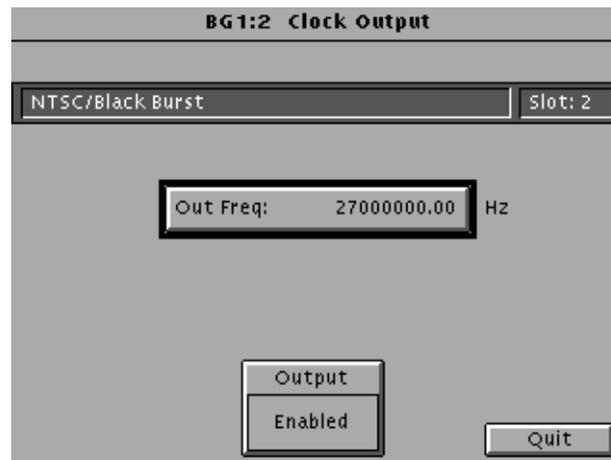
3. To set the clock frequency, touch **Out Freq:** on the display. Set the frequency using one of the following methods:
