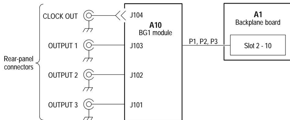
Figure 3–1: BG1 module block diagram
