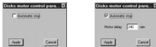
Figure 3–21: Specifying automatic motor control parameters
