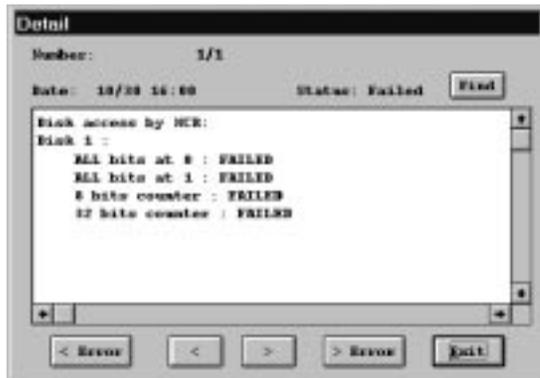
Figure 6–24: Disk access by NCR failure
