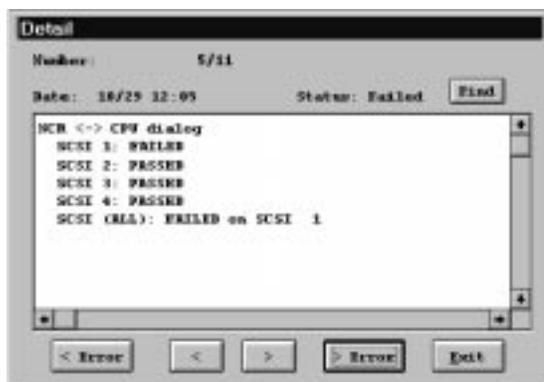
Figure 6–22: NCR <-> CPU failure
