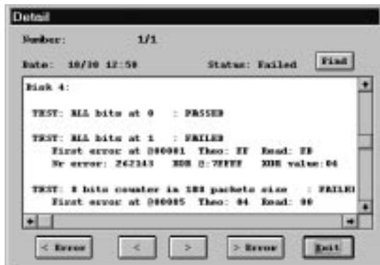
Figure 6–25: Disk access by DMA failure
