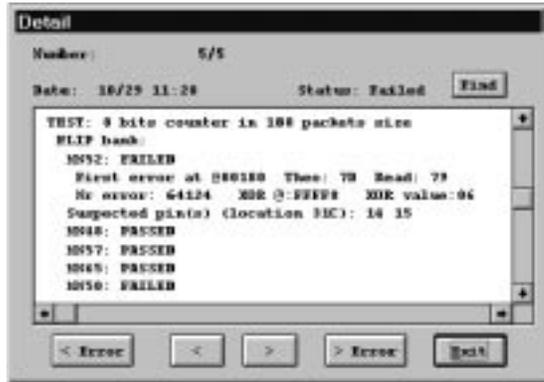
Figure 6–21: EISA failure
