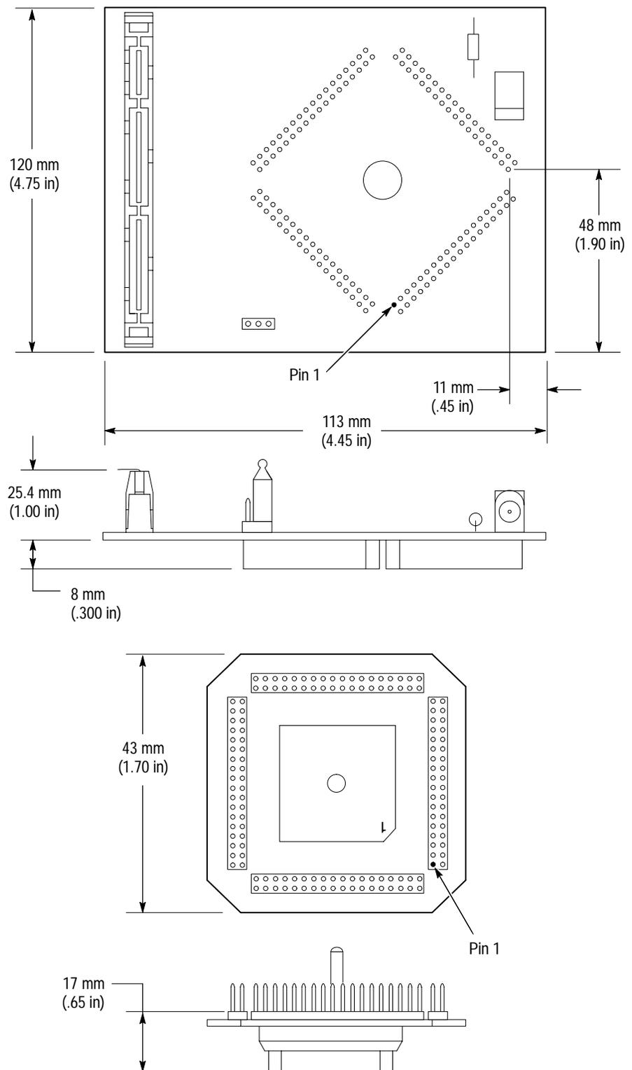
Figure 3-2: Dimensions of the probe adapter
