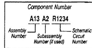
Chassis mounted components have no Assembly Number prefix - see end of Replaceable Parts List.
