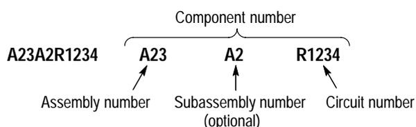
**Read: Resistor 1234 (of Subassembly 2) of Assembly 23**
