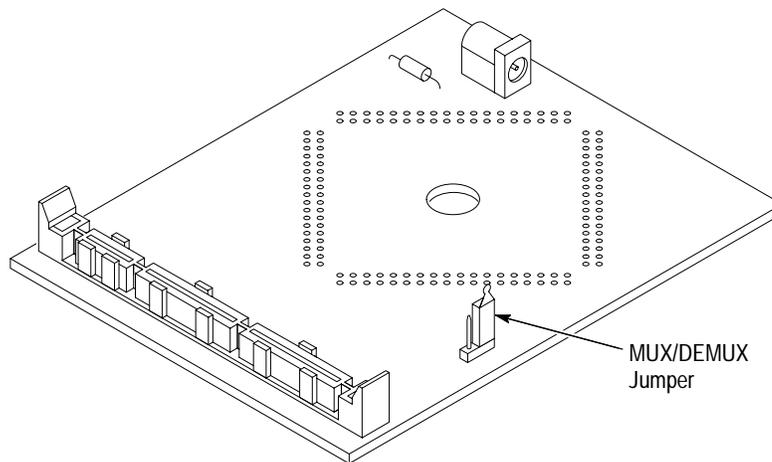
Figure 3–1: Jumper locations on the probe adapter
