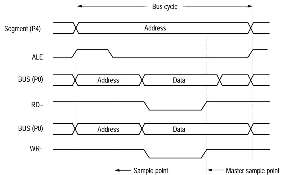
Figure 3–3: 80C167 multiplexed bus timing
