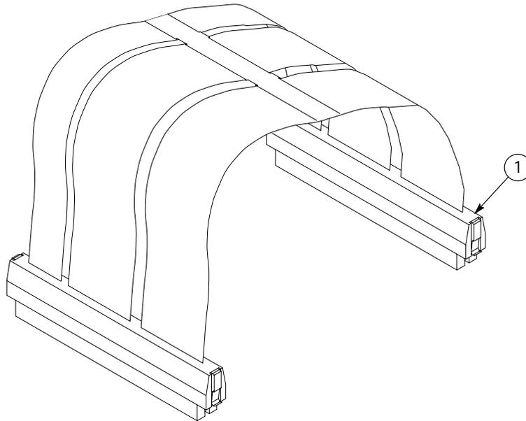
**Figure 2: High density probe cable**
