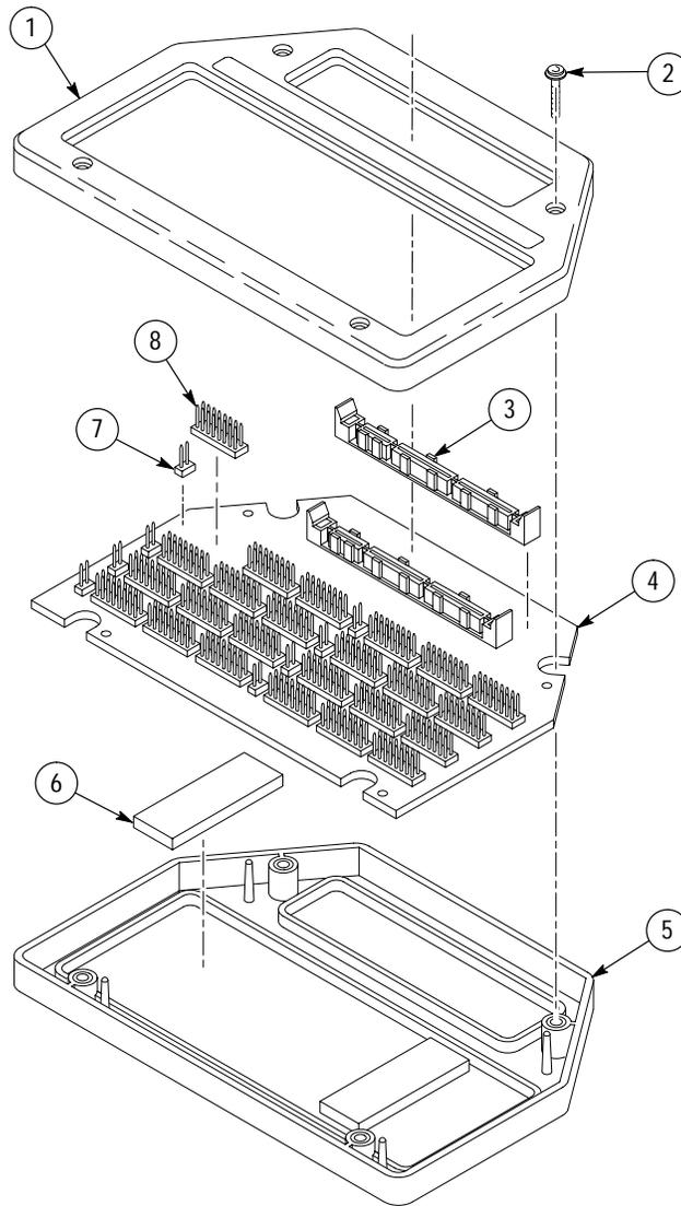
Figure 3: 192-Channel High-Density Probe exploded view
