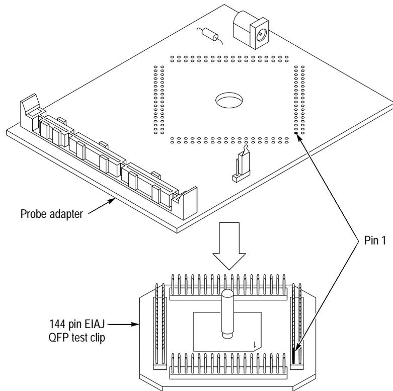
**Figure 1–2: Attaching the PQFP clip to the probe adapter.**
