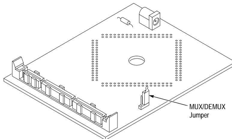
Figure 1–1: Jumper locations on the probe adapter
