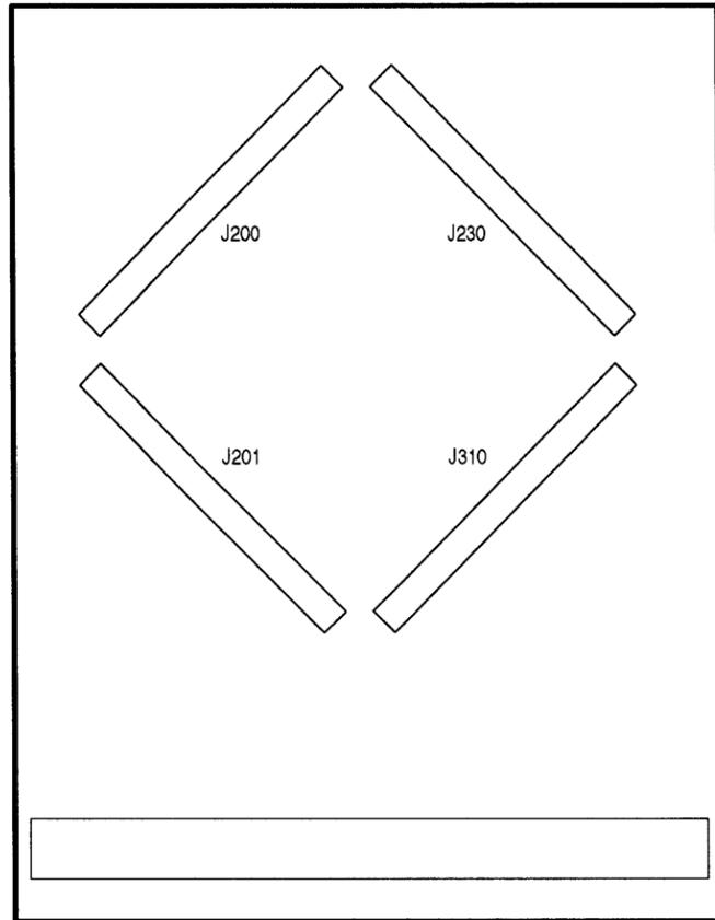
A01 SAB-C167 probe adapter board component locations
