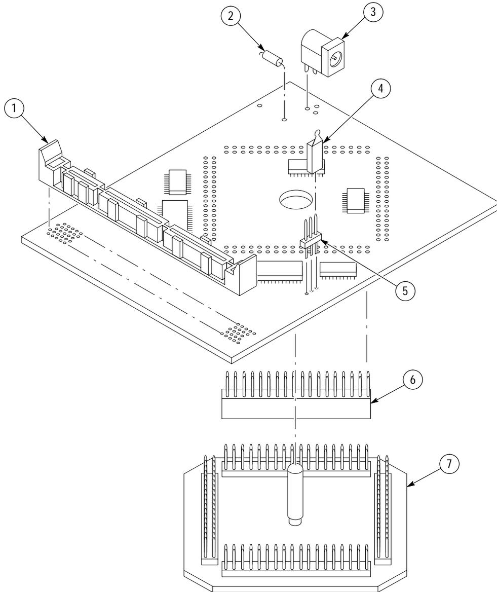
Figure 1: 80C167 probe adapter exploded view
