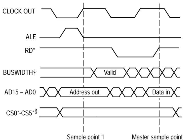
†For the 8XC196NT microcontroller, the BUSWIDTH signals are latched on the falling edge of the CLOCKOUT signal immediately after the falling edge of the ALE signal.
