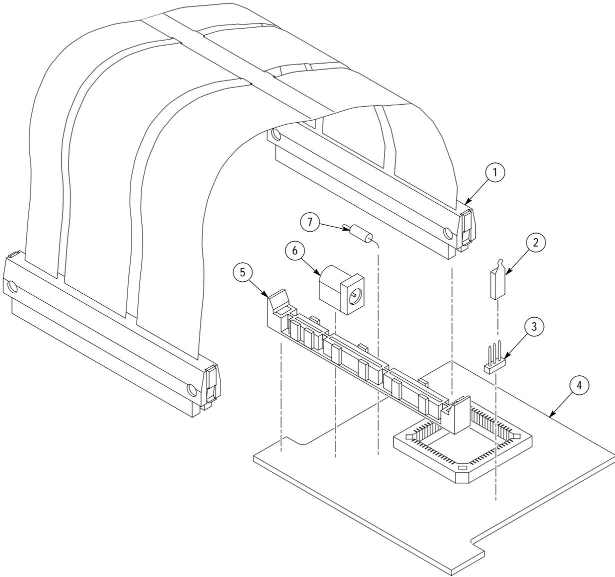
Figure 1: 8XC196NT probe adapter exploded view
