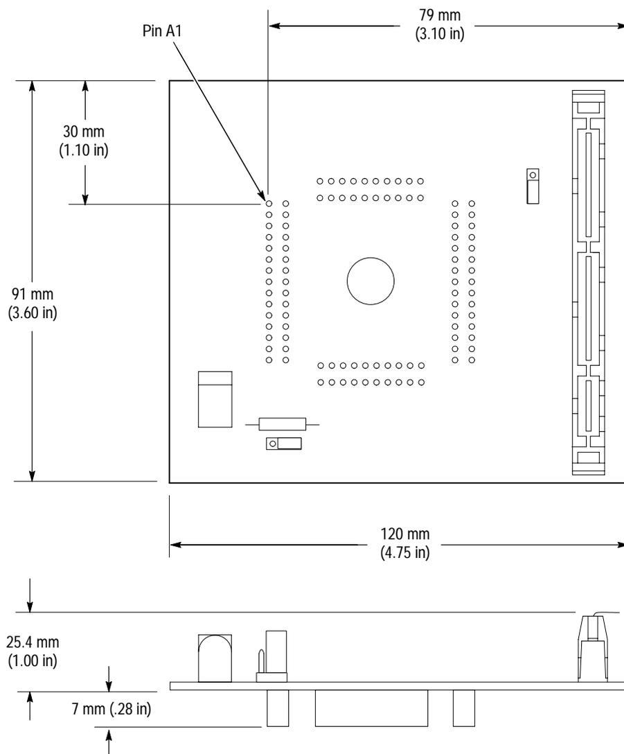
Figure 3–2: Dimensions of the 8XC196NP probe adapter
