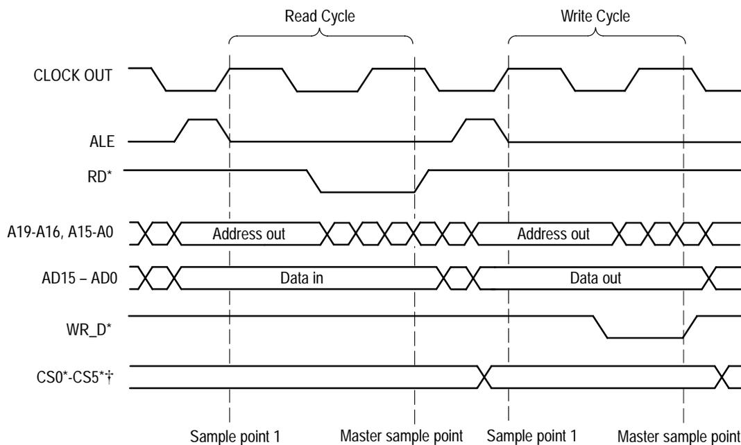
**Figure 3-5: Demultiplexed bus timing for the 8XC196NP microcontroller only**
