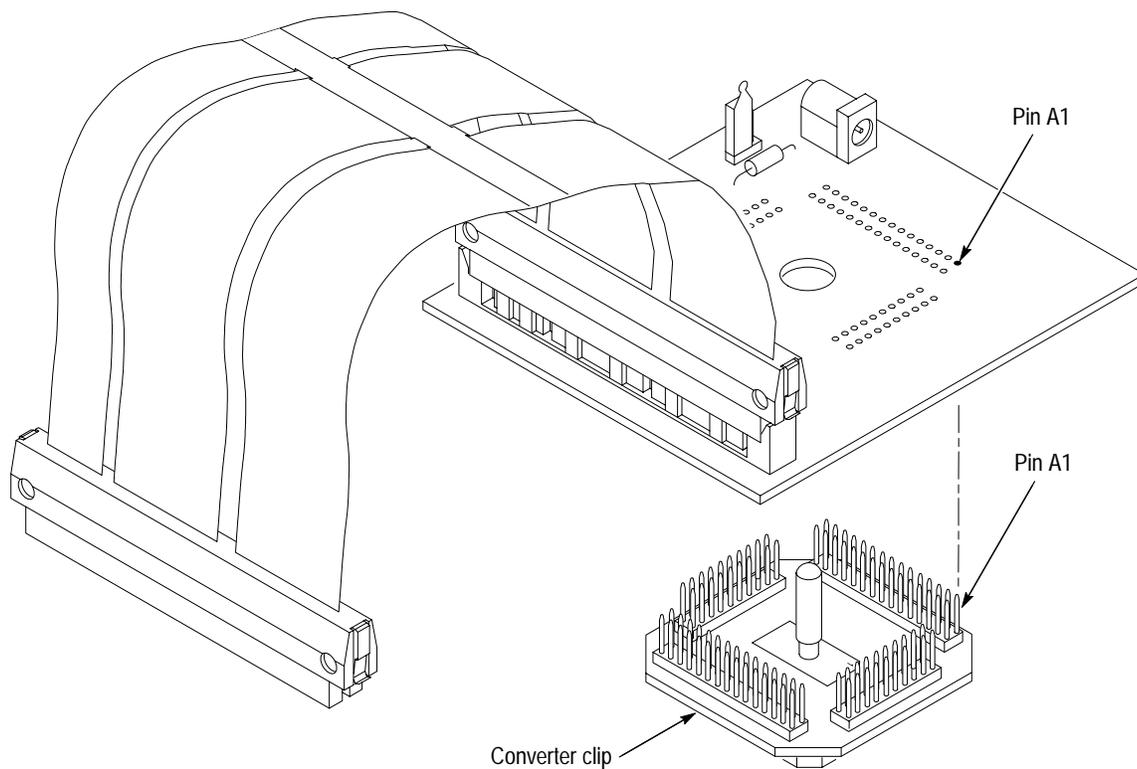
**Figure 1-6: Placing the converter clip onto the probe adapter**
