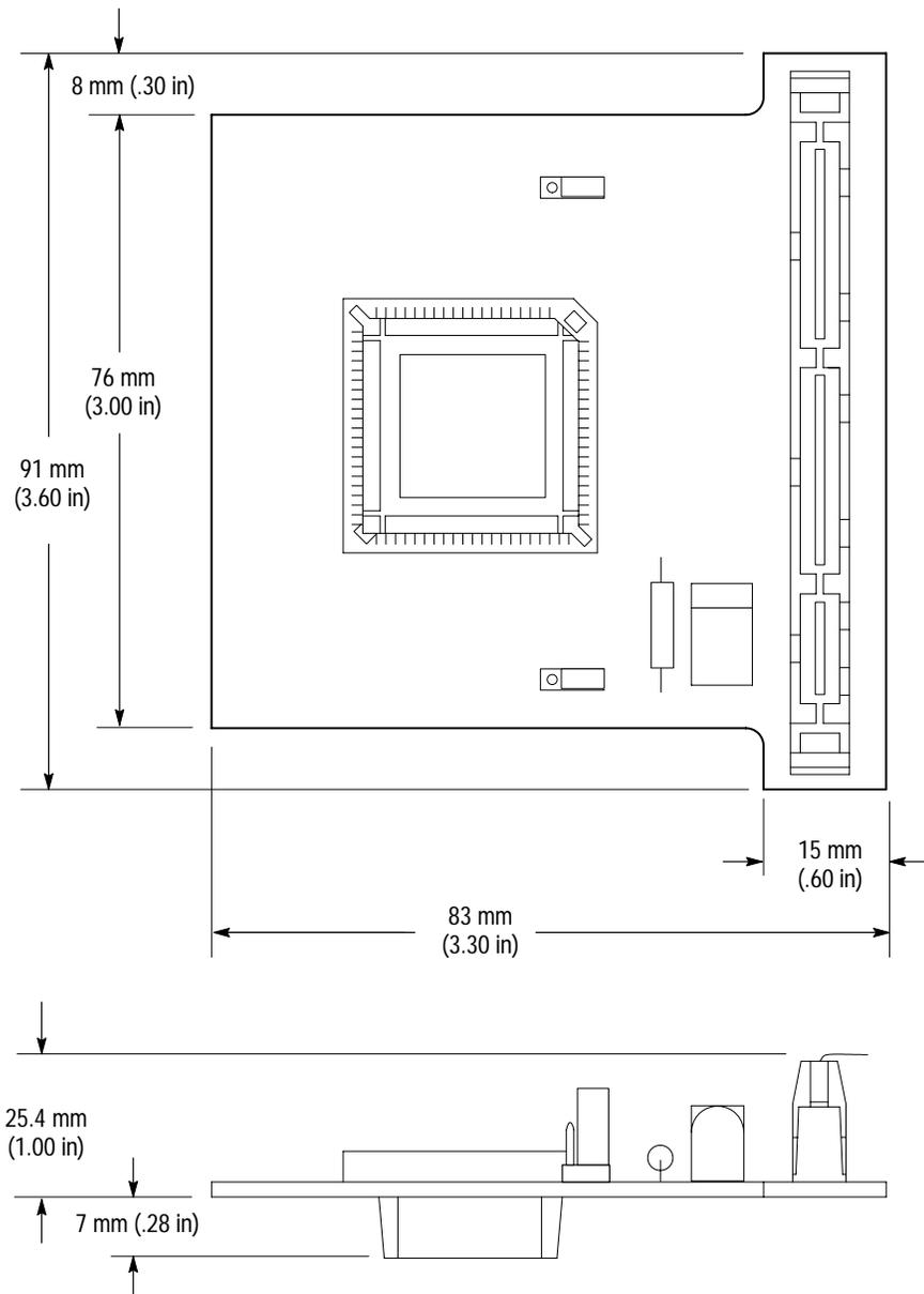
Figure 3–3: Dimensions of the 8XC196NT probe adapter
