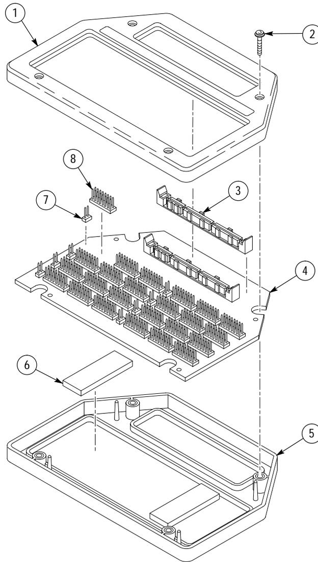
Figure 3: 192-Channel High-Density Probe exploded view
