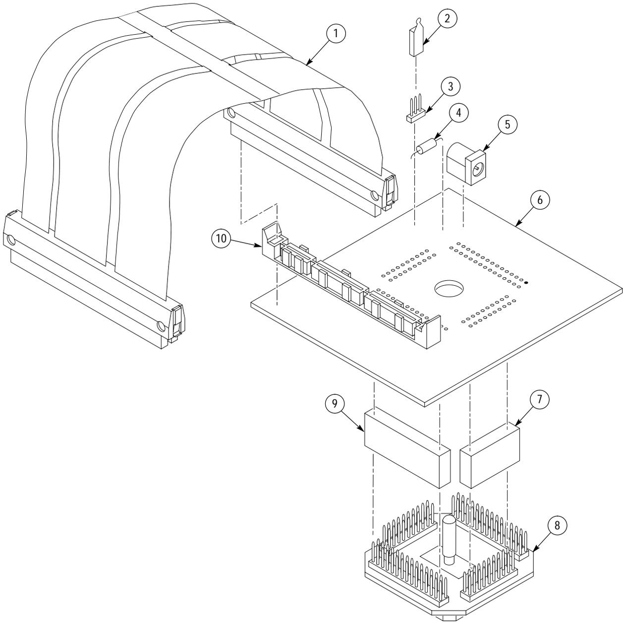
Figure 2: 8XC196NP probe adapter exploded view
