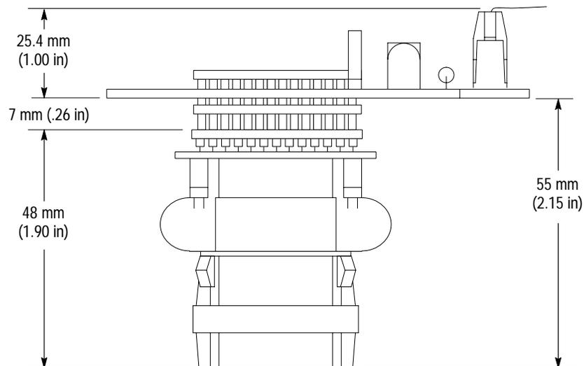
**Figure 3–3: Dimensions of the PGA-to-QFP converter clip**
