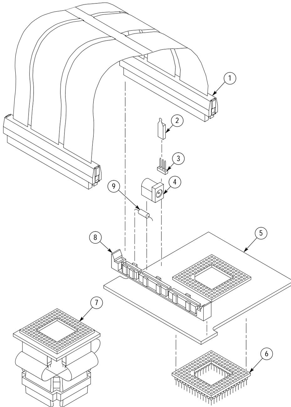
Figure 1: i960 Jx probe adapter exploded view
