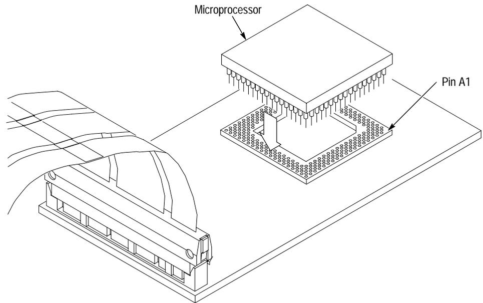
**Figure 1-2: Placing a microprocessor into the probe adapter**
