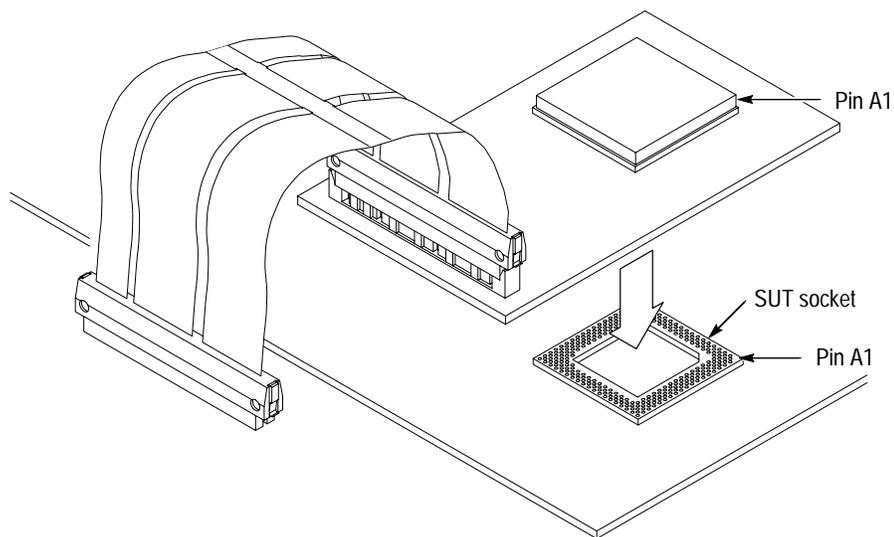
**Figure 1-3: Placing a PGA probe adapter onto the SUT**
