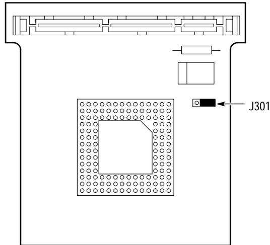
Figure 3–1: Jumper location on the probe adapter
