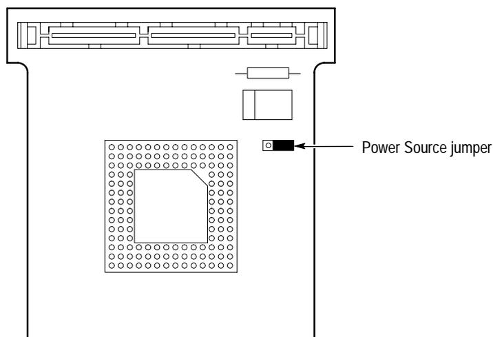
Figure 1–1: Power Source jumper location
