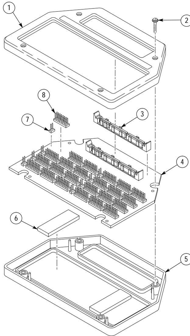
Figure 2: 192-Channel High-Density Probe exploded view
