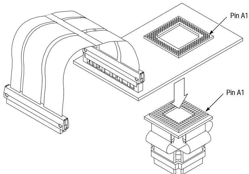
**Figure 1-6: Placing the converter clip onto the probe adapter**
