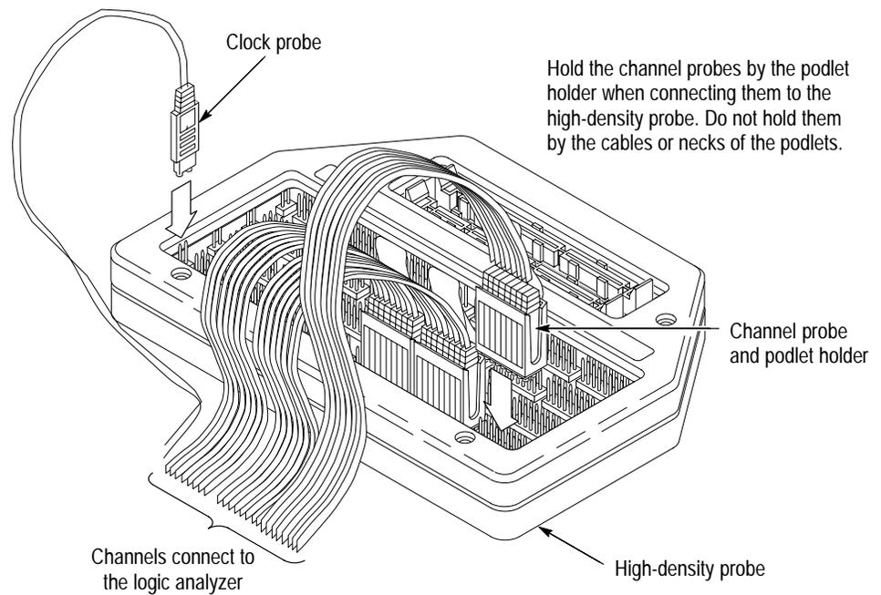
**Figure 1-4: Connecting channel and clock probes to a high-density probe**
