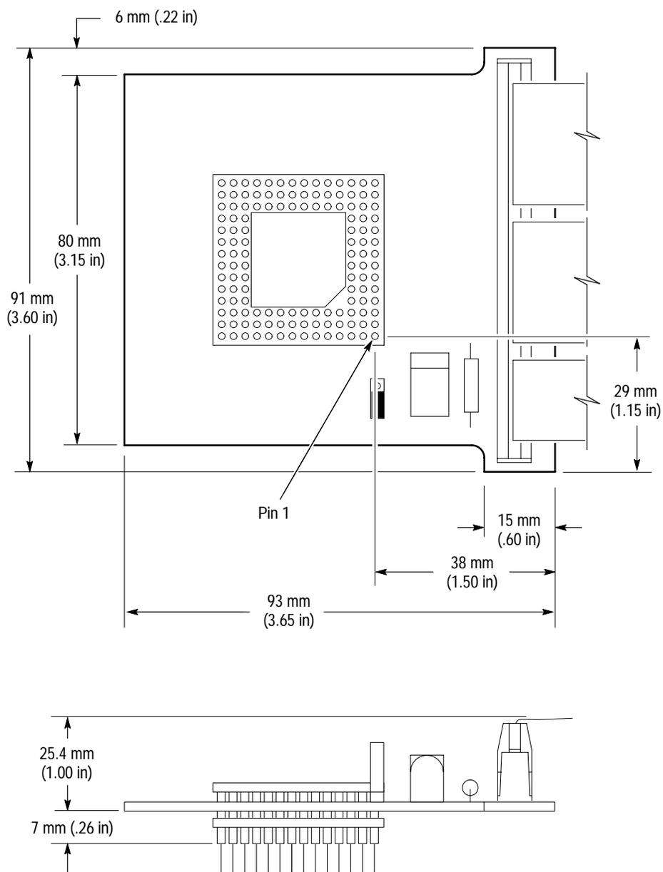
Figure 3–2: Dimensions of the probe adapter
