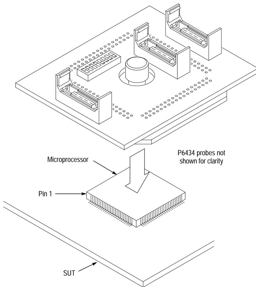
**Figure 1-3: Placing the probe adapter onto the SUT**
