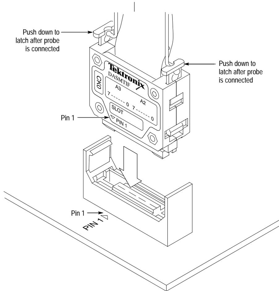
**Figure 1-1: Connecting P6434 probes to the probe adapter**
