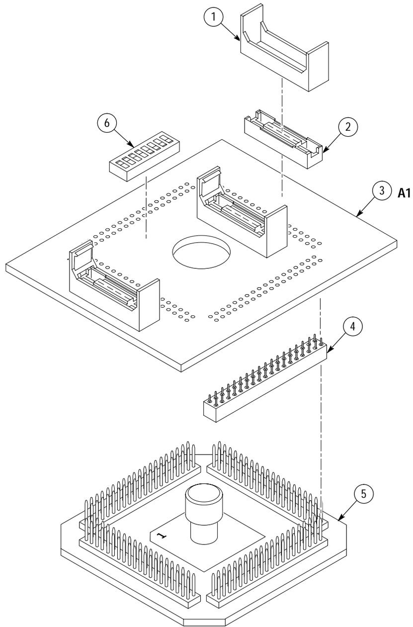
Figure 1: PowerPC MPC505 probe adapter exploded view
