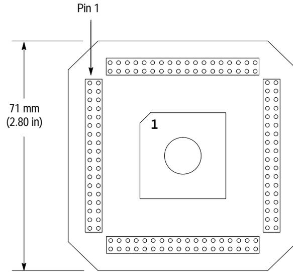
**Figure 3-2: Dimensions of the test clip**
