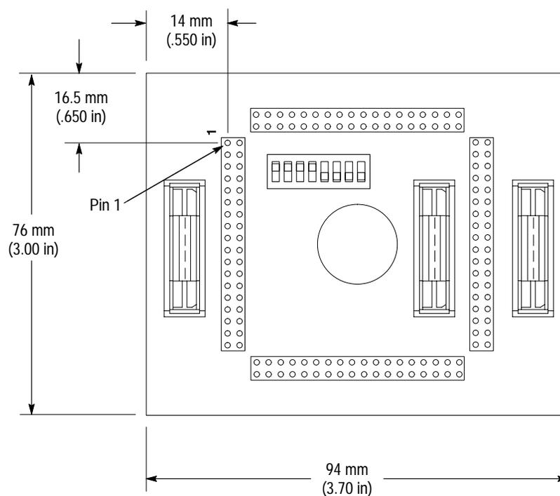
**Figure 3-1: Dimensions of the probe adapter**
