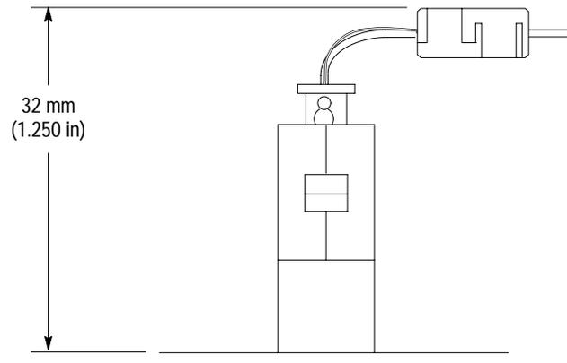
**Figure 3-4: Height of the P6434 probe after connected to the probe adapter**
