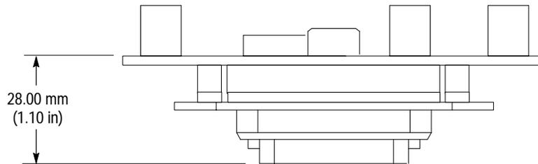
**Figure 3-3: Vertical height of the probe adapter and test clip**
