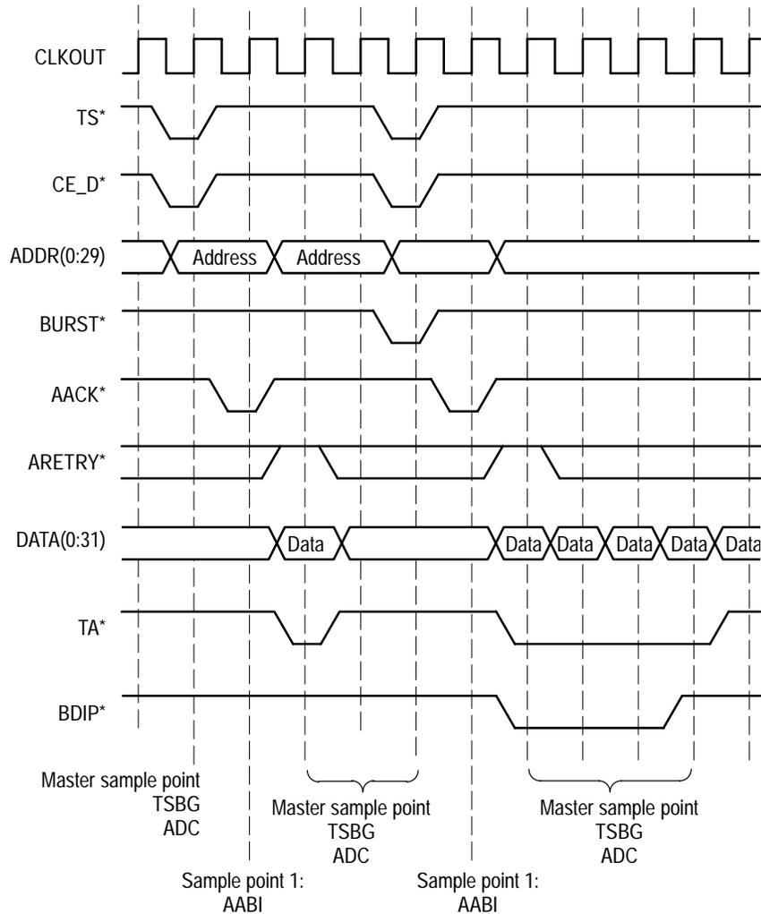
Figure 2-2: PowerPC MPC505 bus timing non-pipelined
