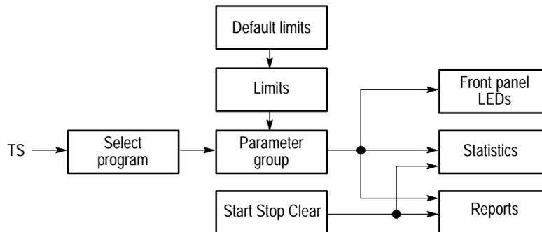
**Figure 4–13: Functions of MONITORING menu**
