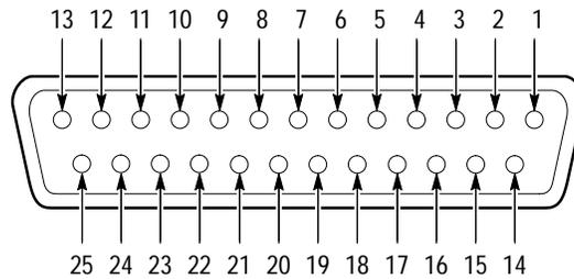
**Table A-1: Pin assignment of TS PARALLEL connector (corresponding to DVB Document A010)**
