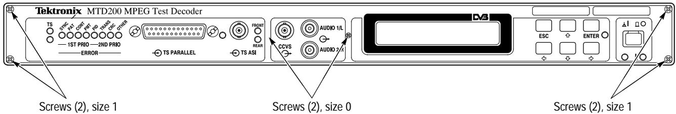
Figure 6-2: Front-panel screws
