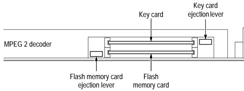
**Figure 3-1: Slot for key card**
