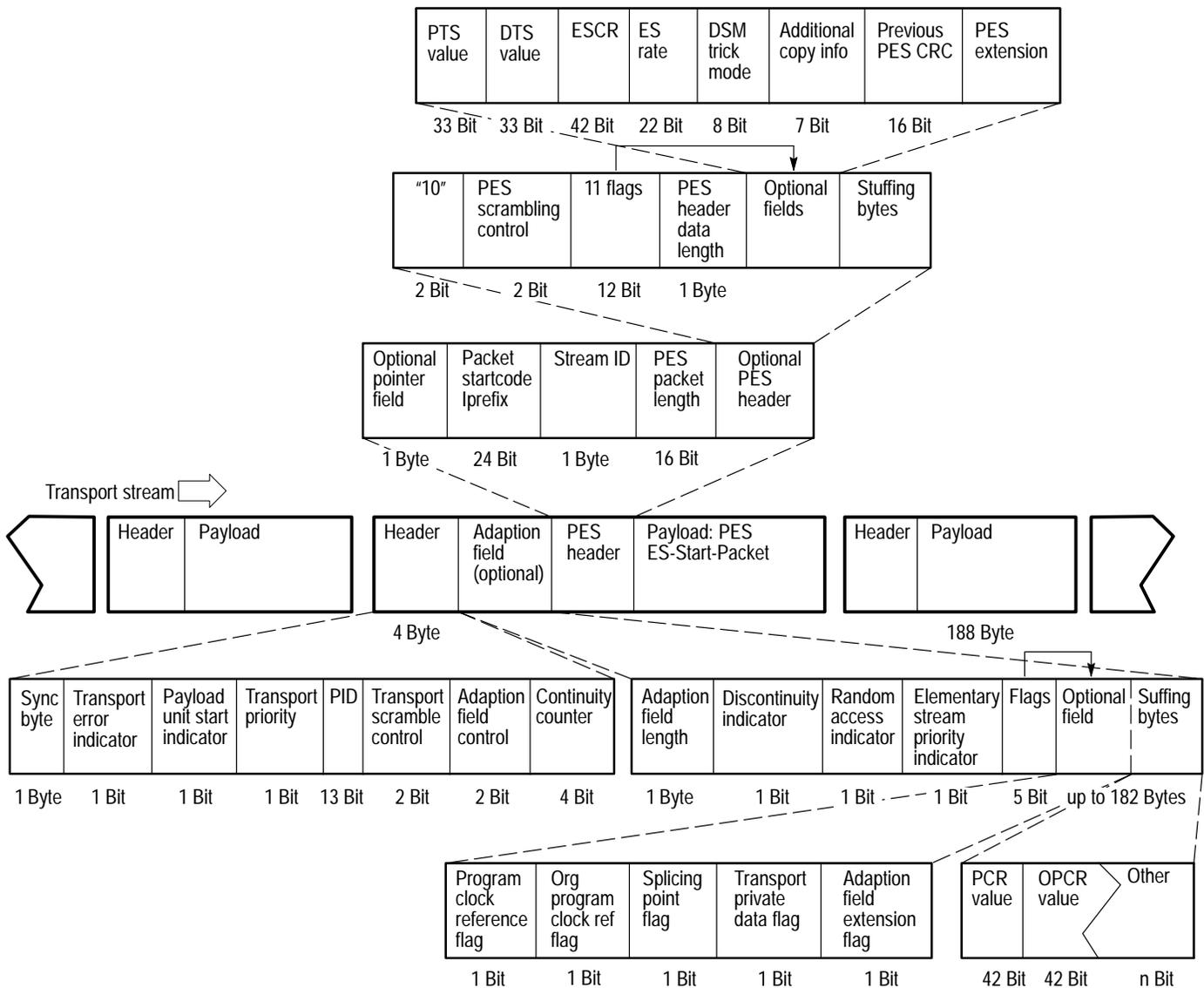
Figure 2–1: Elements of the transport stream syntax
