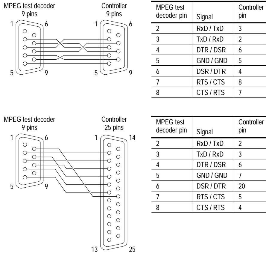
Figure A-2: Wiring diagram for hardware handshake
