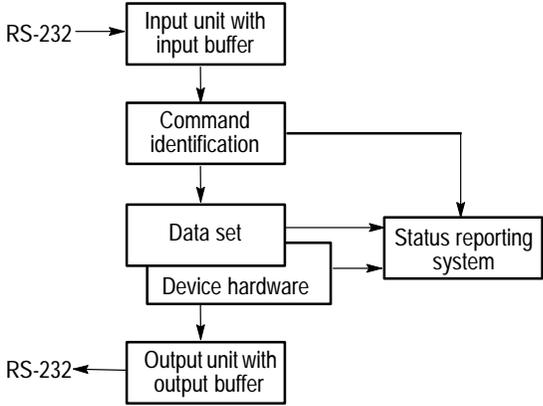
Figure 5–2: Instrument model with remote control via RS-232 interface
