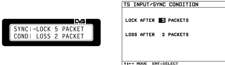
**Figure 4-31: TS INPUT/SYNC CONDITION menu**
