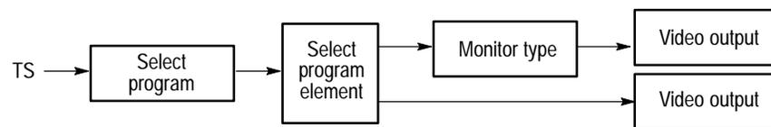
**Figure 4–23: Interaction of DECODER functions**
