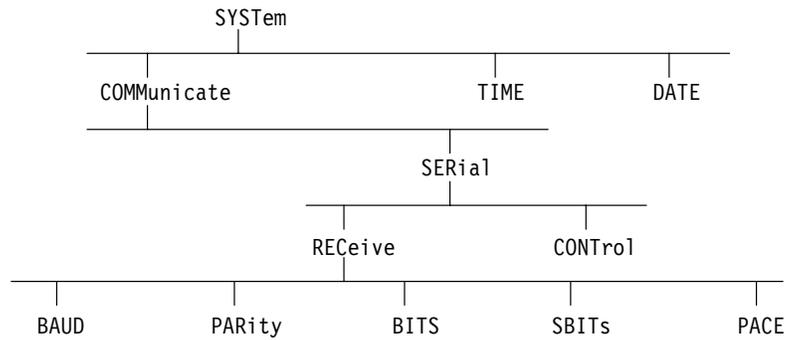
**Figure 5-1: Tree structure of SCPI command systems (SYSTEM shown as an example)**
