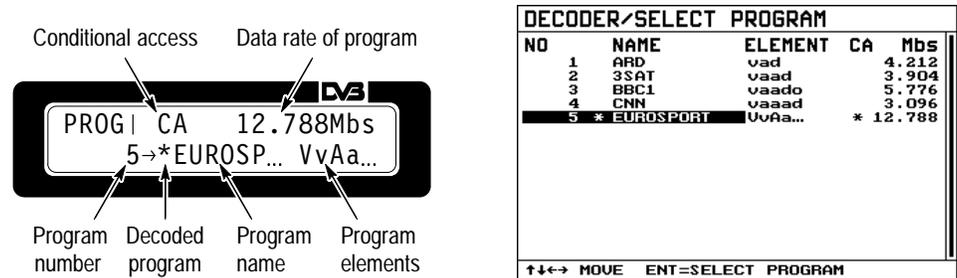
**Figure 4–24: DECODER/SELECT PROGRAM menu: Selecting a program via its name**
