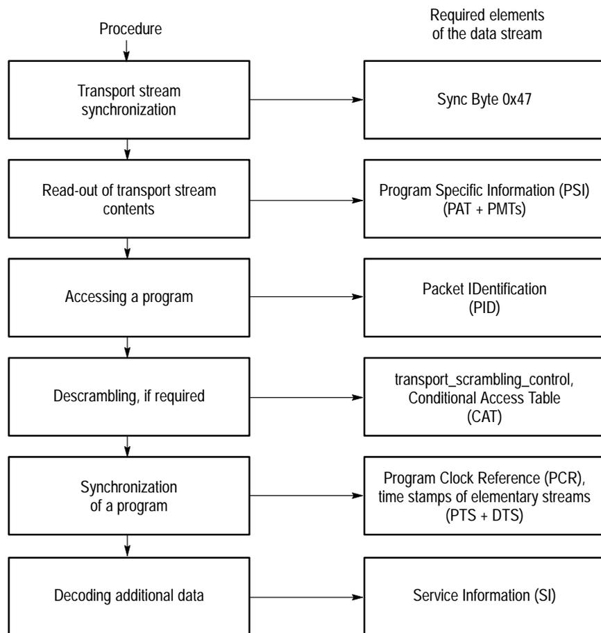
Figure 1–2: Functions of a transport stream demultiplexer
