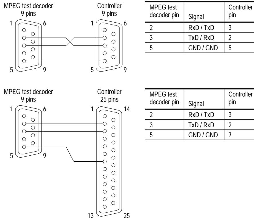
**Figure A-1: Wiring Diagram for software handshake**
