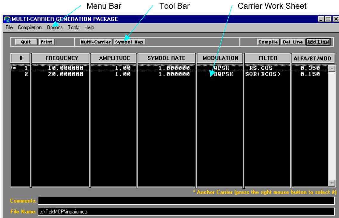
Waveforms are defined by adding all the required carriers to the project. The main window provides access to all the edition and configuration functions. It is composed by:
