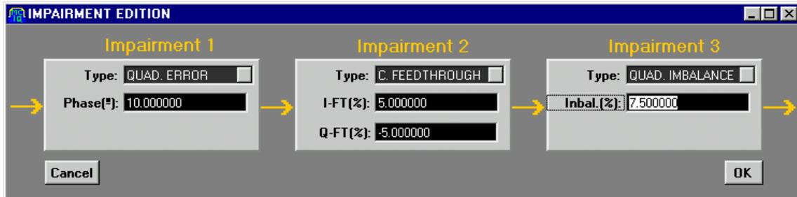
Three blocks are accessible to the user. Each block can add an impairment process to the calculation chain. The following impairment types and parameters can be used in each block:
