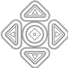
In the lower right area of the front panel is a five-button group (up-down-left-right-center). The arrow buttons serve the functions of moving the cursor left and right across the displayed waveform or changing values (◀▶), scrolling through a menu or changing values (▲▼), and scrolling pages (◆ + ▲▼).
