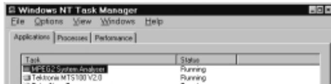
**Figure B-1:** Select the locked application in the Task Manager window
