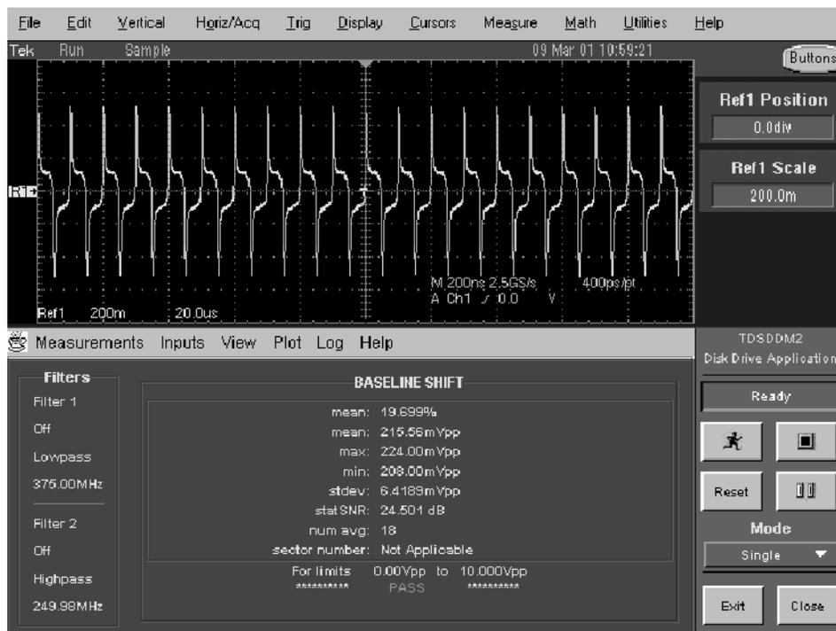
Figure 2-38: Baseline Shift measurement results example
