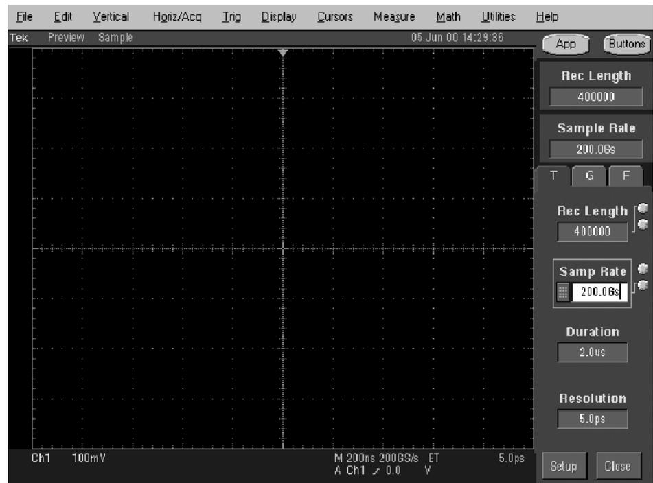
Figure 1-6: Spectral Control T tab for a TDS7104 oscilloscope
