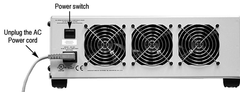
**Figure 4-15: Power switch and AC power cord locations**
