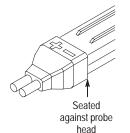
CAUTION. To avoid damaging the square pin connectors, do not insert anything larger than a 0.025-inch square pin into the inputs.
