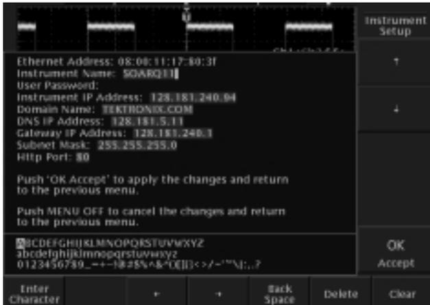
Figure 1. TDS3000B IP address menu. From your oscilloscope's front panel, then select menu options in this order: Utility, System, I/O, Ethernet Network Settings, Change Instrument Settings.
