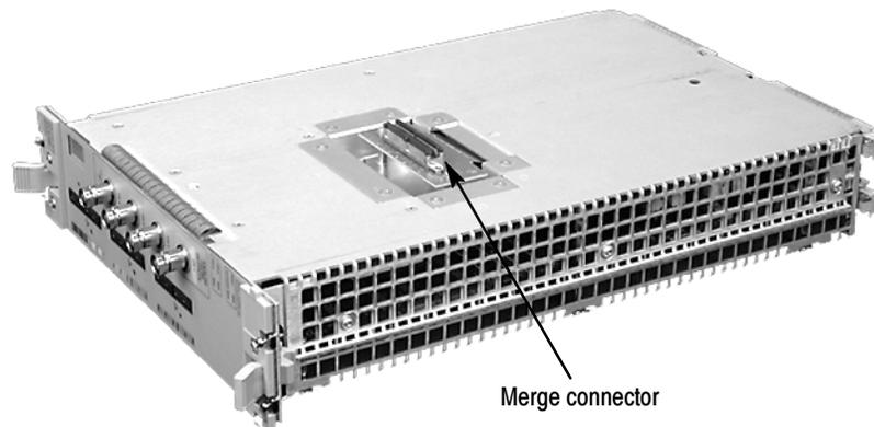
**Figure 2-6: Merge connector (shown in the extended position)**
