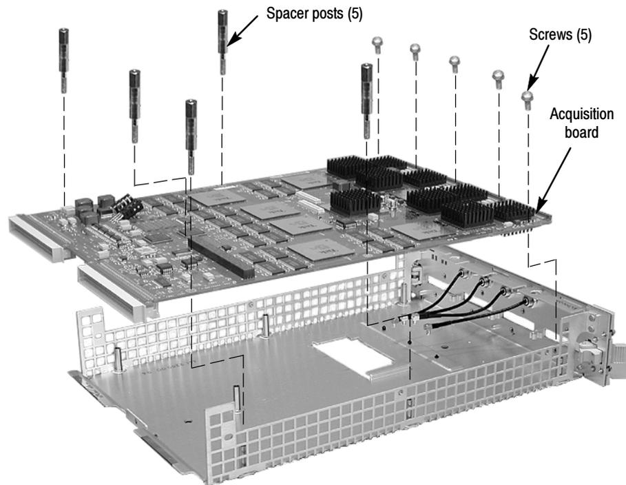
**Figure 6-12: Removing the acquisition board from the chassis**
