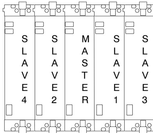
**Figure 2-8: Location of modules in a merged system**
