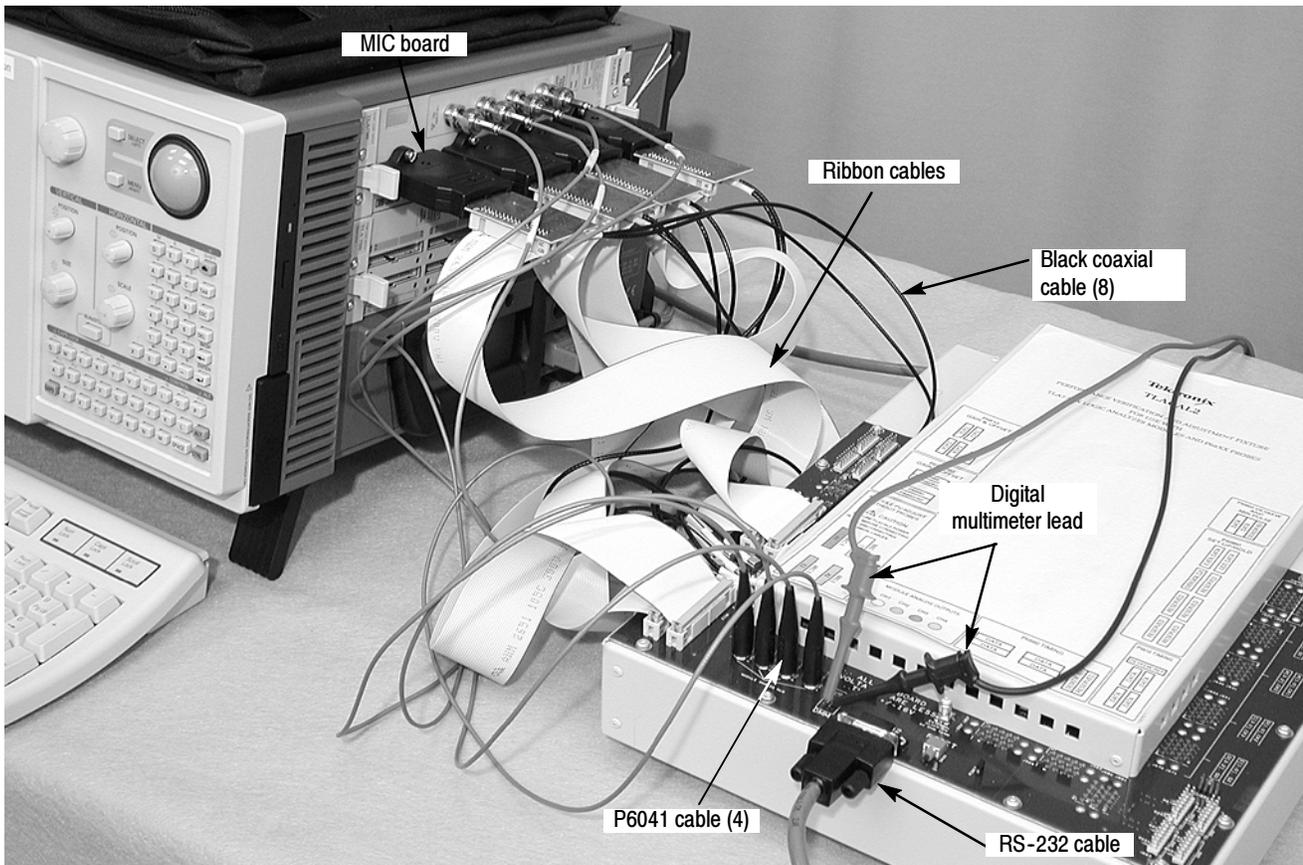
Figure 2-4: TLACAL2 performance verification and adjustment test fixture
