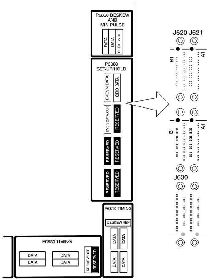
**Figure 4- 6: P6860 Setup & Hold procedure connections**
