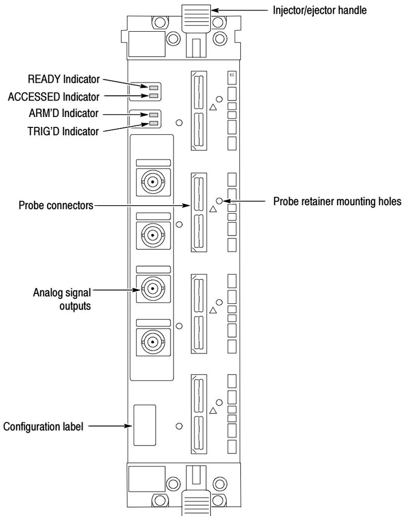
**Figure 2-5: Front panel of the logic analyzer module**
