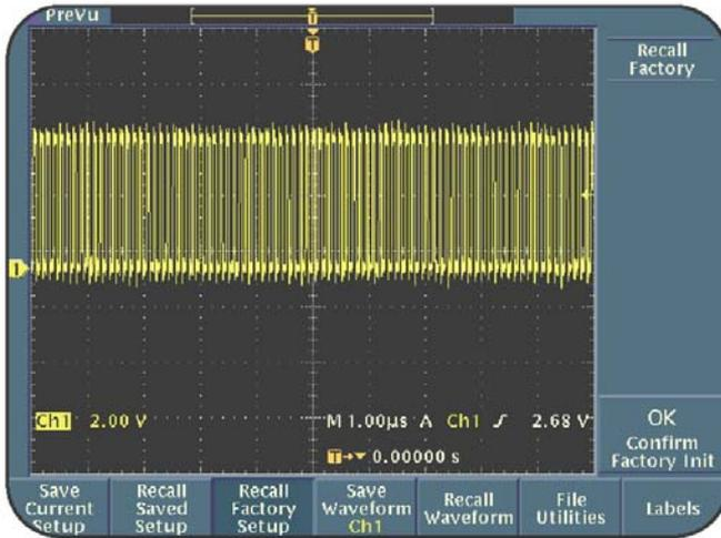
**Figure 6.11: Clock signal in vector form**
