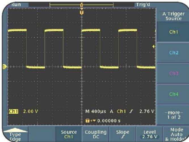
*Figure 1.9: TRIGGER Section menu-based controls*
