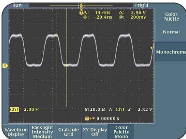
**Figure 6.10: Monochrome display mode**
