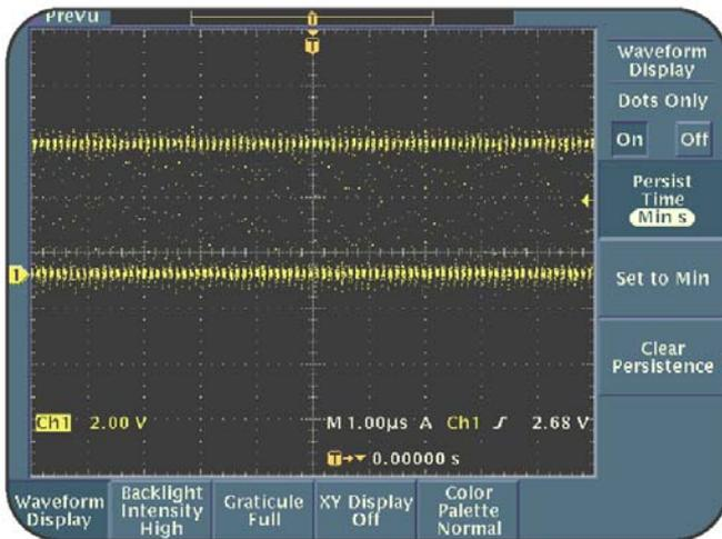
**Figure 6.12: Clock signal with Dots Only On**
