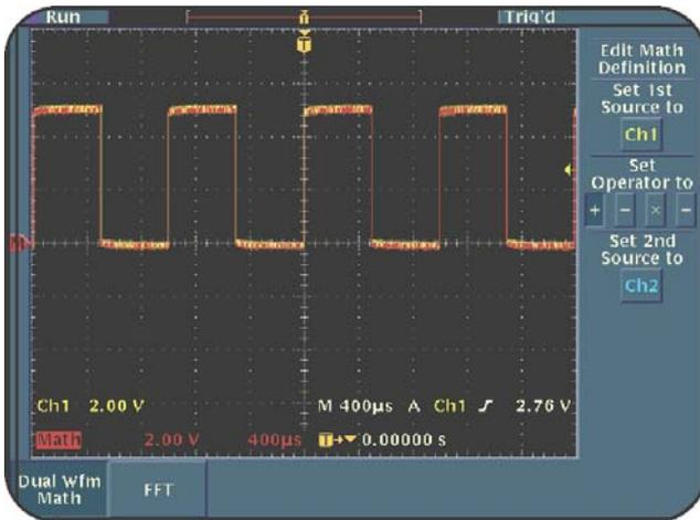
**Figure 1.5: TDS3000 oscilloscope MATH menu-based controls**
