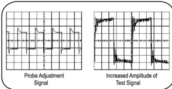
**Figure 1.21: Overcompensated probe**
