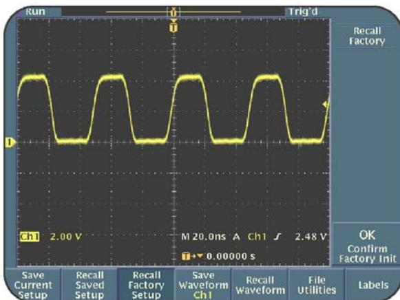
**Figure 6.2: 20 MHz CLOCK signal**
