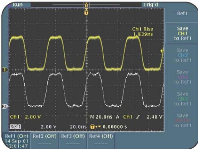
**Figure 6.7: Recalled reference waveform**
