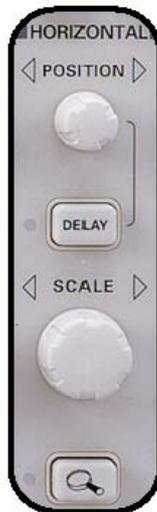
**Figure 1.6: TDS3000 HORIZONTAL section controls**
