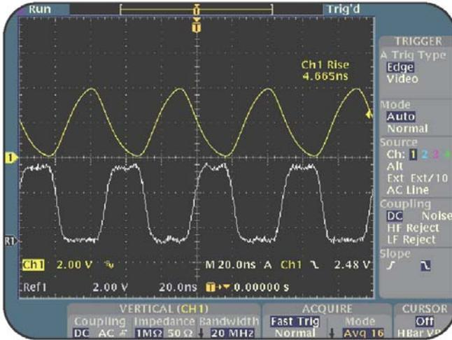
**Figure 6.8: QUICKMENU display**
