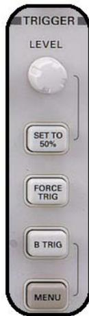
*Figure 1.7: TDS3000 TRIGGER section controls*
