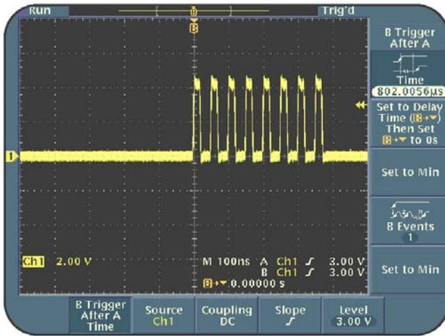
**Figure 3.7: B TRIG enabled after a delay of about 800us**
