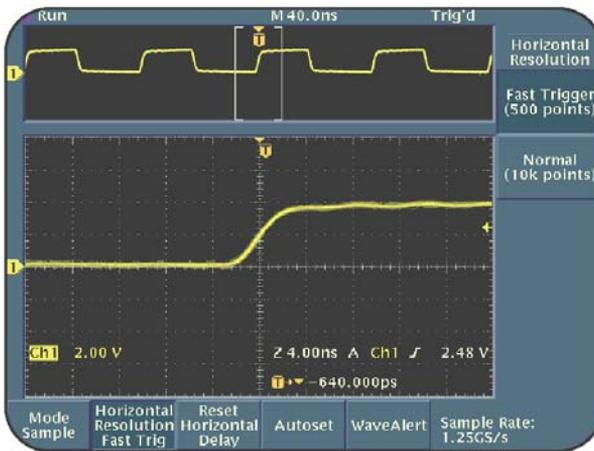
**Figure 3.5: Magnified display with Fast Trigger (500 points) mode**
