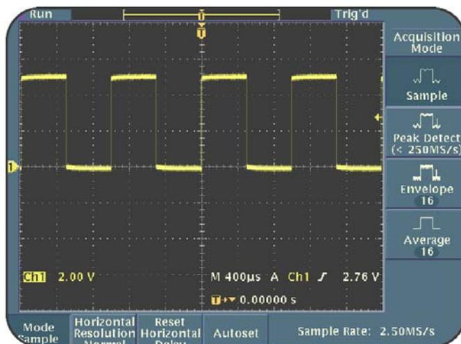
**Figure 1.11: Menu-based functions for the ACQUIRE section**
