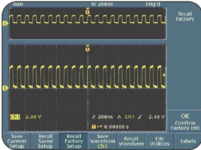
**Figure 3.3: Zoom mode waveform display**
