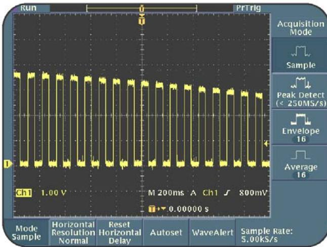
**Figure 5.2: Noisy variable amplitude signal**
