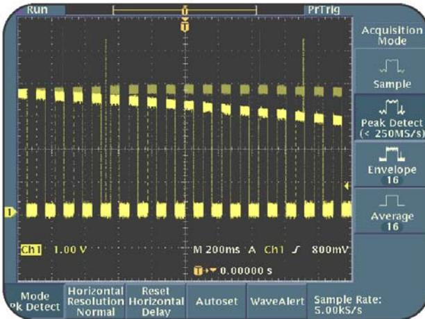
**Figure 5.4: Noisy variable amplitude signal with glitches, captured with Peak Detect mode in an intensity graded display**
