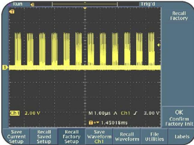
**Figure 3.6: Unstable overlapping waveforms**
