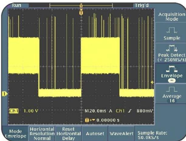
**Figure 5.6: Accumulated peak-detected waveforms with the Envelope acquisition mode**
