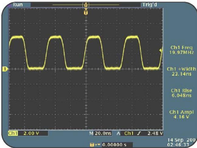
**Figure 6.3: Automatic measurements**
