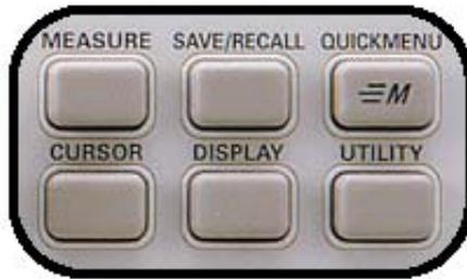
*Figure 6.1: TDS3000 front panel menu function controls*
