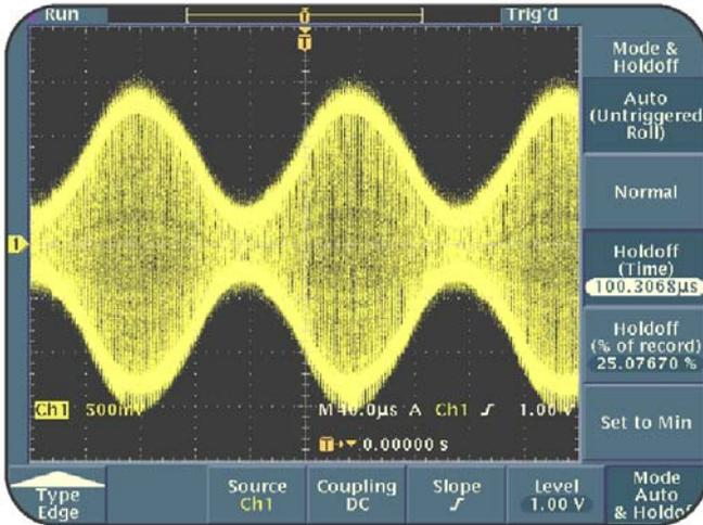
**Figure 4.5: AM signal, with trigger holdoff**
