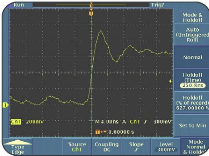
**Figure 5.7: Step response waveform with ground lead**
