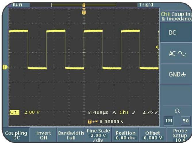
**Figure 1.4: VERTICAL menu-based options for CH1**
