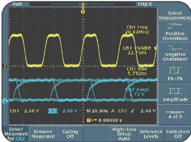
**Figure 6.4: Simultaneous amplitude measurement of CH1 and CH2**
