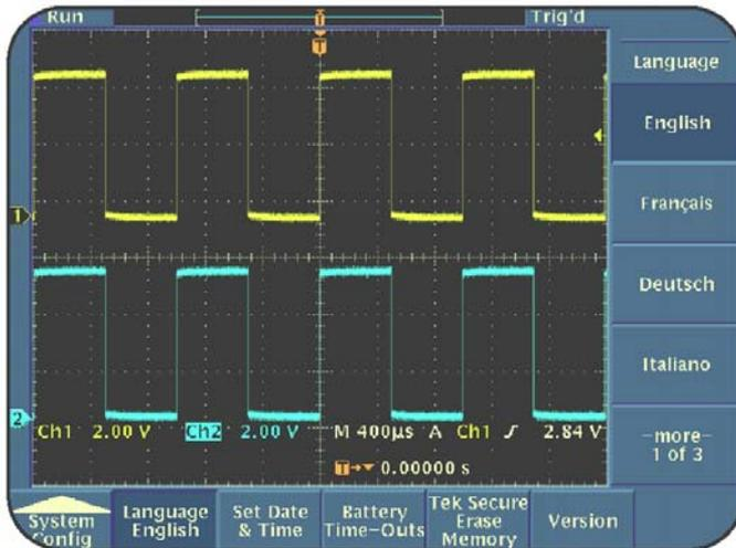
**Figure 1.19: CH1 Probe Compensation Signal**
