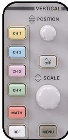
**Figure 1.3: TDS3000 VERTICAL section controls**
