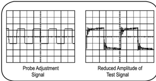
**Figure 1.20: Undercompensated probe**
