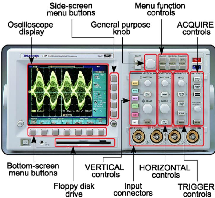
Figure 1.1: A TDS3054 digital phosphor oscilloscope
