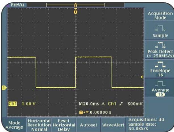
**Figure 5.5: Reduced signal noise with the Average acquisition mode**
