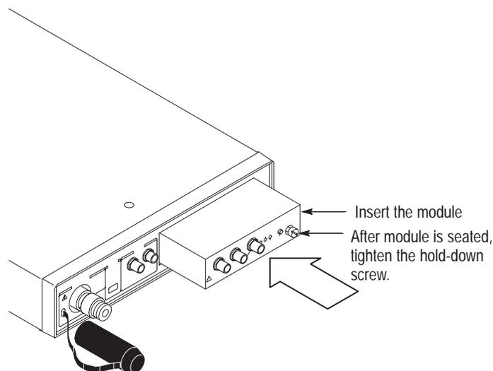
Figure 7: Installing a Clock Recovery Module
