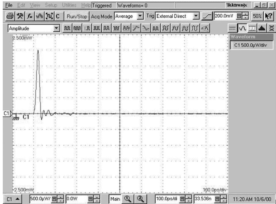
Figure 15: Proper positioning of the impulse for optimum curve download
