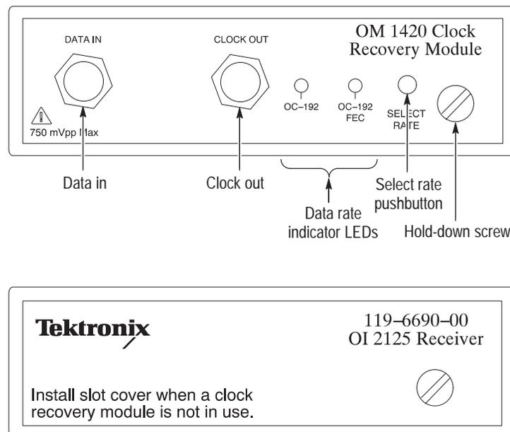
Figure 6: Clock Recovery Modules for the receiver
