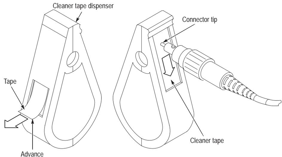
**Figure 20: Cleaning an optical connector**
