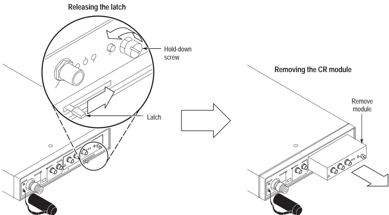
Figure 8: Releasing the module with the latch
