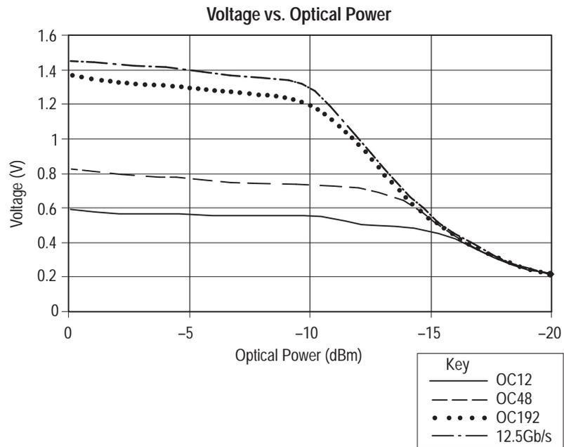
Figure 11: OI2125 Output Voltage versus Input Optical Power
