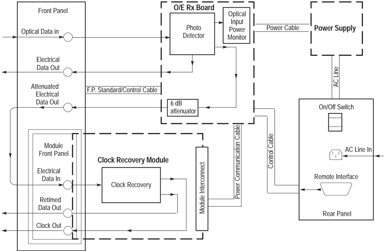
Figure 12: O/E Receiver interconnect diagram
