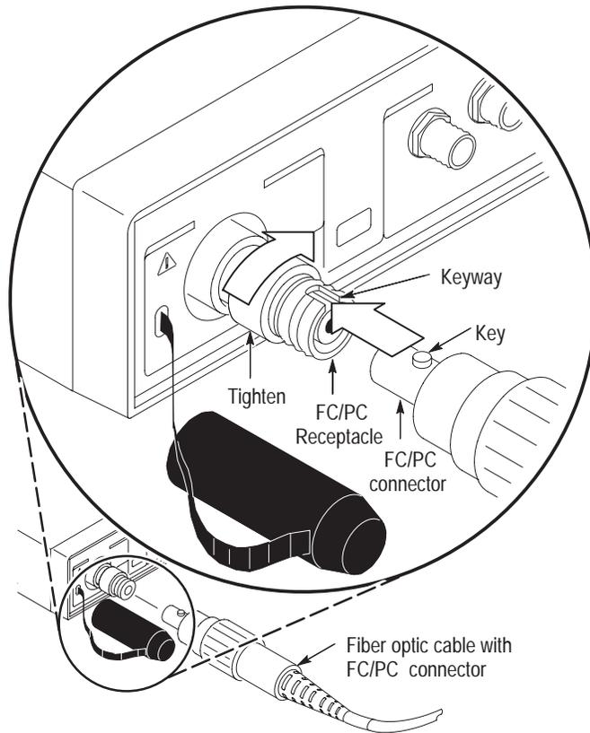
Figure 4: Connecting a fiber optic cable
