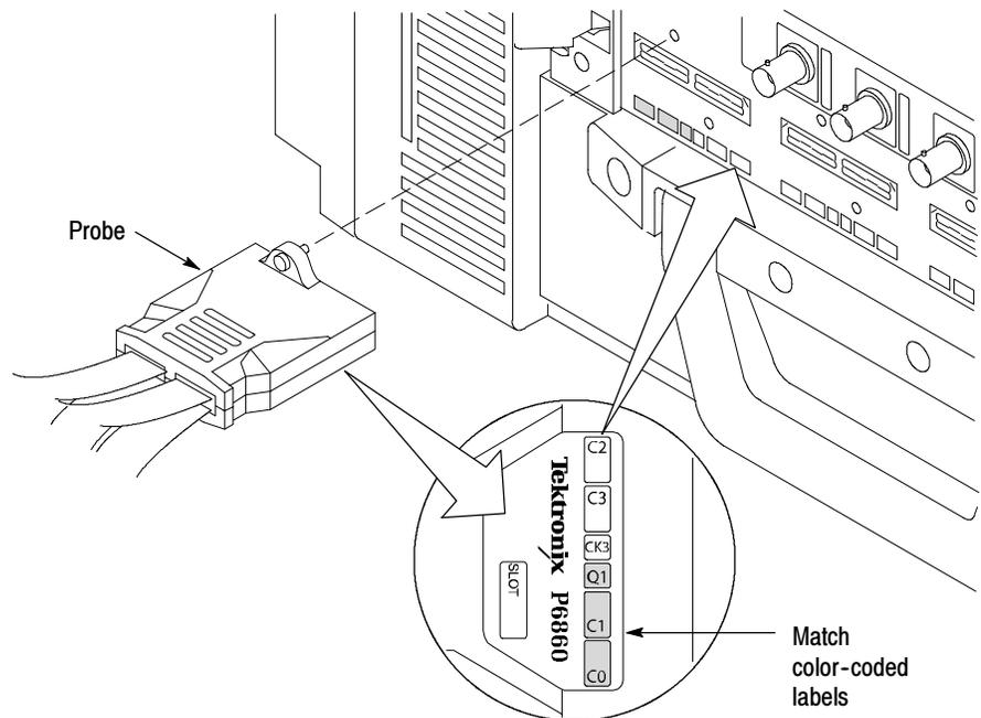
**Figure 1-9: Connecting the probes to the logic analyzer**
