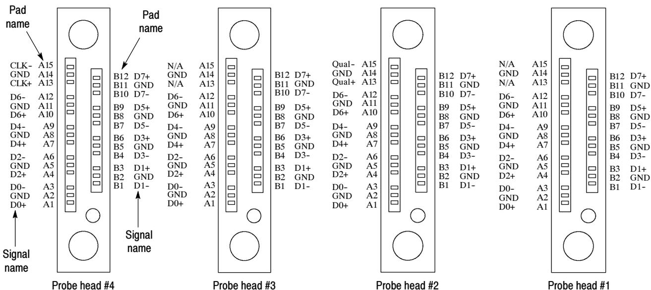
Figure 2- 5: P6880 Differential probe land footprint
