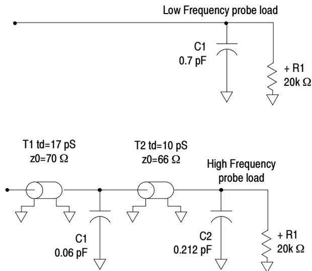
**Figure 2-17: High-Density and High-Density Differential probe load model**
