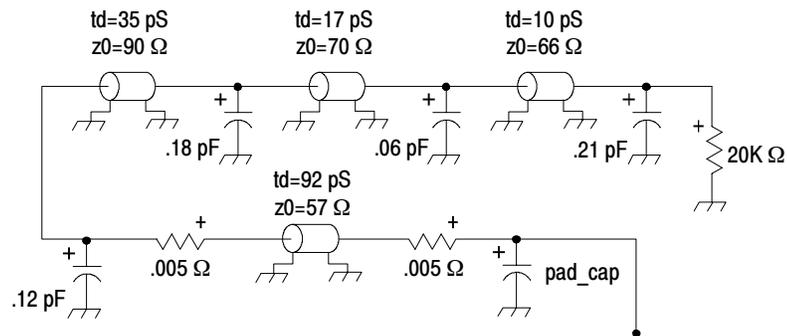
**Figure 2-18: Mictor-on-PCB to Compression adapter load model**
