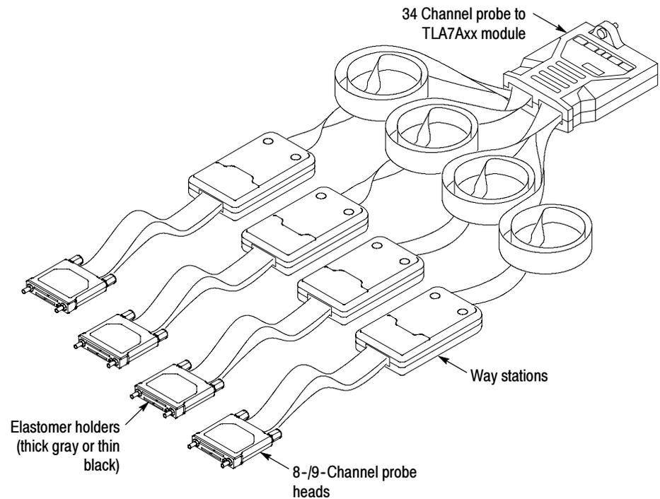
**Figure 1-5: P6880 High-Density Differential probe**
