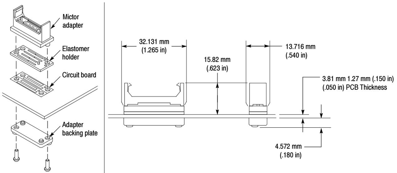
**Figure 1-7: 34-Channel Compression-on-PCB to P6434 Mictor adapter**
