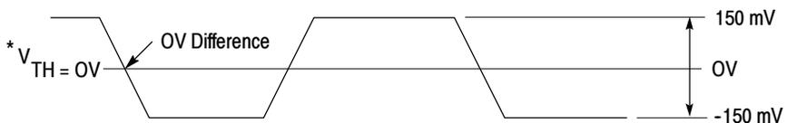
\* Note: For differential inputs, the module threshold should be set to OV (assuming no common mode error).
