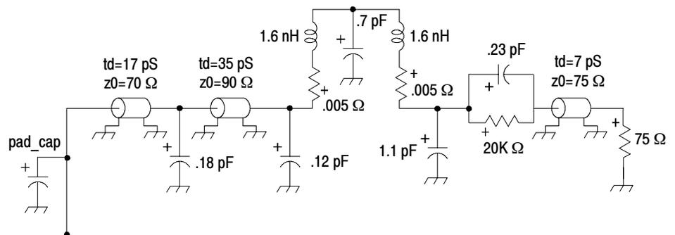
**Figure 2-19: Compression-on-PCB to P6434 Mictor adapter load model**
