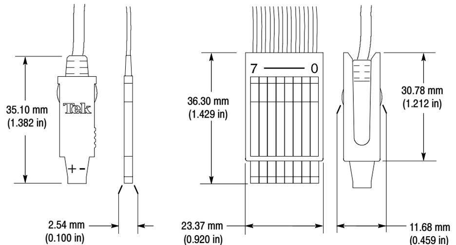
**Figure 2-10: Physical attachment requirements for the P6810 probe**
