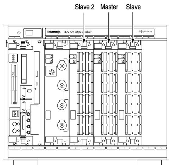
**Figure 1-1: Configuration of the slave 2, master, and slave modules**
