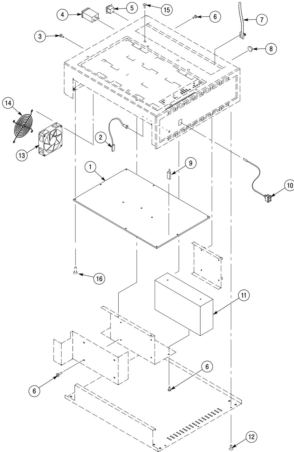
Figure 6-3: Preprocessor unit exploded view
