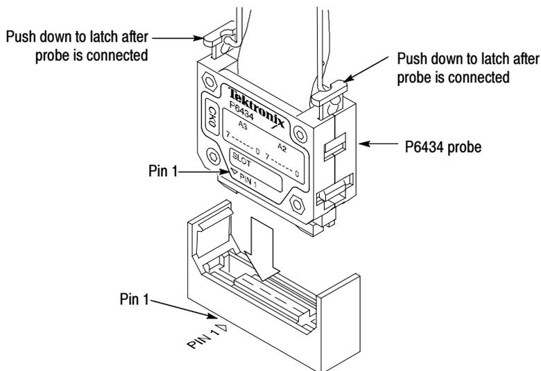
**Figure 1-12: Operating the P6434 probe latches**
