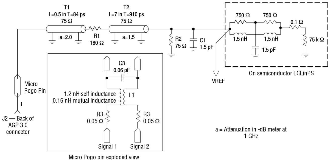
**Figure 4-3: Backside source sync load model**
