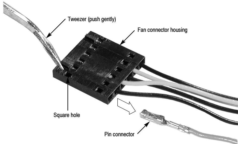
**Figure 5-4: Removing the fan pin connector**
