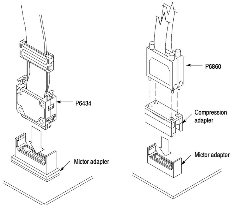
**Figure 1-13: Probes with mictor adapters**
