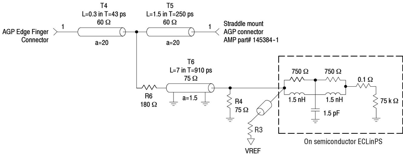
**Figure 4-2: Interposer source sync load model**
