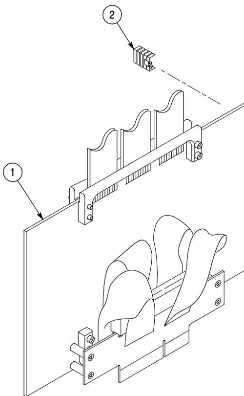
**Figure 6-1: Interposer probe head exploded view**
