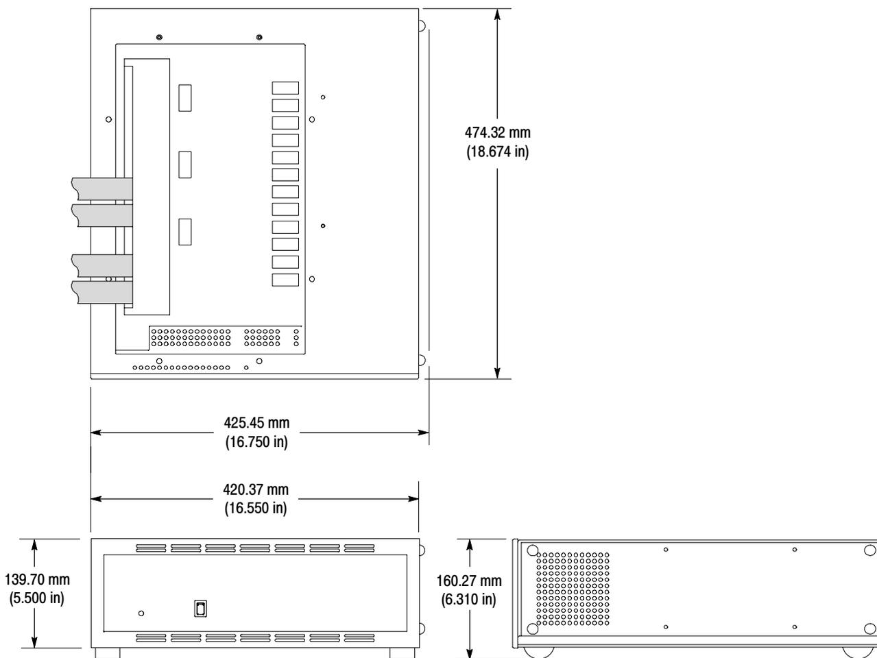
**Figure 4-6: Dimensions of the preprocessor unit**
