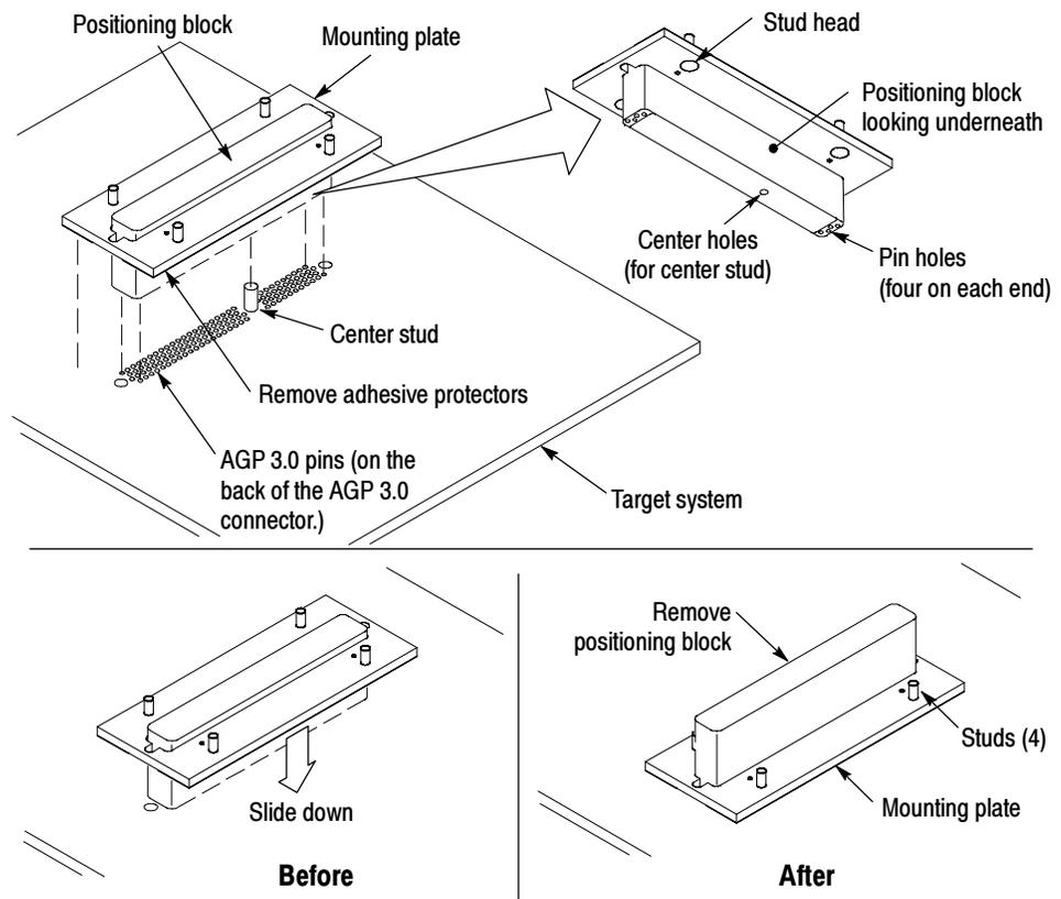
**Figure 1-6: Attaching the mounting plate to the target system**
