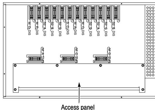
**Figure 1-14: Preprocessor unit and access panel**
