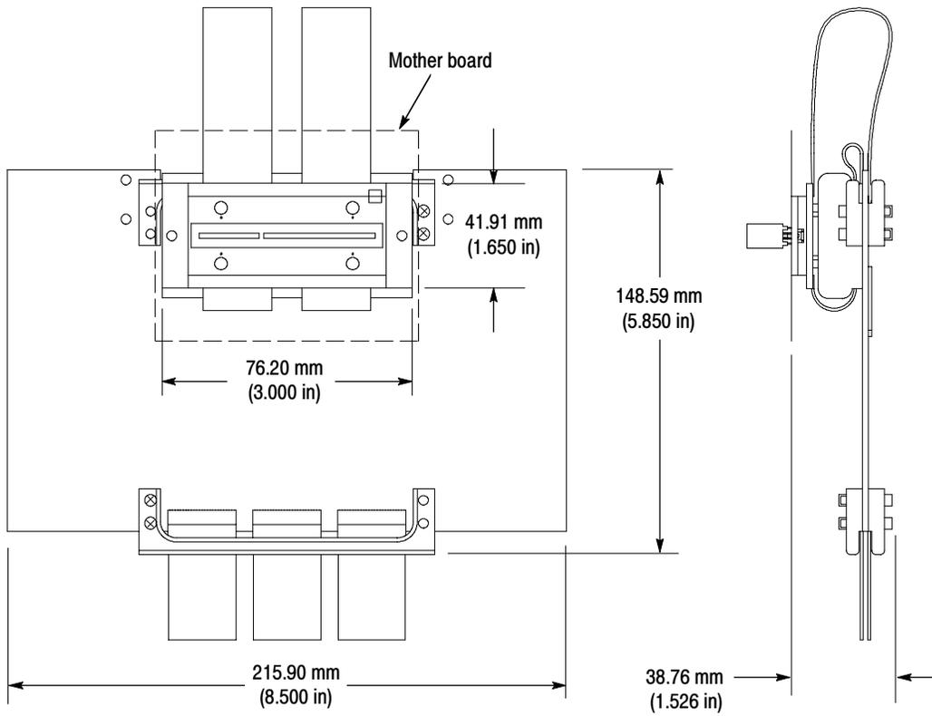
**Figure 4-5: Dimensions of the AGP 3.0 Backside probe head**
