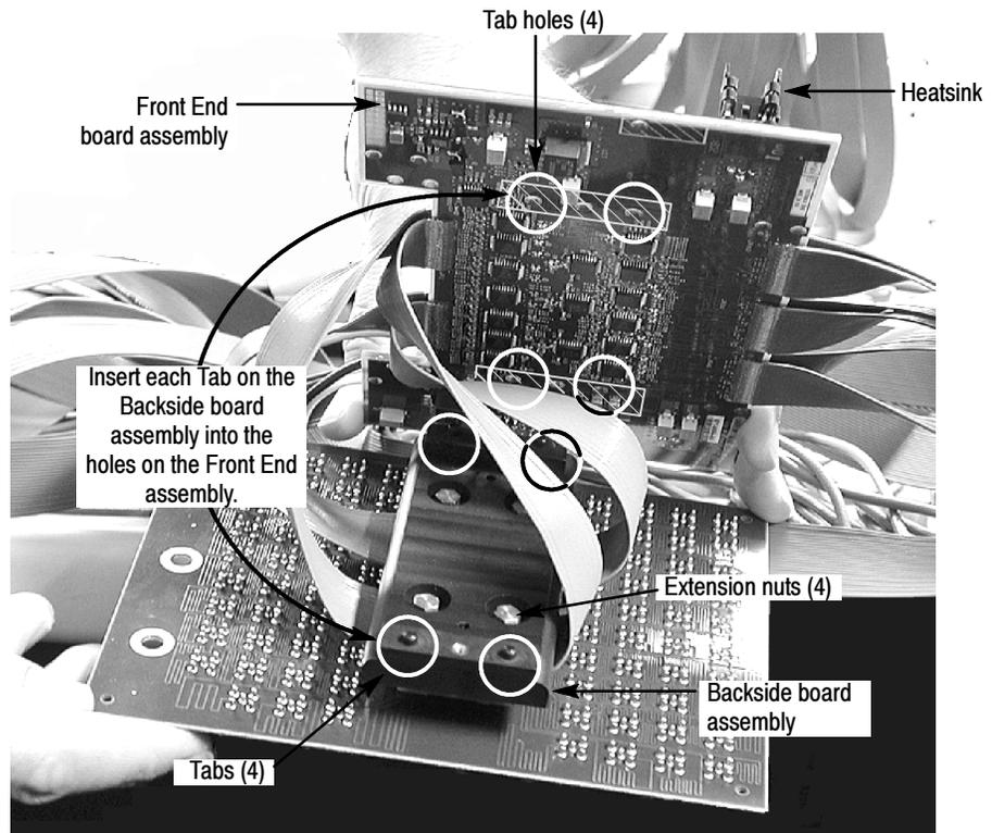
**Figure 1-7: Attaching the Front End board assembly**
