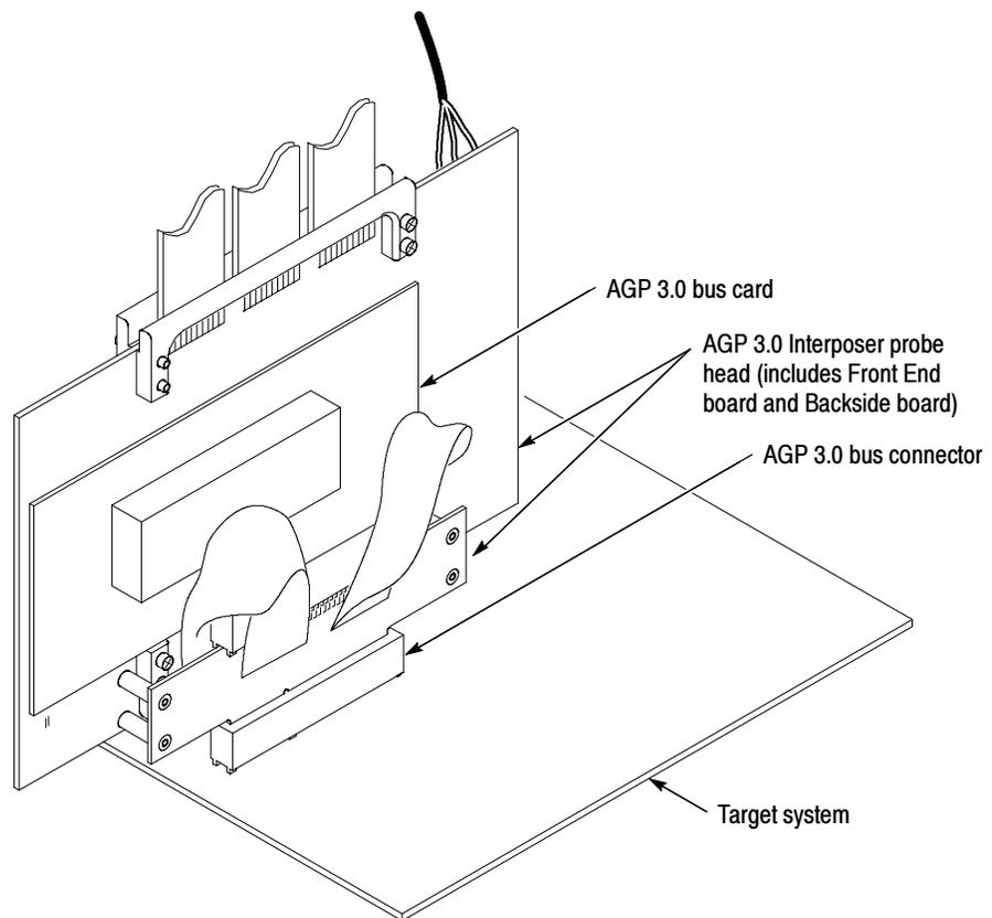
**Figure 1-3: Connect the Interposer probe adapter to the AGP 3.0 bus connector**
