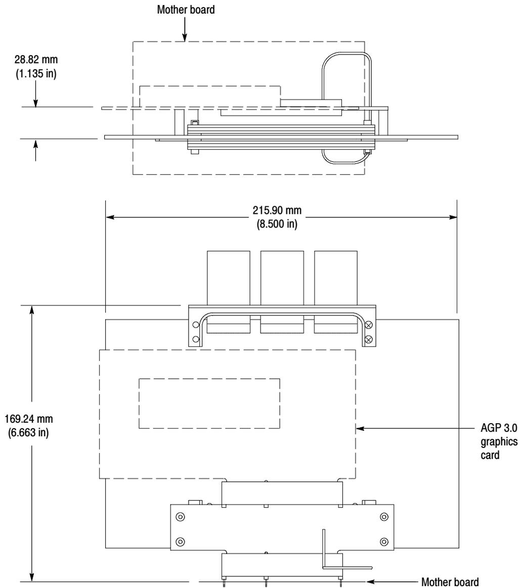
**Figure 4-4: Dimensions of the AGP 3.0 Interposer probe head**
