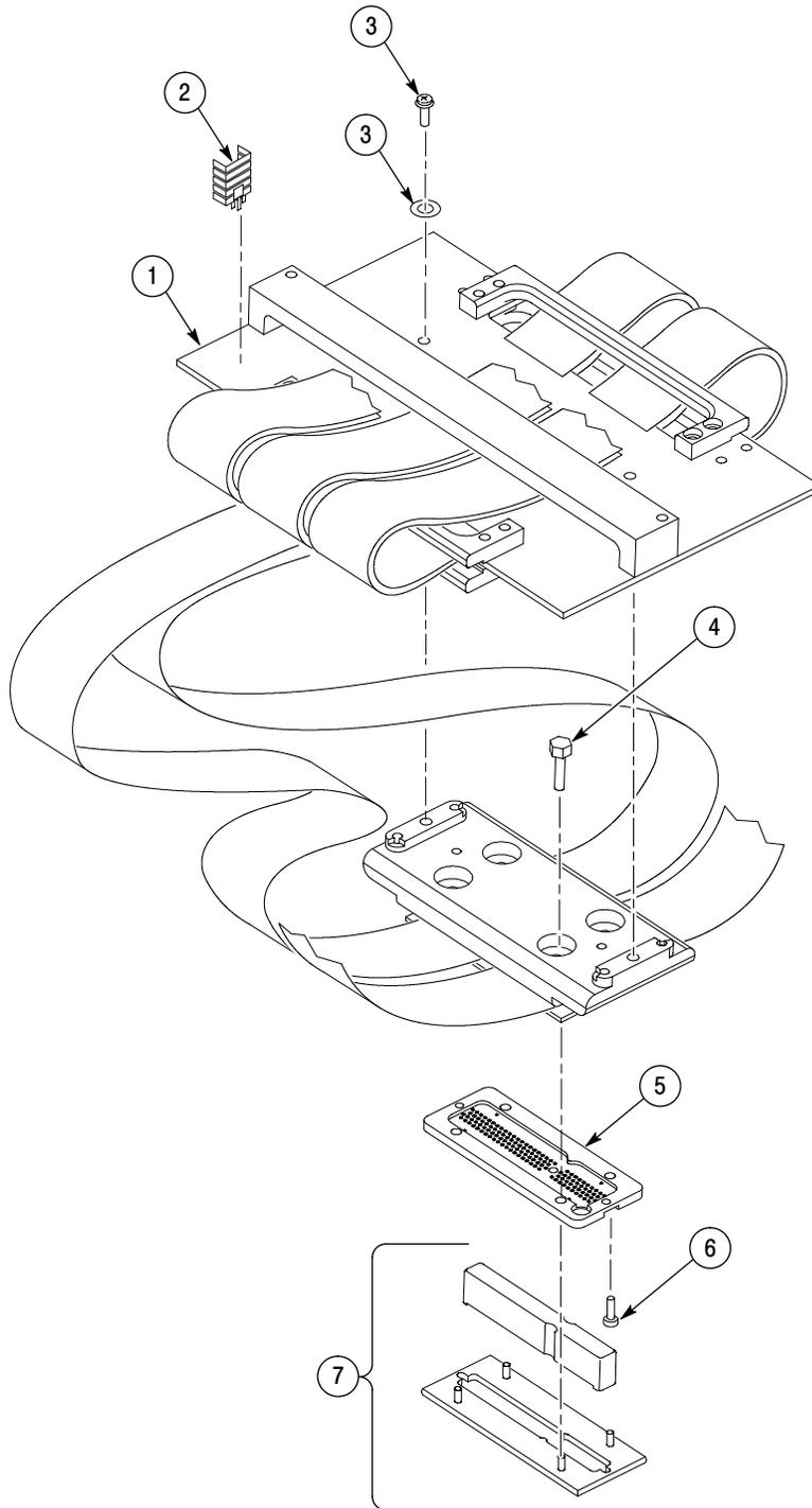
**Figure 6-2: Backside probe head exploded view**
