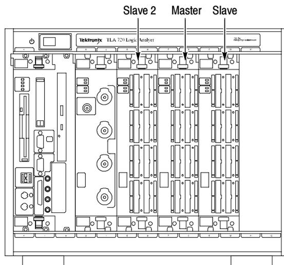
**Figure 1-11: Configuration of the slave 2, master, and slave modules**
