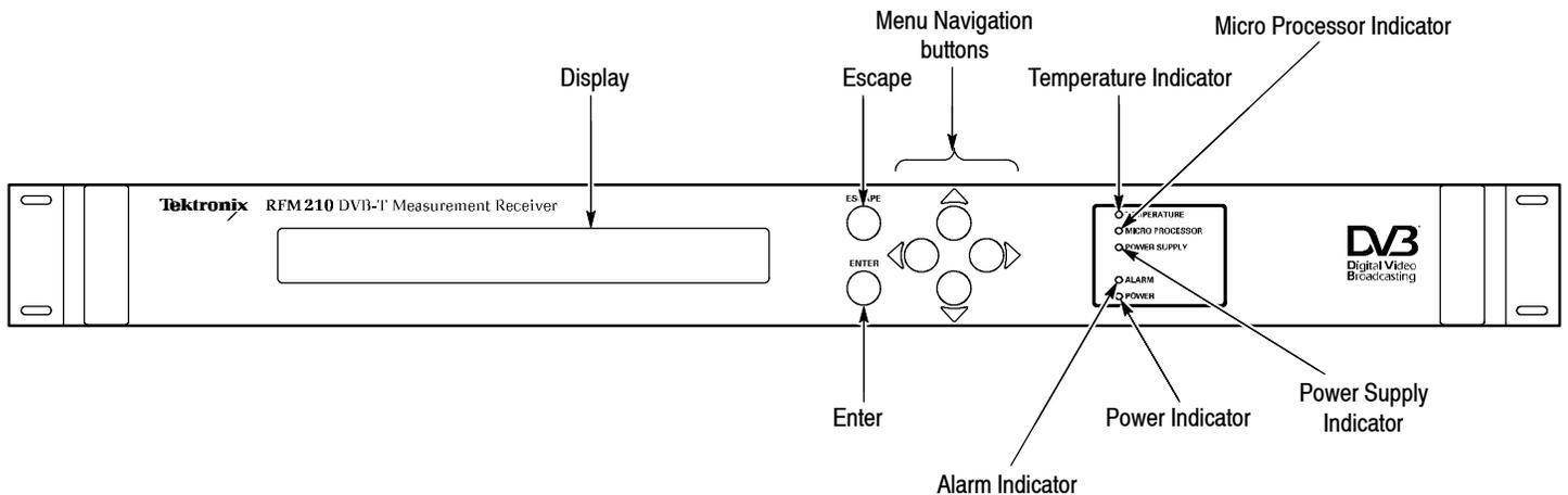
Figure 1-1: RFM210 DVB-T Measurement Receiver front panel display, controls and indicators
