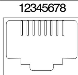
**Figure C-1: Ethernet Port Pin Numbering**
