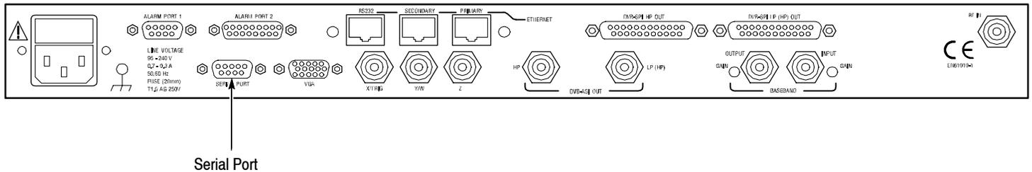
**Figure B-1: Location of RS232 serial port on rear panel**
