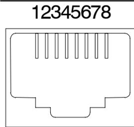
**Figure C-2: Test Port Pin Numbering**
