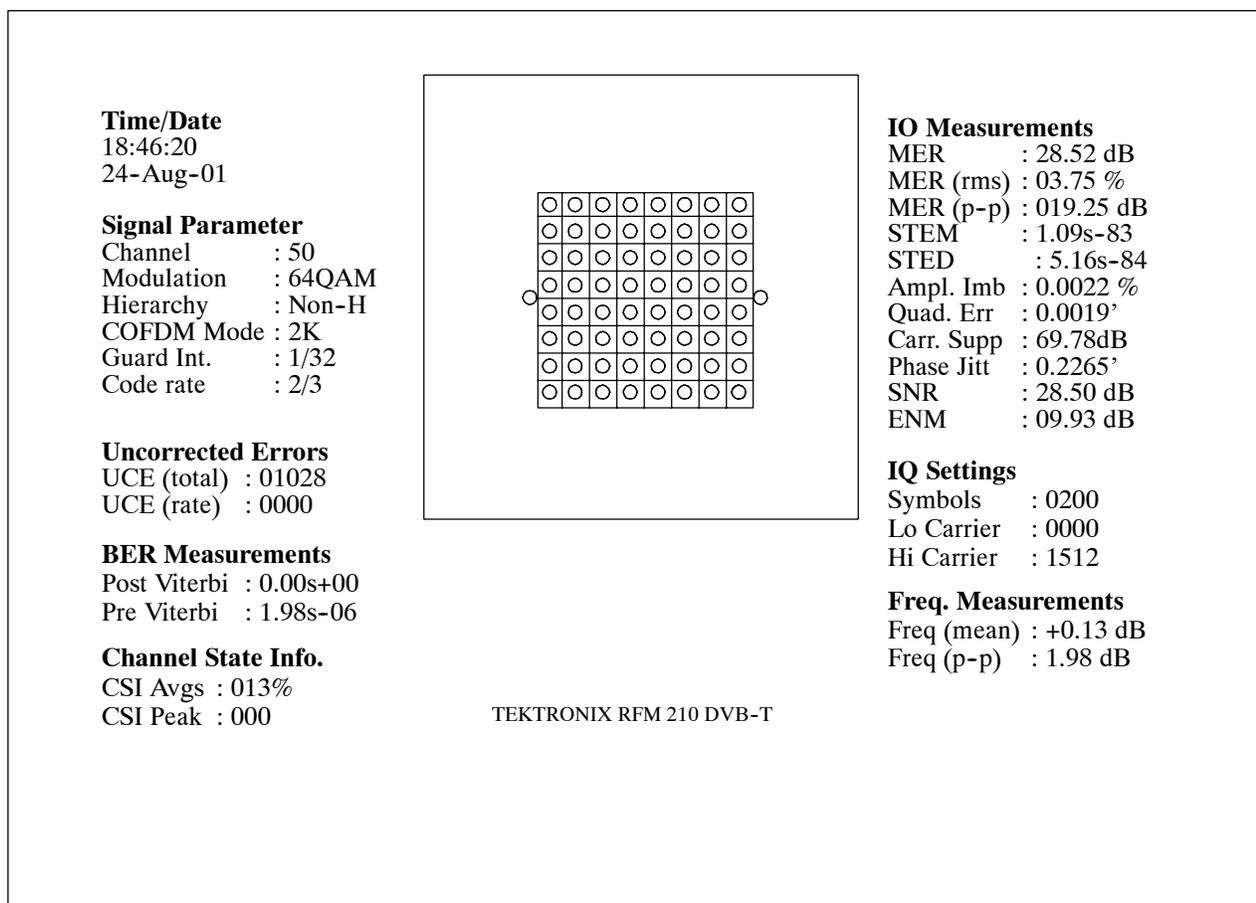
Figure 5-1: Example of output to VGA monitor
