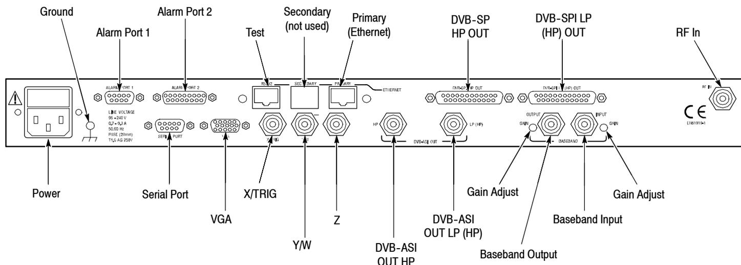
**Figure 1-2: RFM210 DVB-T Measurement Receiver rear panel connectors**
