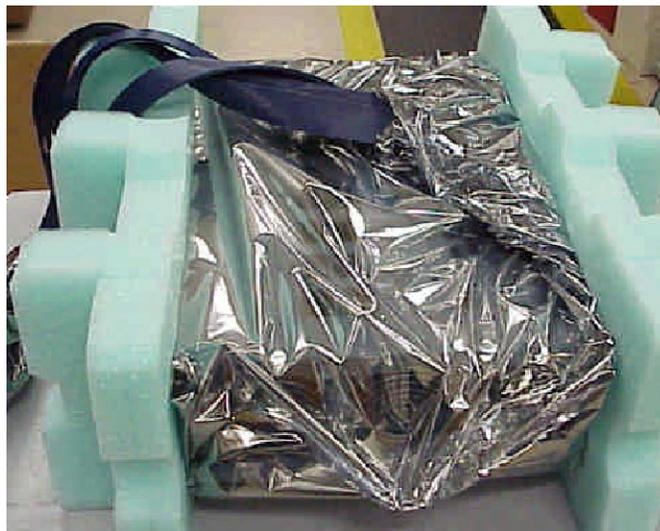
**Figure 1-13: Place the end caps on the preprocessor**
