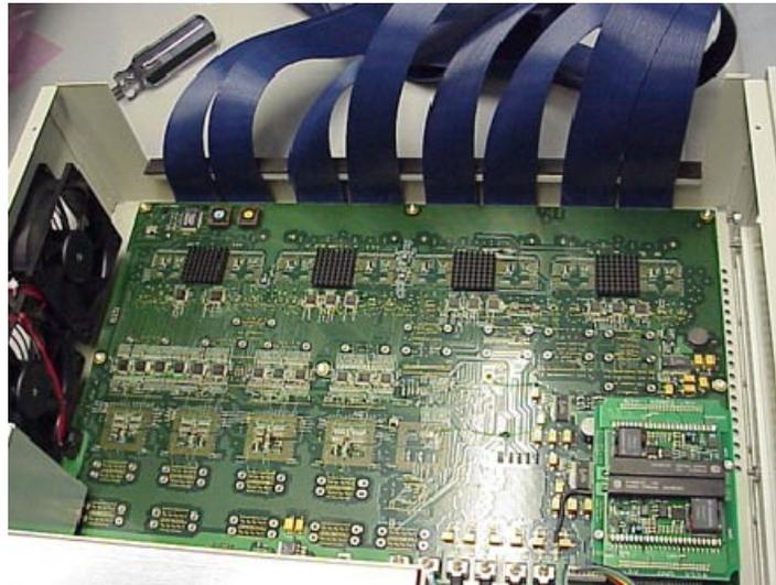
**Figure 5-13: Place logic board in the chassis**
