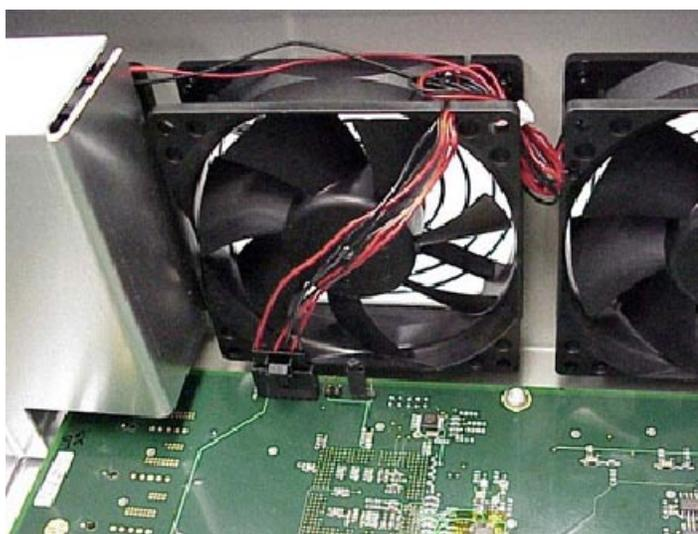
**Figure 5-16: Attach fan plug**
