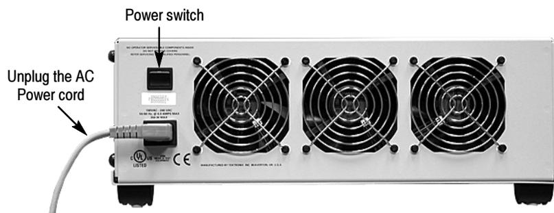
**Figure 5-21: Power switch and AC power cord locations**
