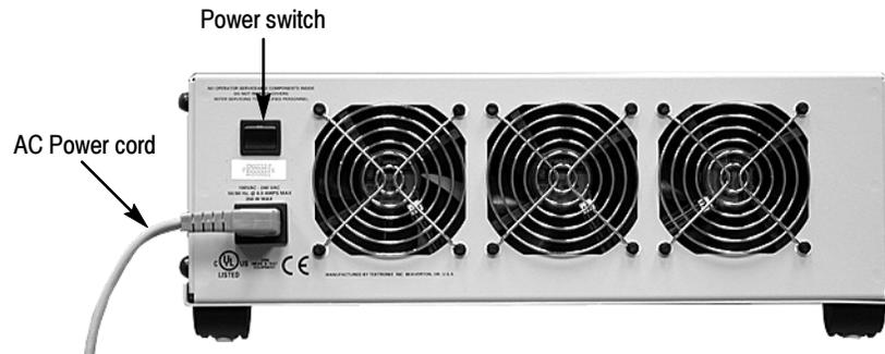
**Figure 5-1: Remove AC power cord**
