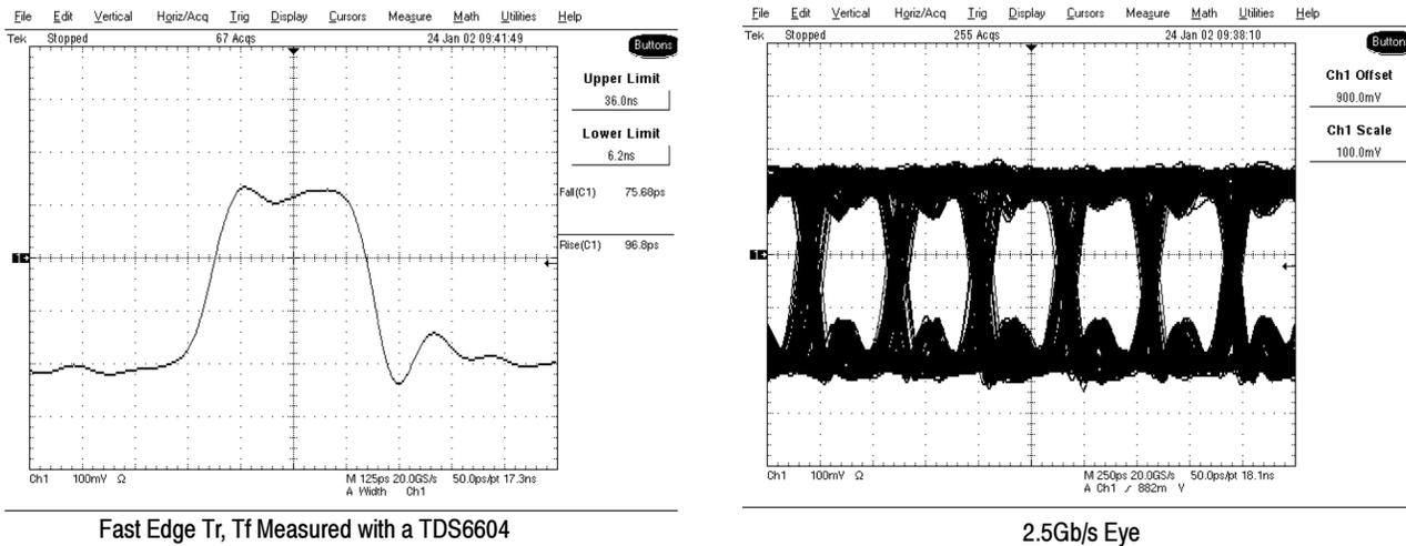
Figure 4: Fast edge and eye diagram
