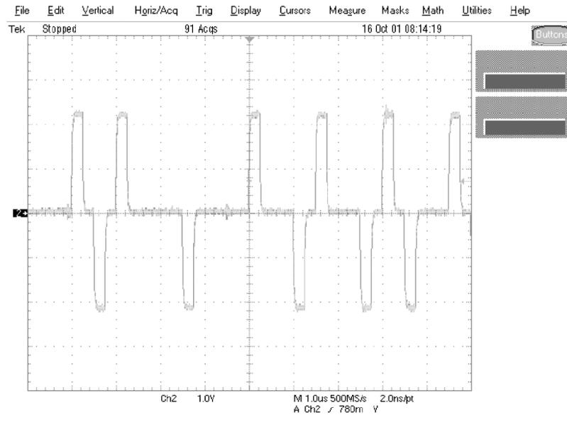
Figure 12: AMI signal at TP3
