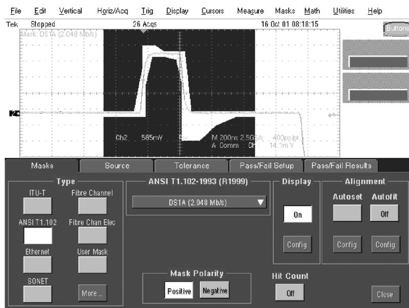
Figure 13: AMI signal in the ANSI T1.102 Mask
