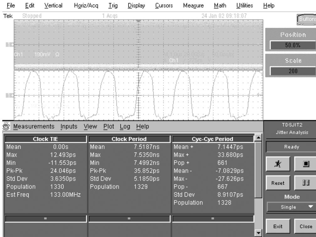
**Figure 6: Jitter analysis demonstrations**
