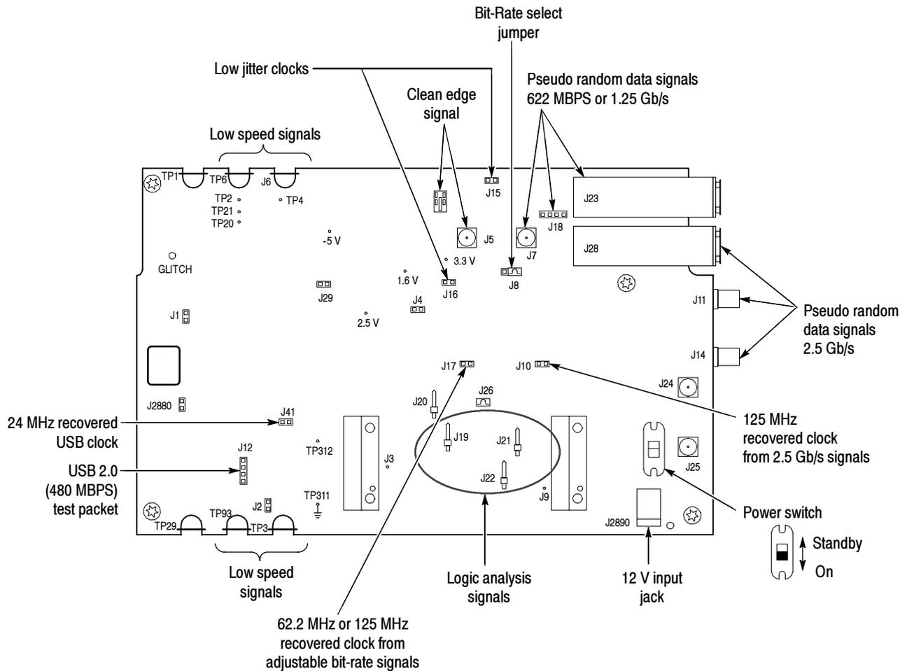
Figure 3: Training Board 2 signal and test points
