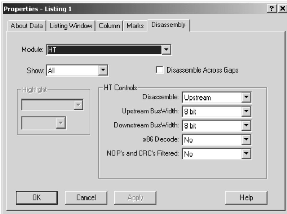
**Figure 2-1: Disassembly display options for HT support package**
