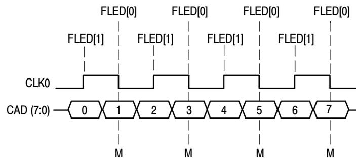
**Figure 3-4: Timing diagram for Upstream or Downstream bus.**
