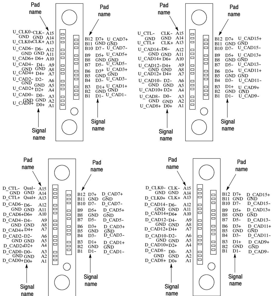
**Figure 3-2: P6880 differential probe land footprint for HT\_Tek and HT\_Tek\_Cal support packages**
