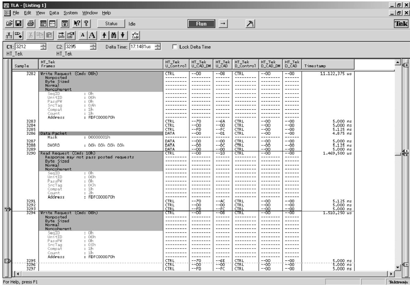
Figure 2-3: Example of All Display format with CRC and NOP packets filtered for the HT\_Tek support package
