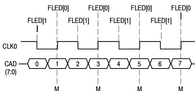
**Figure 3-5: Timing diagram for Upstream and Downstream bus with Clock Inverted.**
