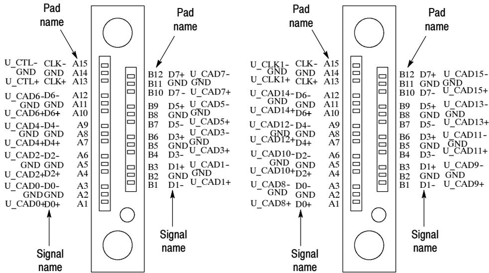
**Figure 3- 1: P6880 differential probe land footprint for HT and HT\_Cal support packages**
