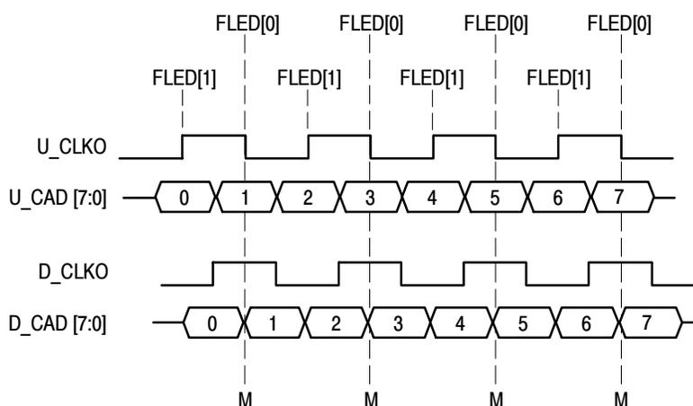
**Figure 3-7: Timing diagram for Upstream and Downstream bus with skew**
