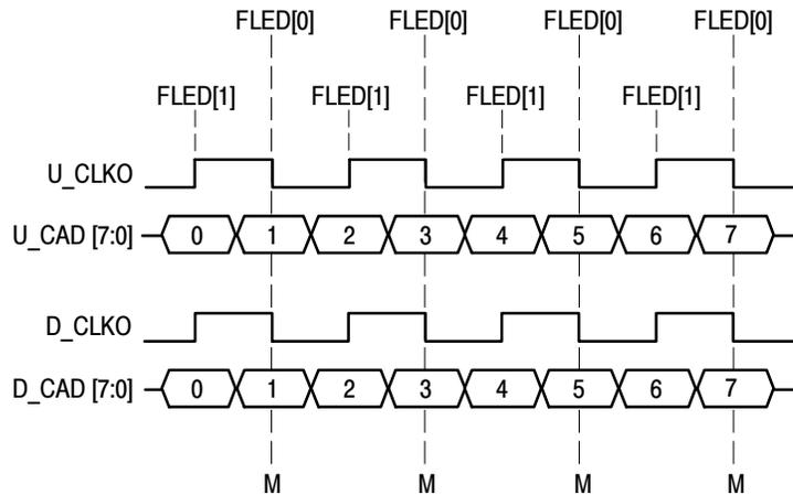
**Figure 3-6: Timing diagram for Upstream and Downstream bus**
