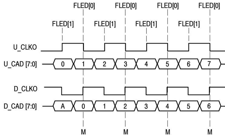
**Figure 3-8: Timing diagram for Upstream and Downstream with 180 degree phase shift**
