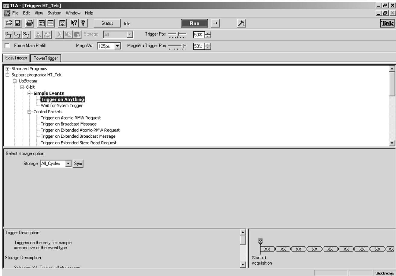
**Figure 2-5: Loading trigger programs**
