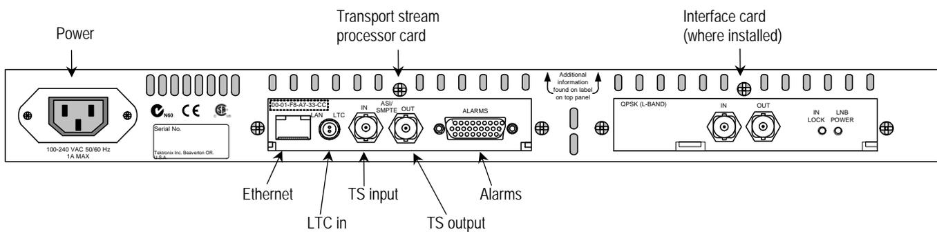
**Figure 1-1: MTM400 connectors (shown with QPSK interface)**
