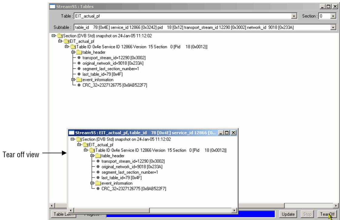
**Figure 3-27: SI Tables view - Tear off view**
