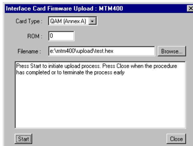
2. Select the **Card Type** to which the firmware is to be uploaded from the drop-down list.
