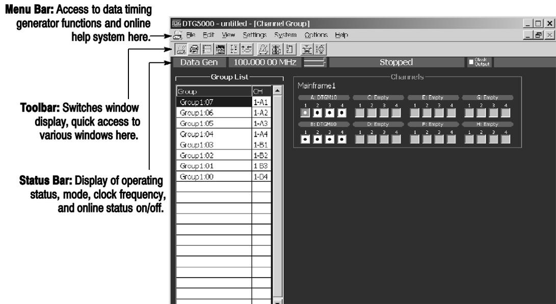
Figure 2-4: Screen elements just after the power on
