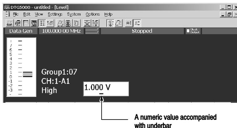
**Using the External Keyboard.** Numeric keys above the alphabetical letter keys, not those on the numeric keypad, are available on the external keyboard. The k (kilo-), M (mega-), G (giga-), m (milli-),  $\mu$  (micro-), n (nano-) and p (pico-) keys are available for auxiliary units.
