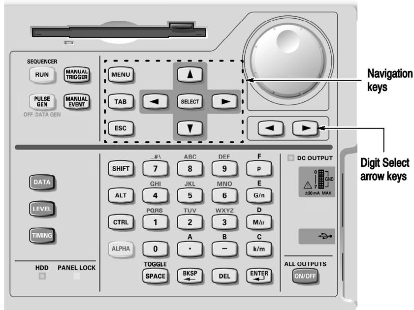
**Figure 2-1: Front panel controls**
