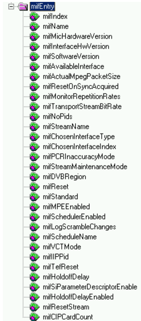
Figure 5-3: MPEG interfaces table structure
