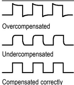
4. If necessary, adjust your probe. The P2220 probe is shown. Repeat as necessary.
