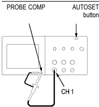
1. Push the **CH 1 MENU ▶ Probe ▶ Voltage ▶ Attenuation** option and select **10X**. Set the switch to 10X on the P2220 probe and connect the probe to channel 1 on the oscilloscope. If you use the probe hook-tip, ensure a proper connection by firmly inserting the tip onto the probe.
