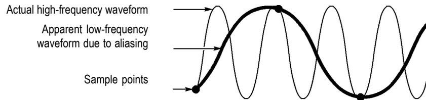
The oscilloscope accurately represents signals, but is limited by the probe bandwidth, the oscilloscope bandwidth, and the sample rate. To avoid aliasing, the oscilloscope must sample the signal more than twice as fast as the highest frequency component of the signal.
