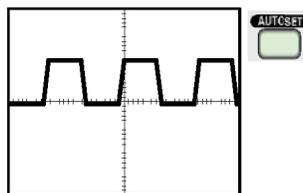
3. Push the **AUTOSET** button. Within a few seconds, you should see a square wave in the display of about 5V peak-to-peak at 1 kHz.
