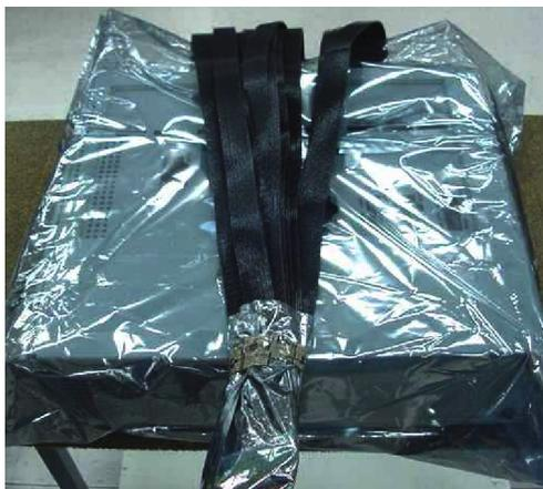
**Figure 12: Preprocessor unit and probe head in static-shielding bags**
