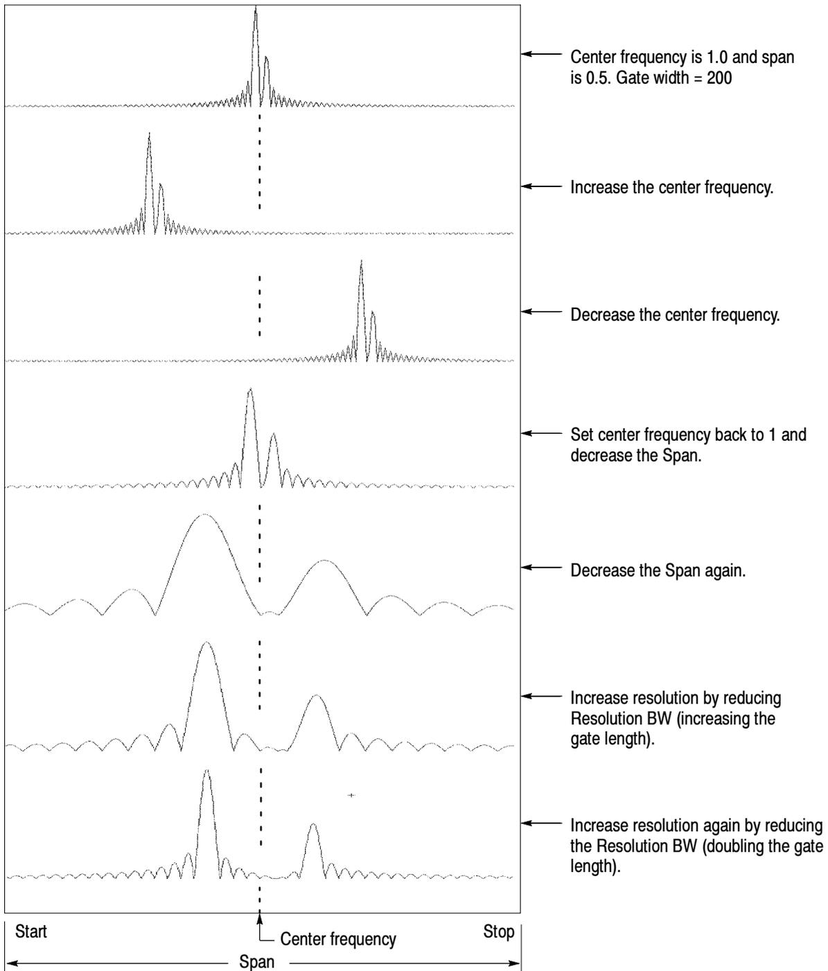
**Figure 3-44: Effects of frequency domain control adjustments**
