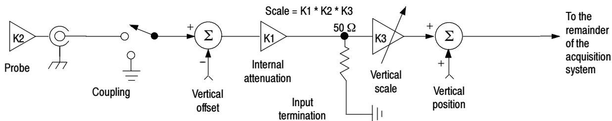
**Figure 3-1: Input and Acquisition Systems and Controls**
