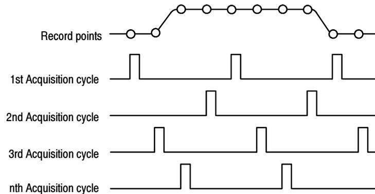
**Figure 3-12: Equivalent-time sampling**
