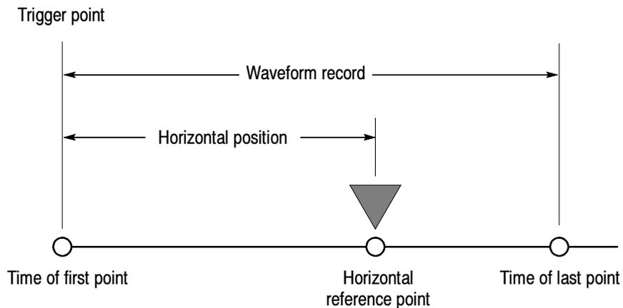
**Figure 3-28: Horizontal Position includes time to Horizontal Reference**
