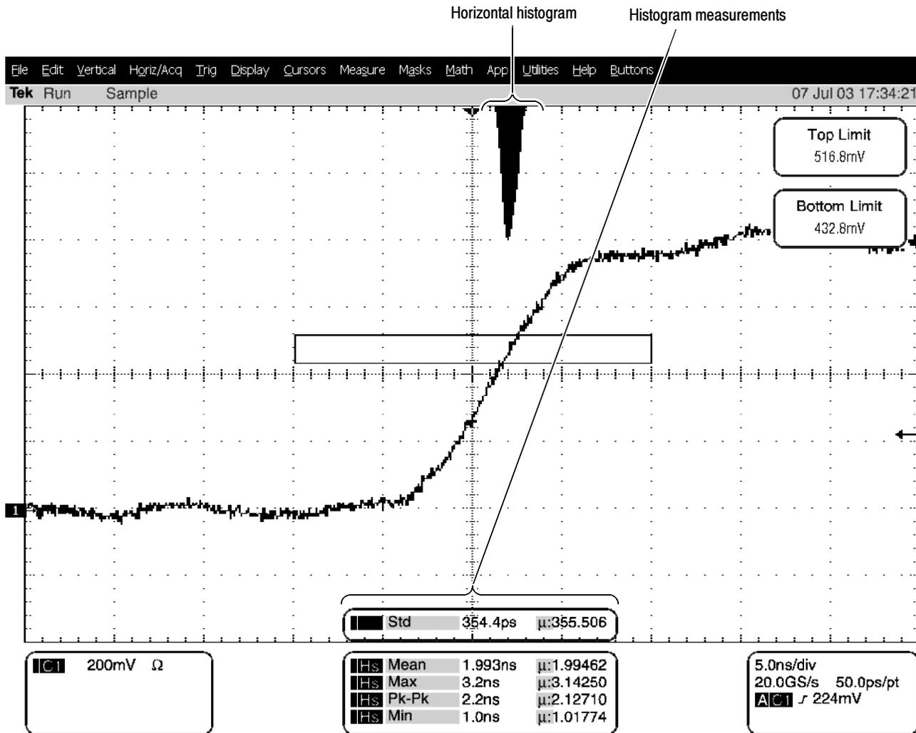
Figure 3-35: Horizontal histogram view and measurement data
