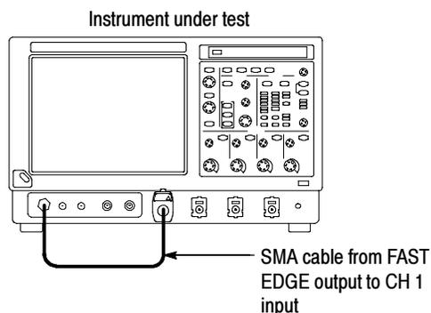
**Figure 1- 11: Setup for time base test**
