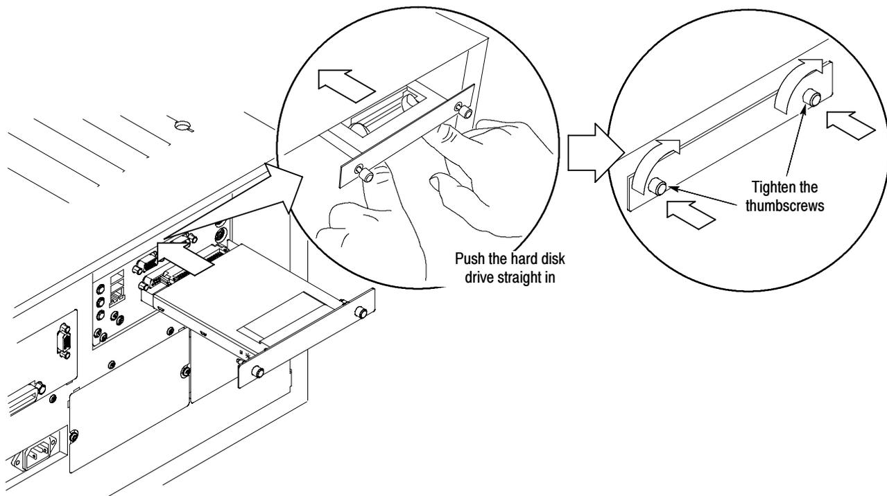
Figure 1-4: Reinstalling the hard drive
