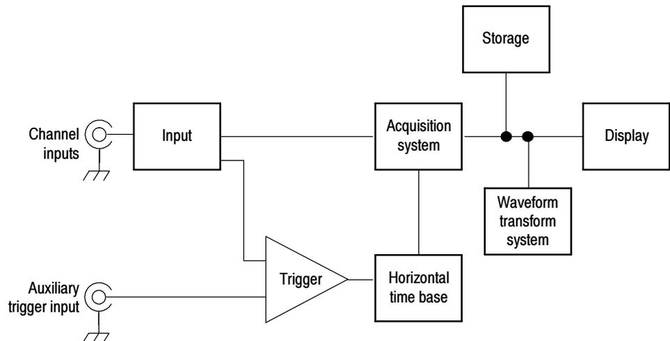
**NOTE.** This section describes how the vertical and horizontal controls define the acquisition of live waveforms. These controls also define how all waveforms are displayed, both live and derived waveforms (math waveforms, reference waveforms, and so on). The sections that follow cover display-related usage:
