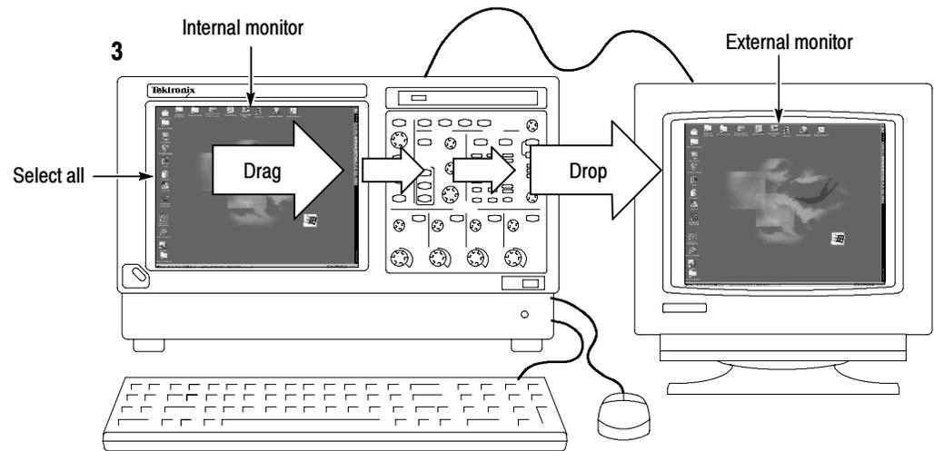
**Figure 1-8: Moving Windows desktop icons to the external monitor**
