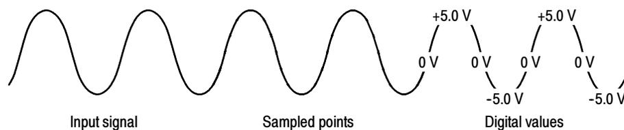
**Figure 3-9: Digital acquisition — sampling and digitizing**
