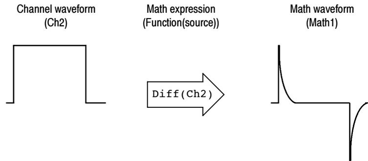
**Figure 3-39: Functional transformation of an acquired waveform**
