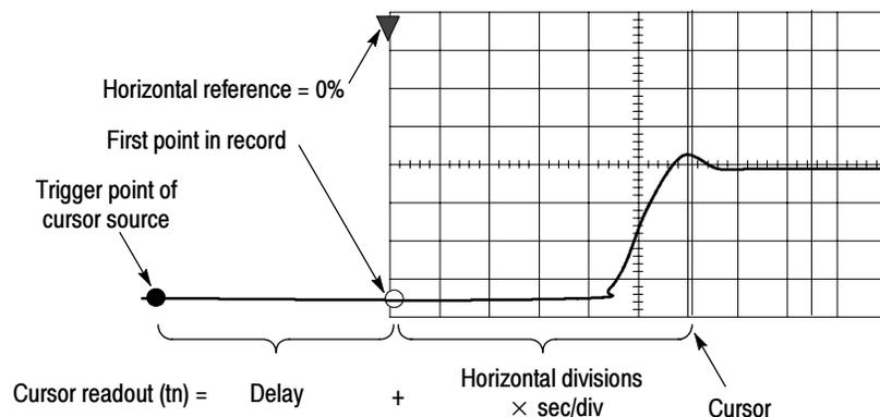
**Figure 3-34: Components determining Time cursor readout values**
