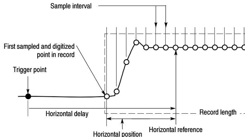
**Figure 3-10: The waveform record and its defining parameters**
