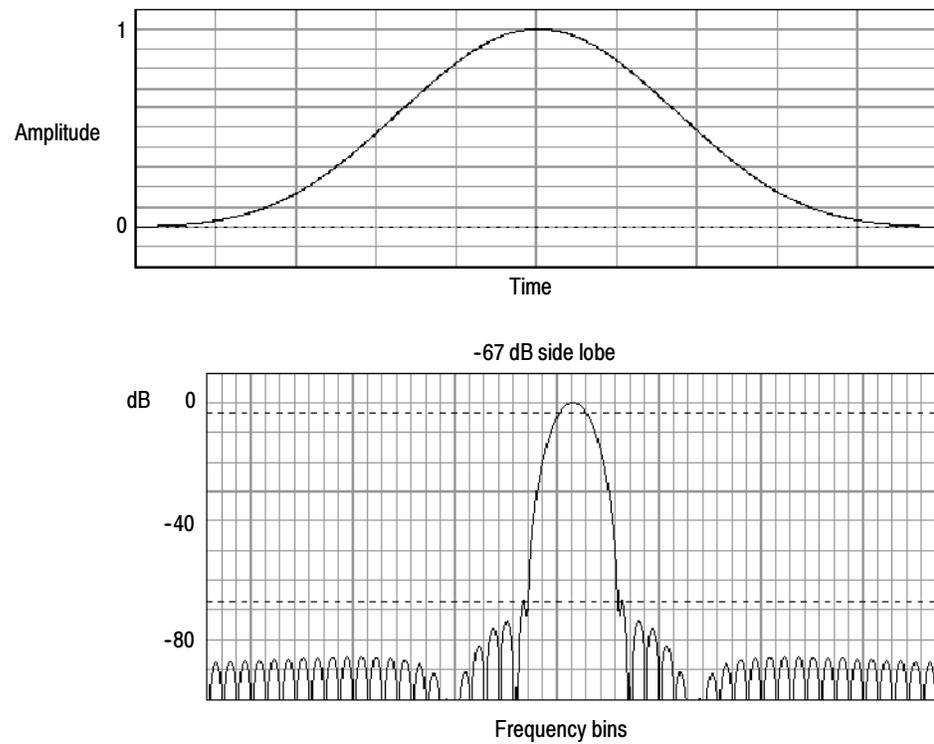
**Figure 3- 54: Time and frequency graphs for the Kaiser-Bessel window**
