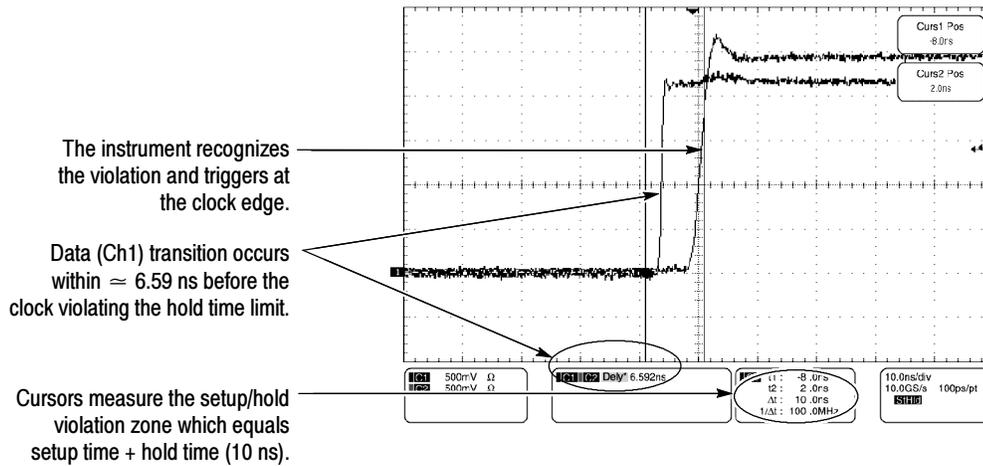
**Figure 3-22: Triggering on a Setup/Hold time violation**
