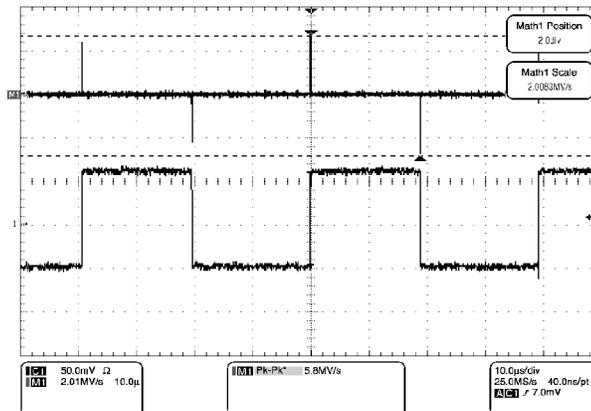
**Figure 3-41: Peak-peak amplitude measurement of a derivative waveform**
