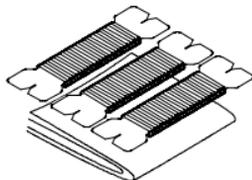
The P7313 HBW Tip-Clip™ Assemblies consist of a colored plastic clip, a flex circuit, and two resistors. Each resistor has one 8 mil diameter wire attached. In addition, there are two elastomeric buttons between the flex and this clip. These are required to ensure reliable contact between the flex and the probe head. Do not remove the flex from the clip, as you may lose the elastomers.
