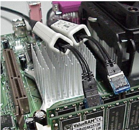
**Figure 20: Circuit board with Tip-Clip assemblies**
