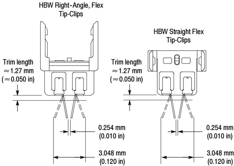
**Figure 13: Wire-lead length for HBW Tip-Clip assemblies**
