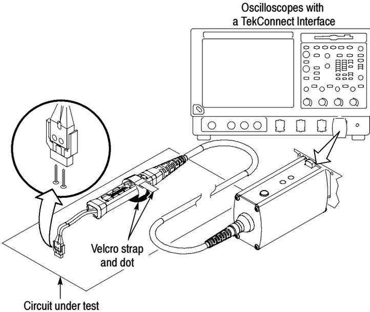
**Figure 17: Square Pin Tip-Clip assembly**
