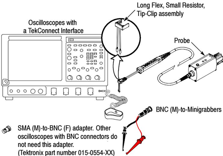
**Figure 3: Equipment used for the functional check**
