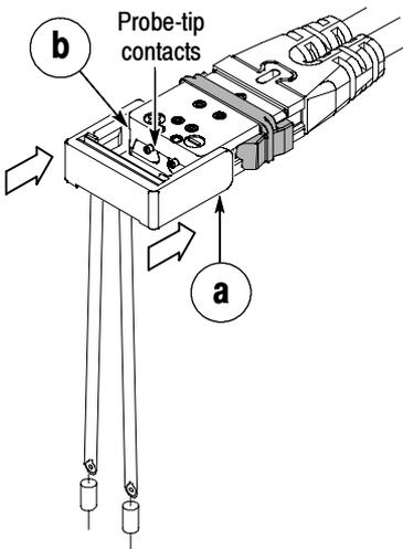
**Figure 5: Installing a Tip-Clip assembly**
