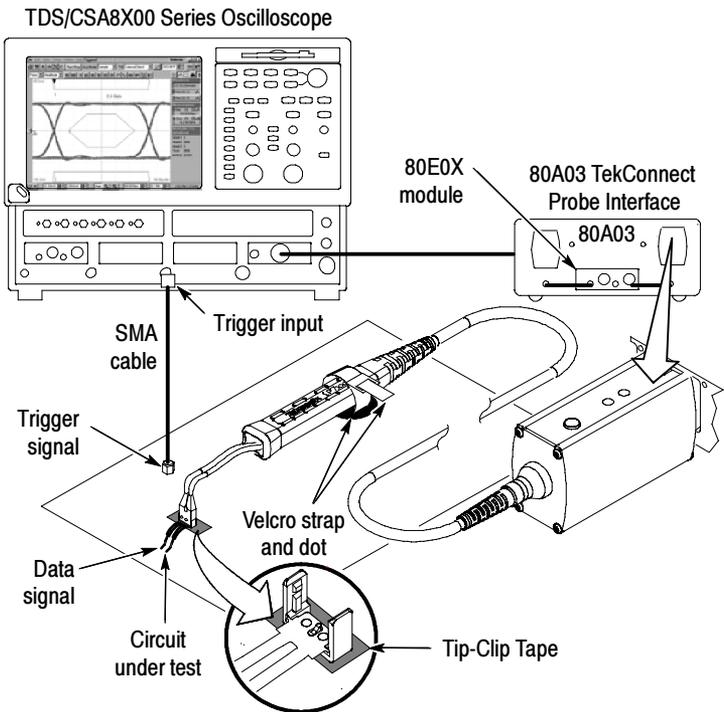
**Figure 12: TDS/CSA8X00 Series Sampling oscilloscope**
