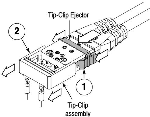
**Figure 8: Removing a Tip-Clip assembly**
