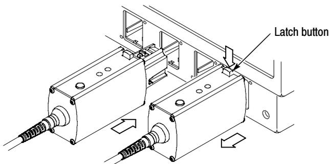
**Figure 1: Connect TekConnect to instrument**
