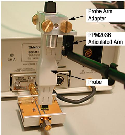
**Figure 18: Fixtured probe**
