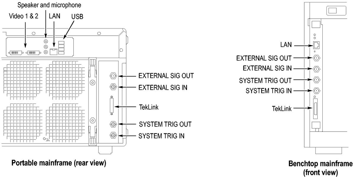
Figure 58: TLA7000 Series external connectors
