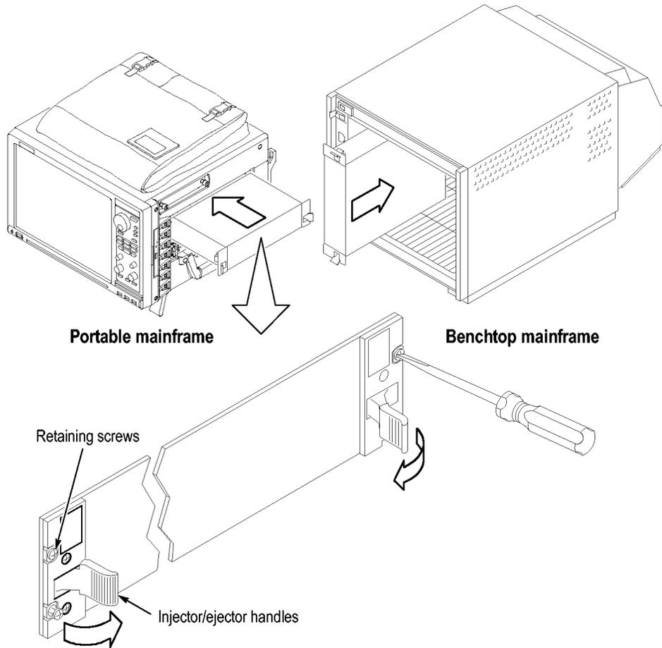
**Figure 39: Installing modules**
