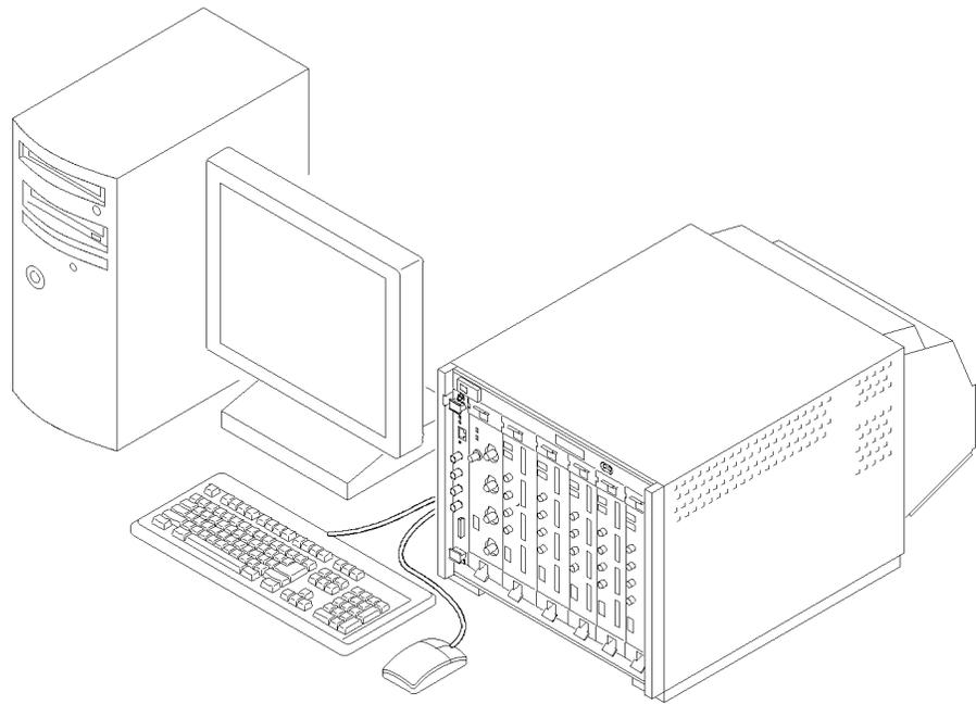
**Figure ii: TLA7016 Benchtop Mainframe (with user-supplied PC controller)**
