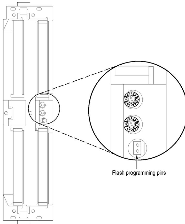
**Figure 59: Flash programming pins**
