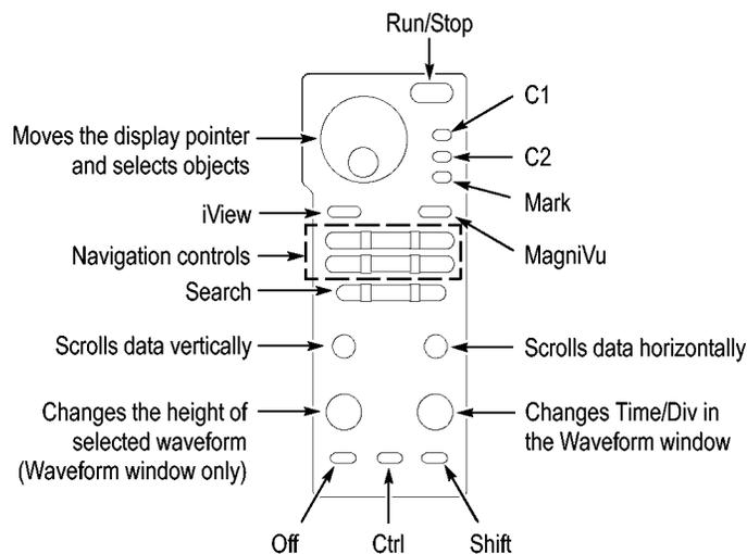
Figure 57: Portable mainframe front panel
