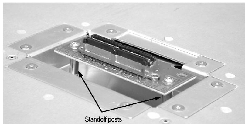
**Figure 49: Removing the merger connector assembly from the module**
