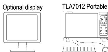
**Figure 6: Portable mainframe setup (up to two modules)**
