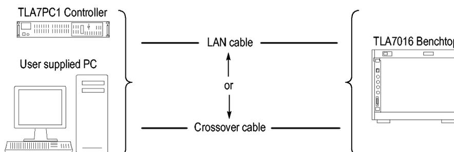
**Figure 7: Benchtop mainframe setup (up to six modules)**
