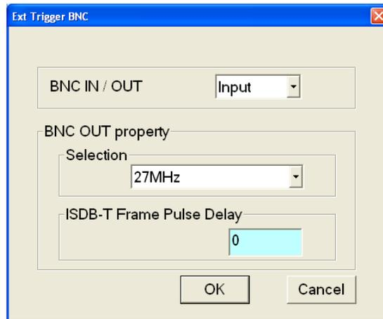
**BNC IN/OUT:** Sets whether to use the rear-panel Trig In/Out connector as a trigger signal input or a reference/ISDB-T frame pulse signal output. You can select INPUT or OUTPUT. For INPUT, the Trig In/Out connector can be used to input an external trigger event. For OUTPUT, the Trig In/Out connector can be used to output a 27 MHz reference clock or an ISDB-T frame pulse signal. Use the Selection list box to select which signal is output from the connector.
