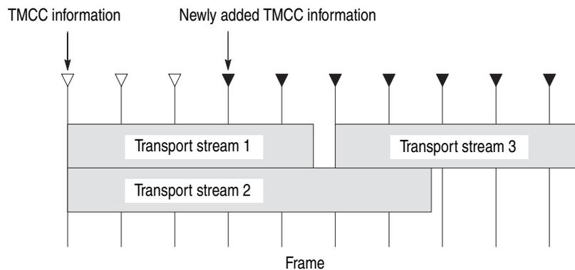
This illustration shows the positional relationship when inserted TMCC information and the transport stream 3 after the transport stream 1 while two transport streams have been multiplexed. The new TMCC information is inserted two frames before the location in which the new transport stream is inserted.
