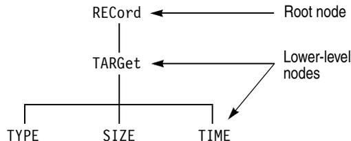
**Figure 3-29: Example of SCPI subsystem hierarchy tree**
