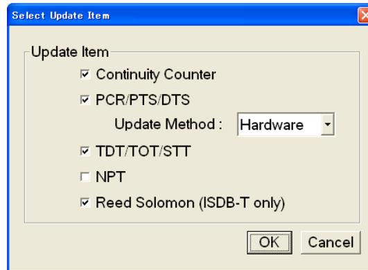
**Continuity Counter:** Sets whether to update continuity\_counter. Press the TAB button repeatedly to select this item, and then press the SELECT button to toggle the check box on or off.
