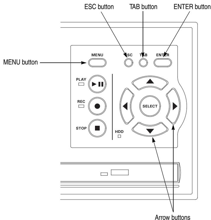
**Figure 2-7: Front panel showing the menu controls**
