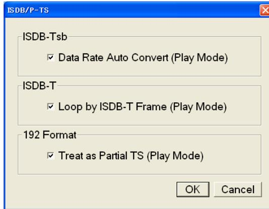
**Data Rate Auto Convert (Play Mode):** Sets whether to set the clock rate automatically when the ISDB-TSB file is loaded. Press the TAB button repeatedly to select this item, and then press the SELECT button to toggle the check box on (checked) or off (not checked). When it is checked, the clock rate is automatically set to  $(2048/1701) \times 27$  MHz and the elementary stream rate becomes constant regardless of the Fixed ES Rate setting.
